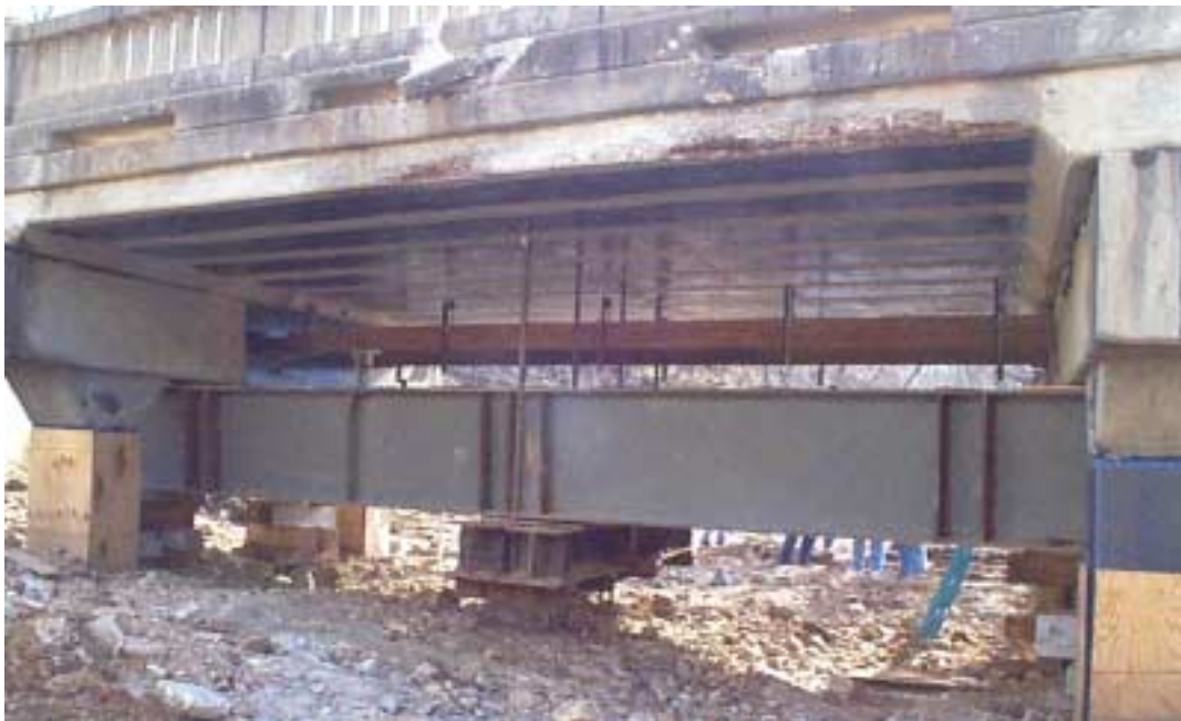
Figure 4.14. Assembled test setup for the middle deck (deck 2).
