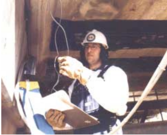
Figure 4.23. Checking the strain gages prior to testing.
