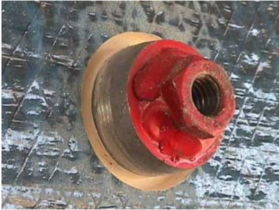
Figure 3.13. Adhesion fixture bonded to the FRP sheet.
