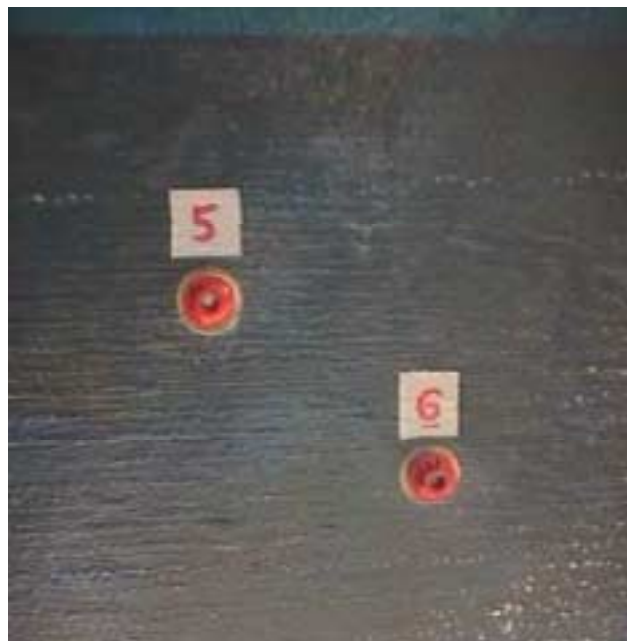
Figure 3.12. Locations of the pull-off tests conducted on bridge deck.
