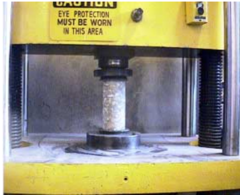
(a) Uniaxial compression test setup
