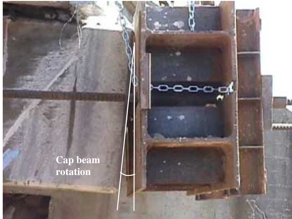
Figure 4.17. Cap beam rotation
