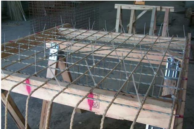
**Figure 2.** Rig for GFRP cage assembly
