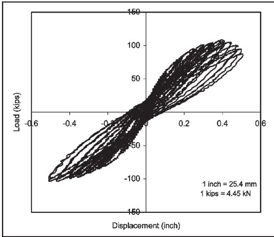
Figure 6 – Hysteretic Loops of Retrofitted Wall Sample W<sub>4</sub>-C-RT.
