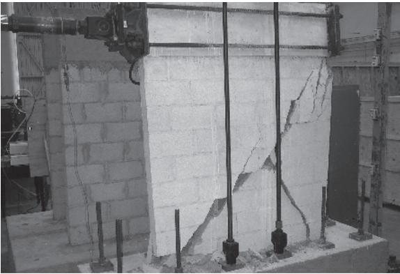
Figure 3 — Shear Failure of the As-built Wall Sample.
