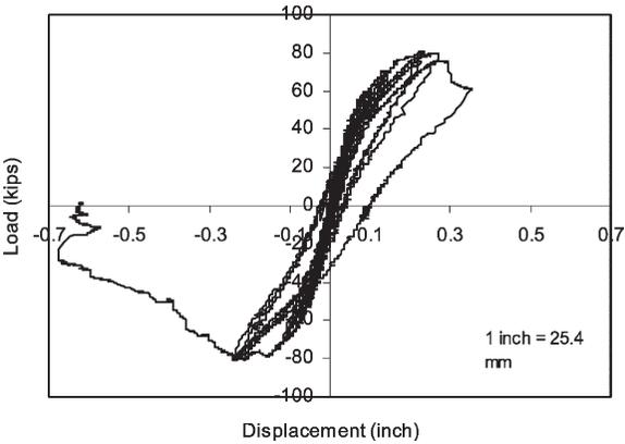
Figure 4 — Hysteretic Loops of the As-built Wall Sample.
