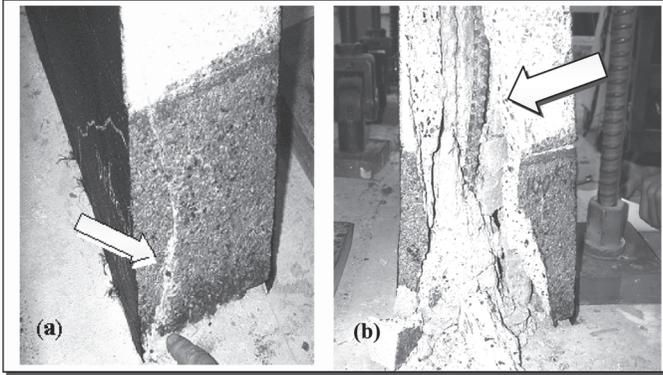
Figure 5 — Premature Compression Failure of Masonry Units at Wall Toes
