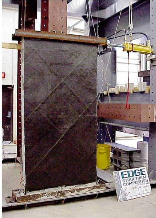
**Figure 5.** Retrofitted Shear Specimen at Failure
