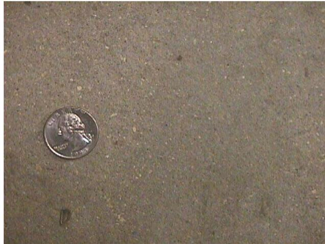
**Figure 3.5: Sandblasted Concrete Surface**
