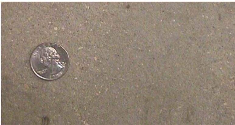
**Figure 5.16: Sandblasted Surface**
