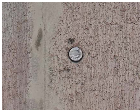
Figure 4.7 Pressure Transducer Placed at the Front Face of Wall
