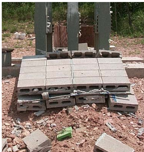
Figure 6.9 Front Face of C1 after Event #6 Figure 6.10 Collapse of C1 after Event #7
