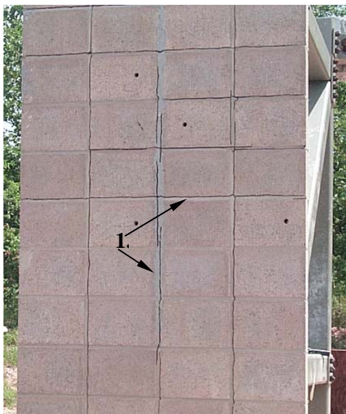
Figure 6.9 Front Face of C1 after Event #6 Figure 6.10 Collapse of C1 after Event #7
