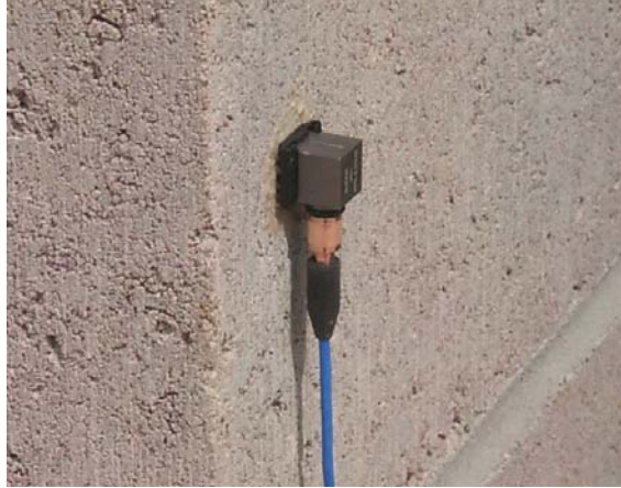
Figure 4.8 Accelerometer Placed to Back Face of Wall
