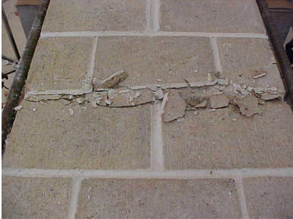
**Fig A.15 Flexural Failure: Crushing of the Masonry (S12-CO0)**
