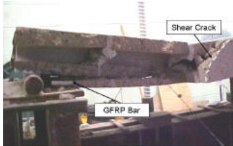
Figure – 6. Shear Failure (Wall B3)
