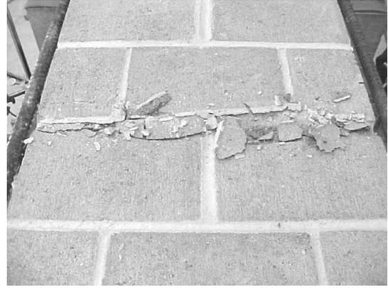
(b) Crushing of Units at Midspan (CO0)
