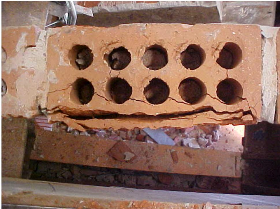
**Fig A.16 Crushing of the Masonry at the Supports (S12-CL0)**
