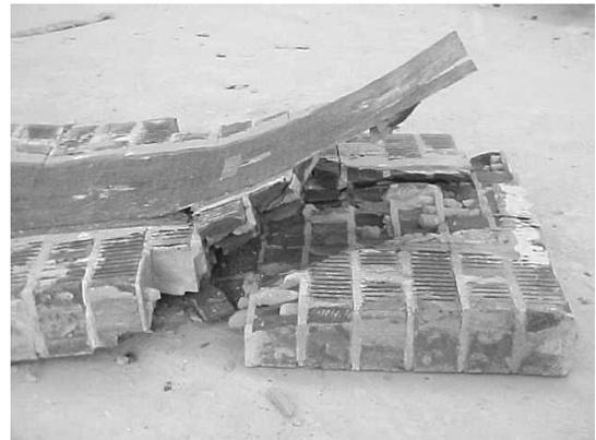
(f) Shear Failure (CL9)
