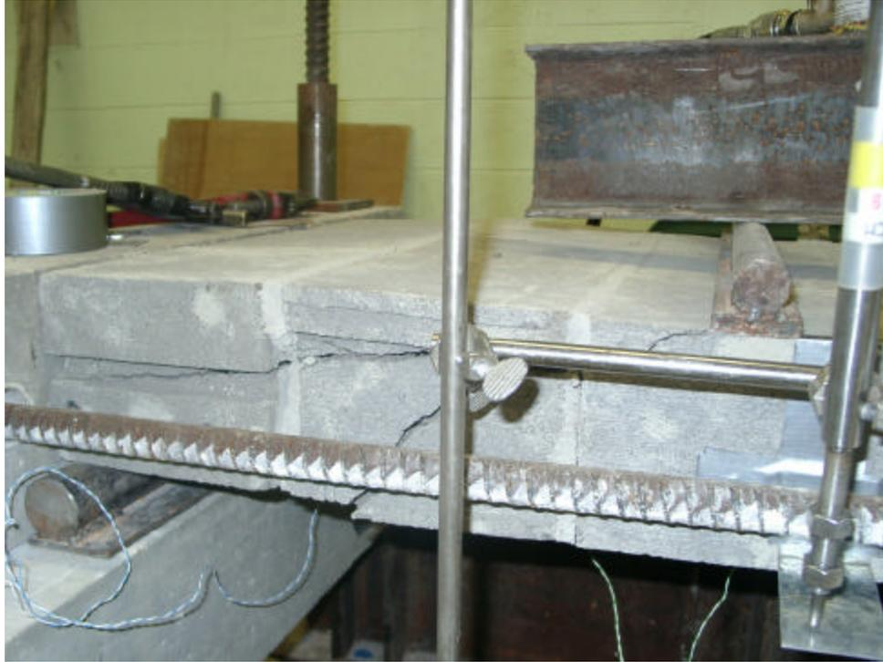
**Fig A.17 Splitting of the Masonry at the Supports (S8-CO5)**
