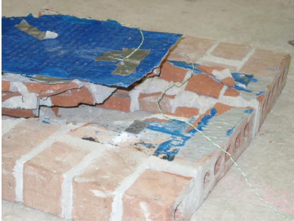
**Fig A.19 Shear Failure (S12-CL7)**
