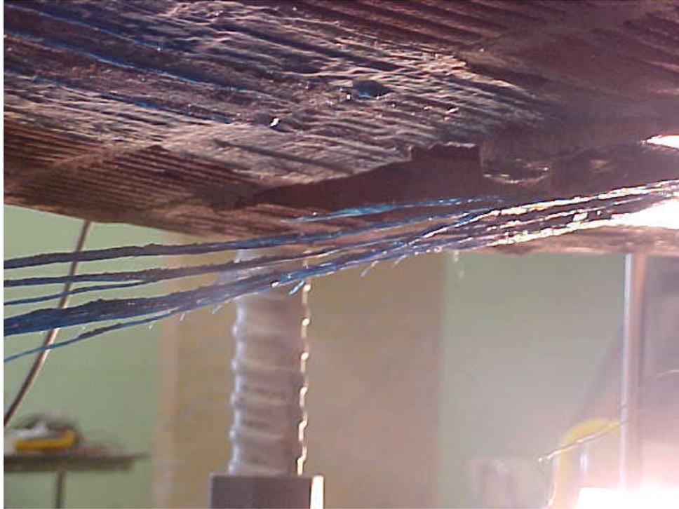
**Fig A.13 Flexural Failure: FRP Rupture (S12-CL3)**
