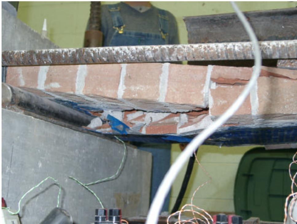
**Fig A.18 Shear Failure (S19-CL7)**
