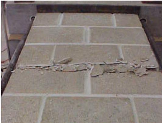
(c) Crushing of Units at Midspan (S12-CO0)
