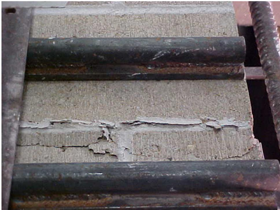
**Fig A.14 Flexural Failure: Crushing of the Masonry (S12-CO0)**
