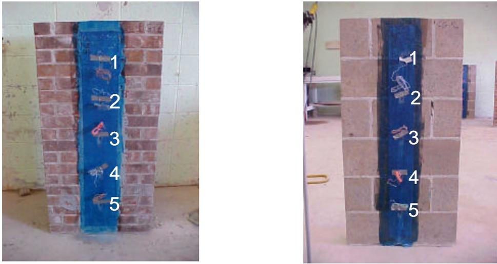
**Figure 3. Test Specimens And Strain Gage Locations**
