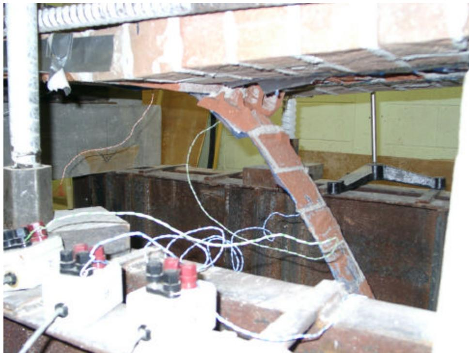
**Fig A.12 Flexural Failure : FRP Debonding (S19-CL5)**
