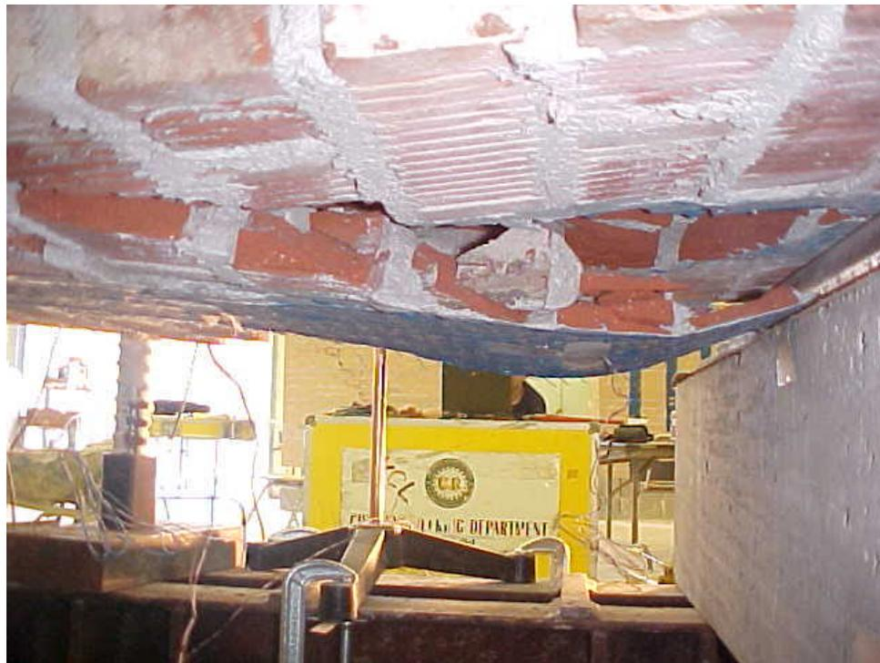
**Fig A.10 Flexural Failure: FRP Debonding (S12-CL5)**
