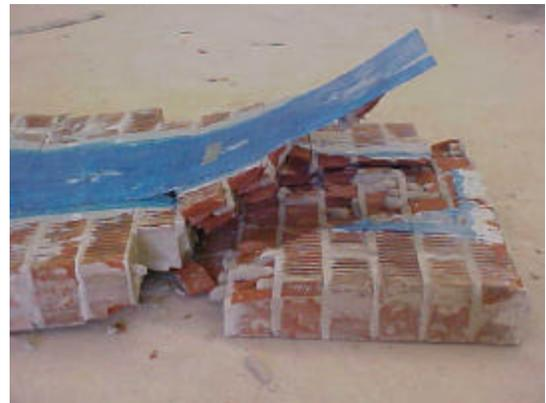
(f) Shear Failure (S12-CL9)
