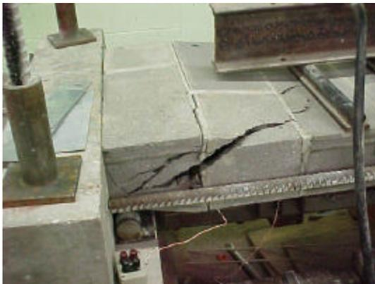
(e) Splitting of the Masonry Units (S8-CO3)
