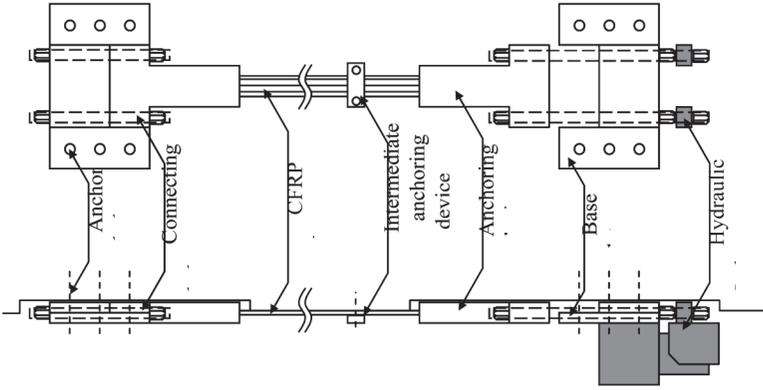
Figure 1—Tensioning system
