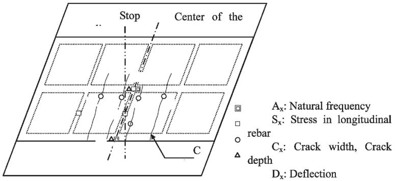
Figure 6—Measurement points of load test
