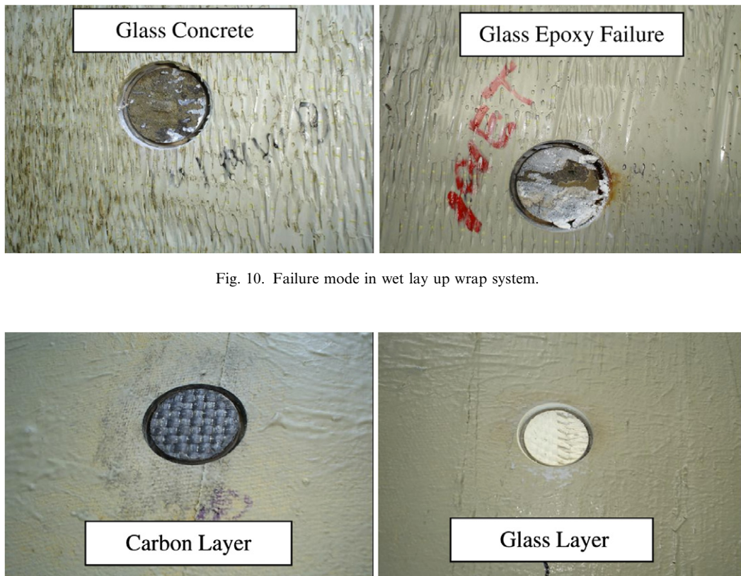
Fig. 11. Failure mode in pre-preg wrap system.
