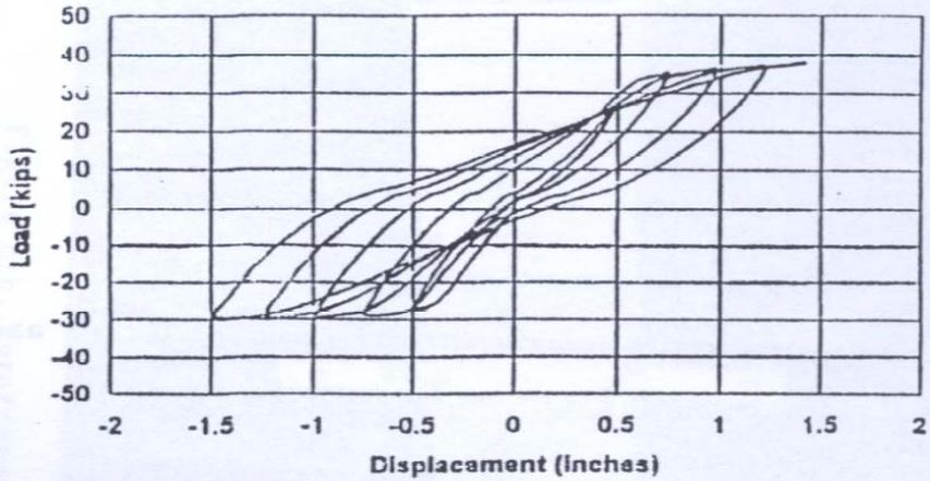
**Figure-1** Load-Deflection plot for the control specimen SP-1
