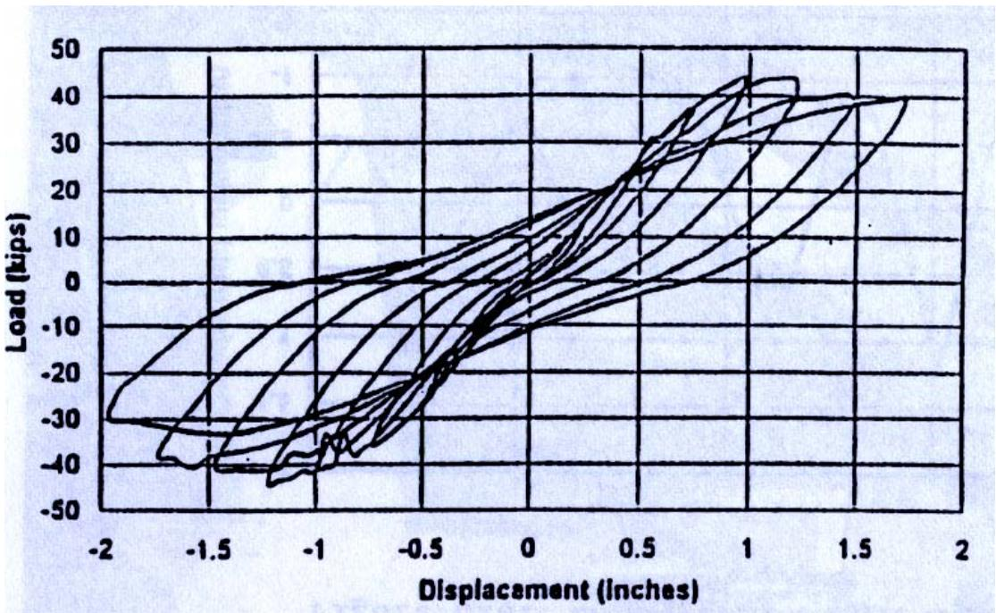
**Figure 2** Load-Deflection plot for the repaired control specimen with E-glass SP-1R
