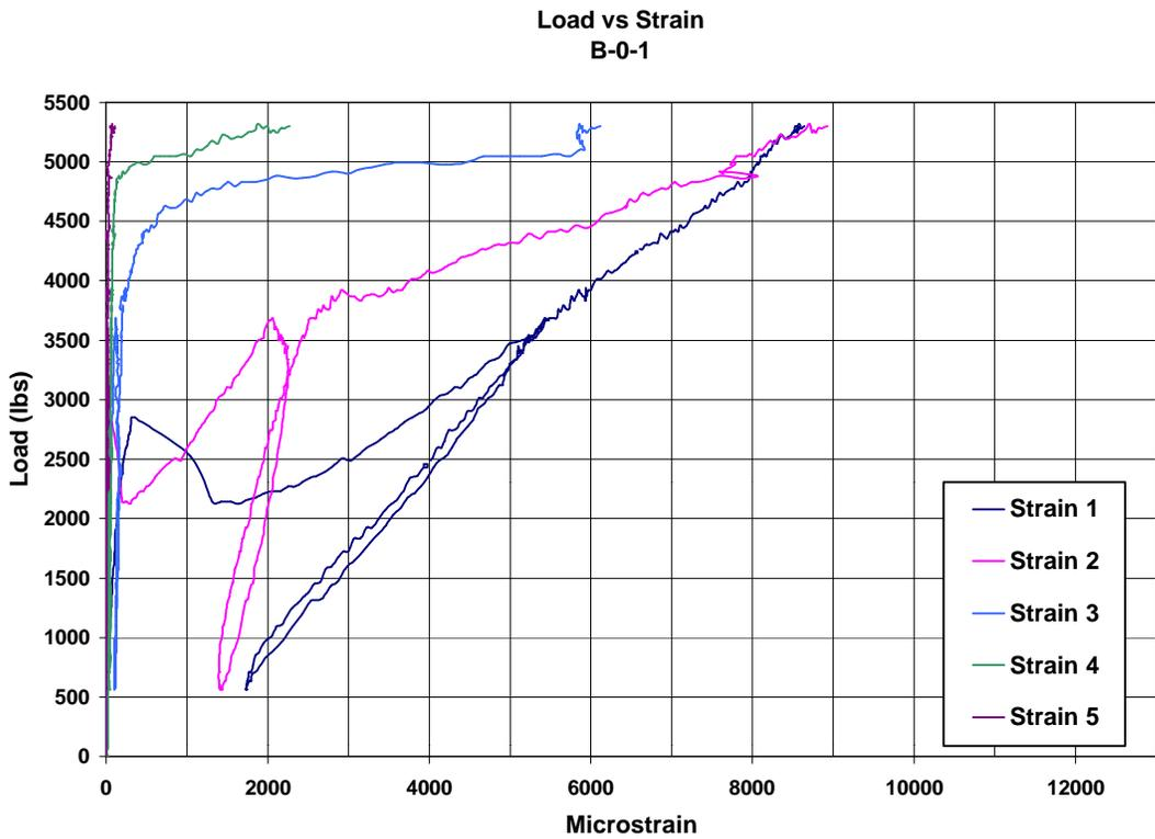
**Figure A.34. Load vs. Strain plot for B-0-1 (1 lb = 4.448 N)**
