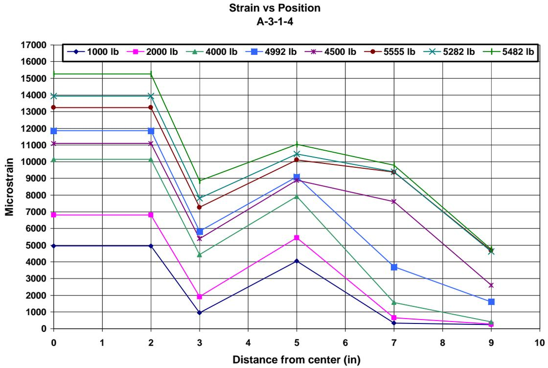
**Figure A.31. Strain vs. Position plot for A-3-1-4 (1 in = 25.4 mm, 1 lb = 4.448 N)**
