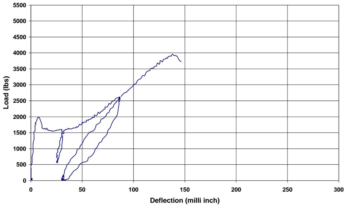
Figure A.57. Load vs. Deflection plot for B-3-1-u (1 in = 25.4 mm, 1 lb = 4.448 N)
