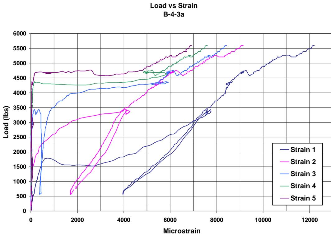
**Figure A.54. Load vs. Strain plot for B-4-3a (1lb = 4.448 N)**
