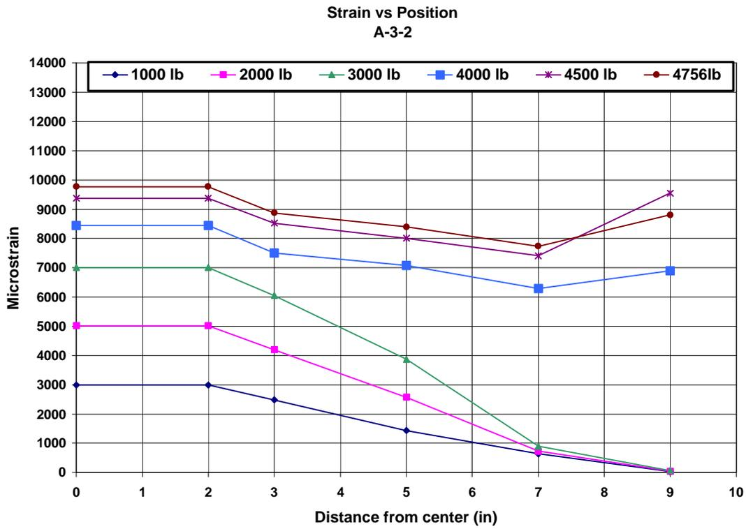
**Figure A.11. Strain vs. Position plot for A-3-2 (1 in = 25.4 mm, 1 lb = 4.448 N)**
