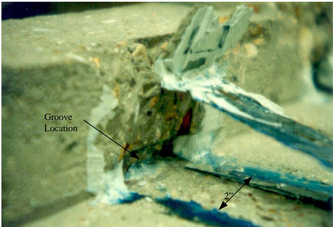
**Figure A.8. Picture of failure location for A-3-1 (1 in = 25.4 mm)**
