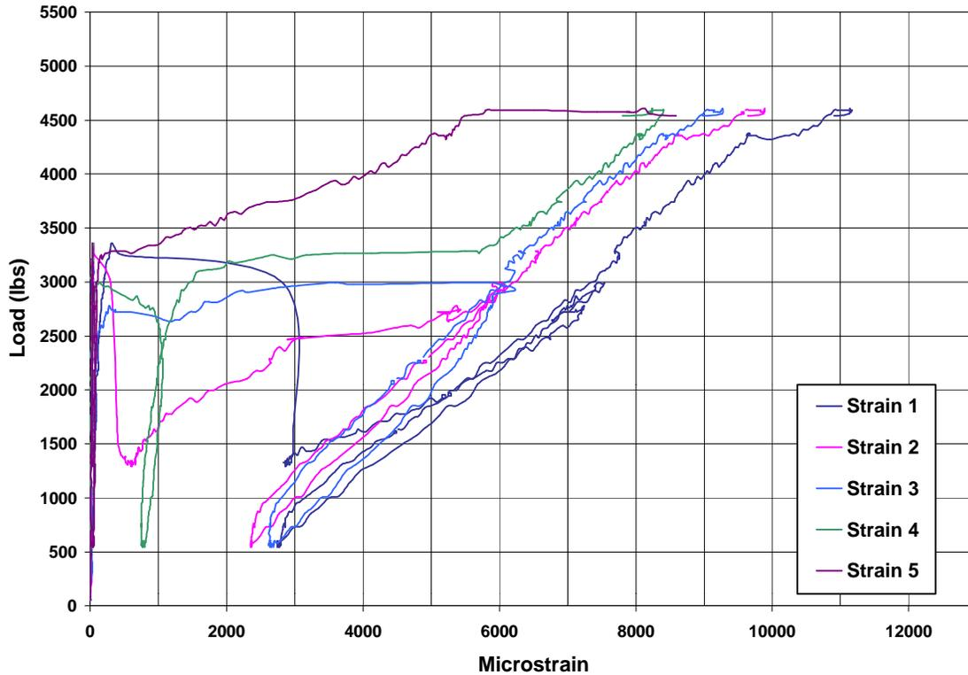
**Figure 4.2. Typical Load vs. Strain plot (A-0-1)**
