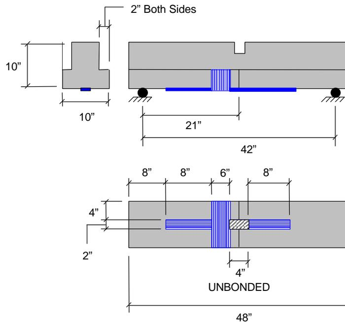
Figure 2.1. Dimensions and orientation of CFRP on flat beam (1 in = 25.4 mm)
