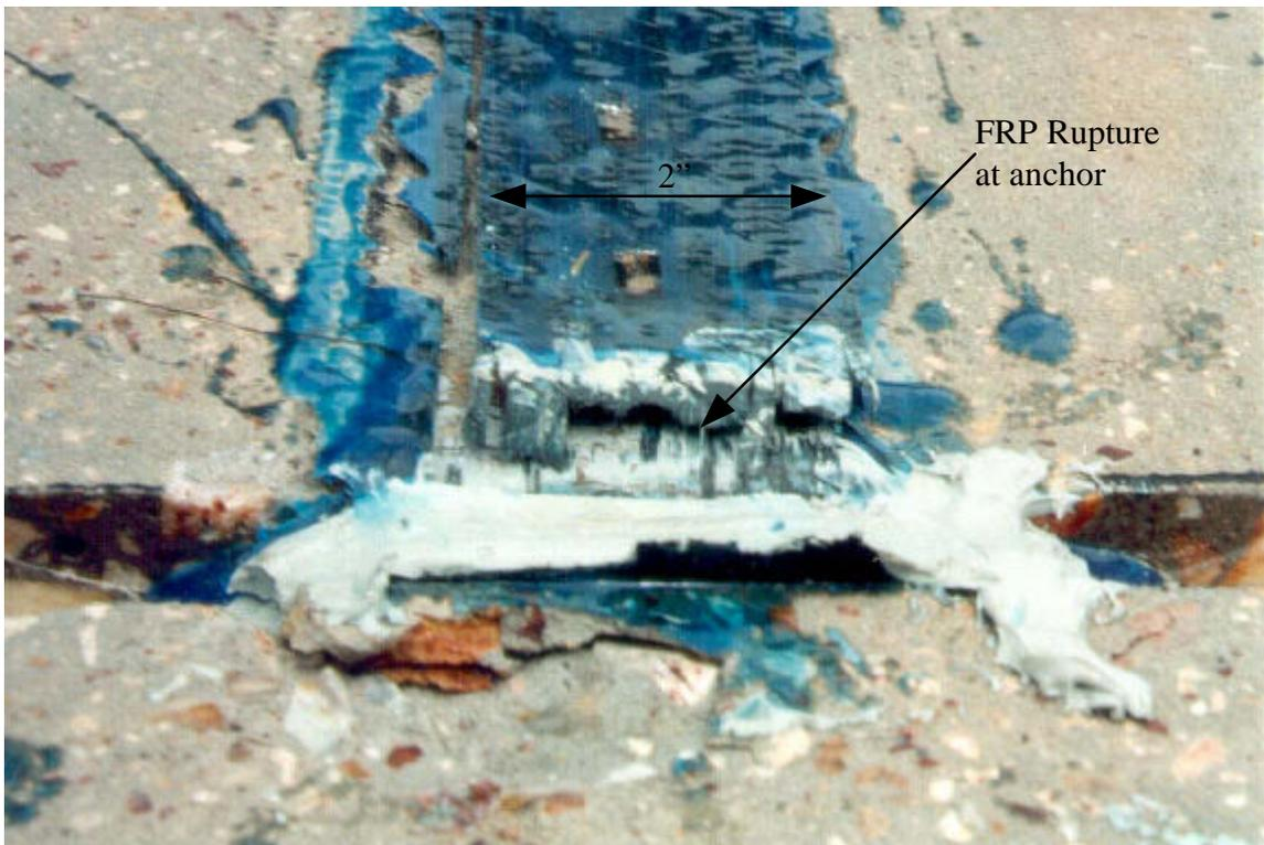
**Figure A.52. Picture of failure location for B-4-3 (1 in = 25.4 mm)**
