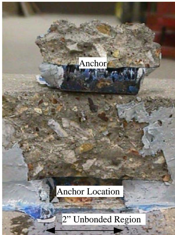
**Figure A.24. Picture of failure location for A-3-1-u (1 in = 25.4 mm)**
