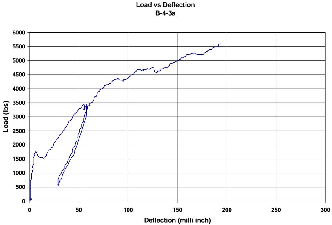
**Figure A.53. Load vs. Deflection plot for B-4-3a (1 in = 25.4 mm, 1lb = 4.448 N)**
