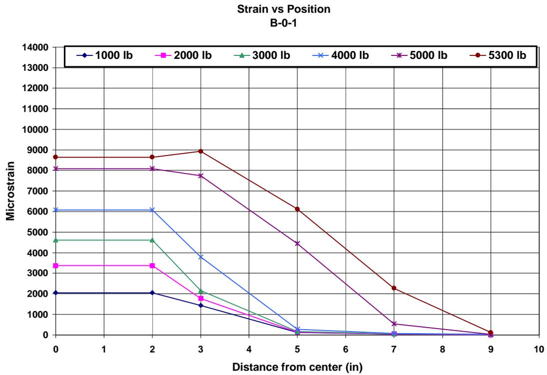
**Figure A.35. Strain vs. Position plot for B-0-1 (1 in = 25.4 mm, 1 lb = 4.448 N)**
