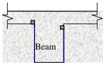
(a) Two options for anchorage of web shear strengthening of beams.
