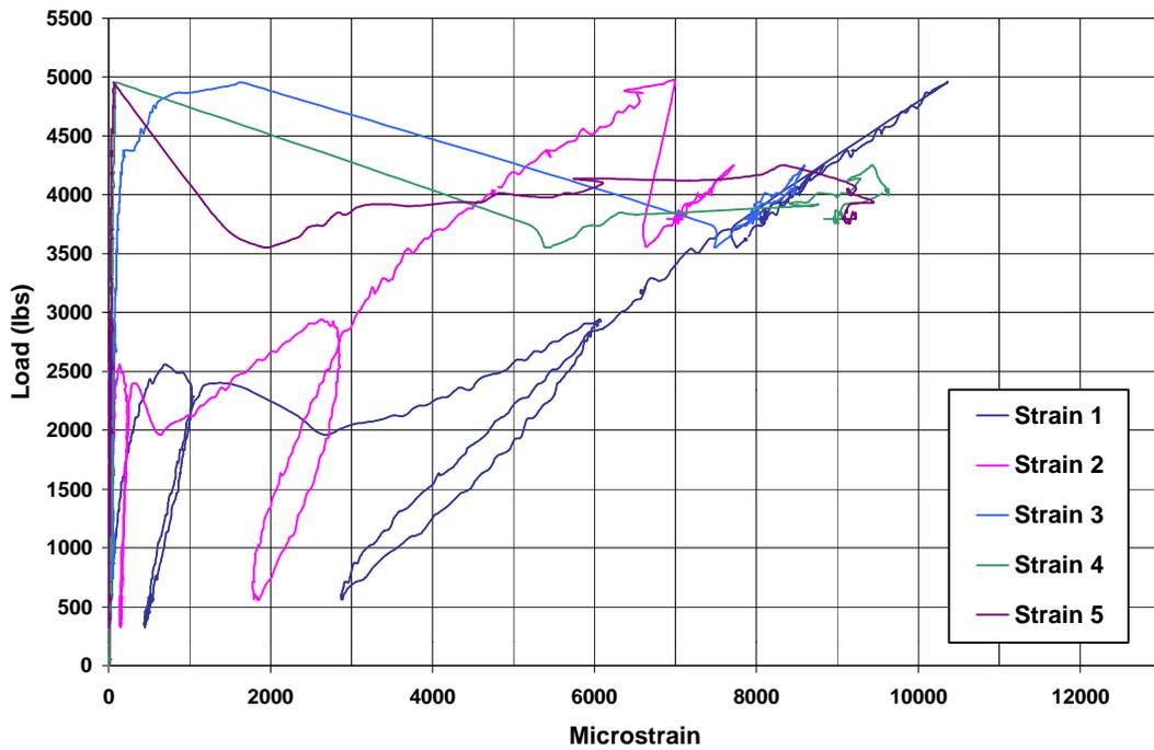
Figure A.46. Load vs. Strain plot for B-3-2 (1 lb = 4.448 N)
