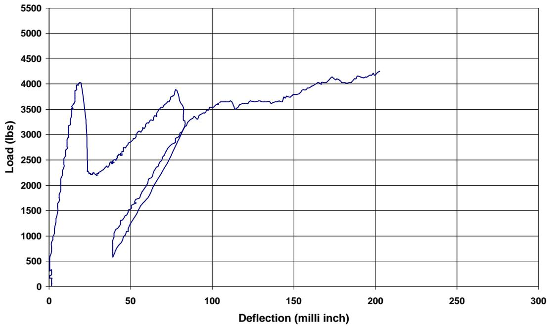
Figure A.17. Load vs. Deflection plot for A-4-3a (1 in = 25.4 mm, 1 lb = 4.448 N)
