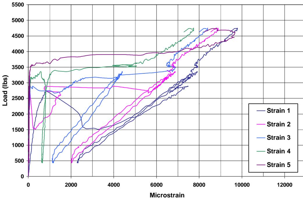
Figure A.10. Load vs. Strain plot for A-3-2 (1 lb = 4.448 N)
