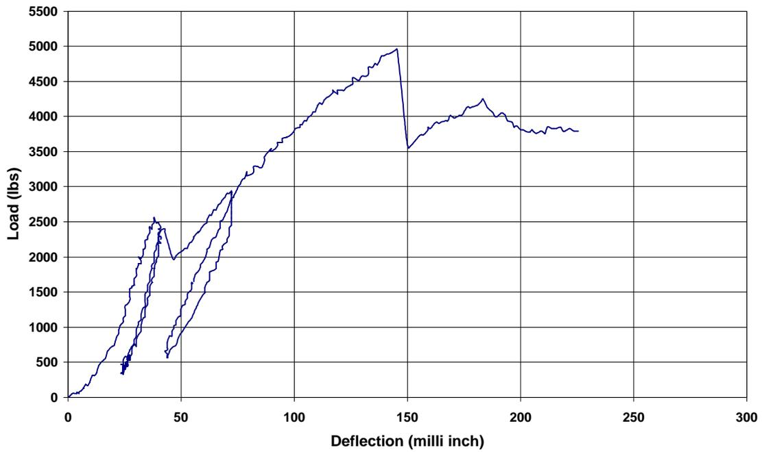
Figure A.45. Load vs. Deflection plot for B-3-2 (1 in = 25.4 mm, 1 lb = 4.448 N)
