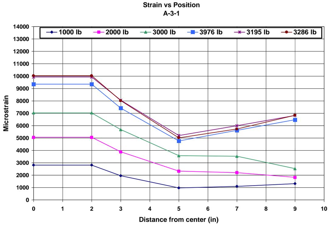
**Figure A.7. Strain vs. Position plot for A-3-1 (1 in = 25.4 mm, 1 lb = 4.448 N)**
