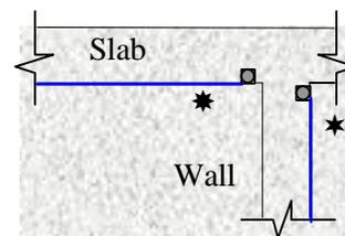
(b) ★Anchorage of flexural or shear strengthening in walls and ★ Anchorage of flexural strengthening in slabs or beams
