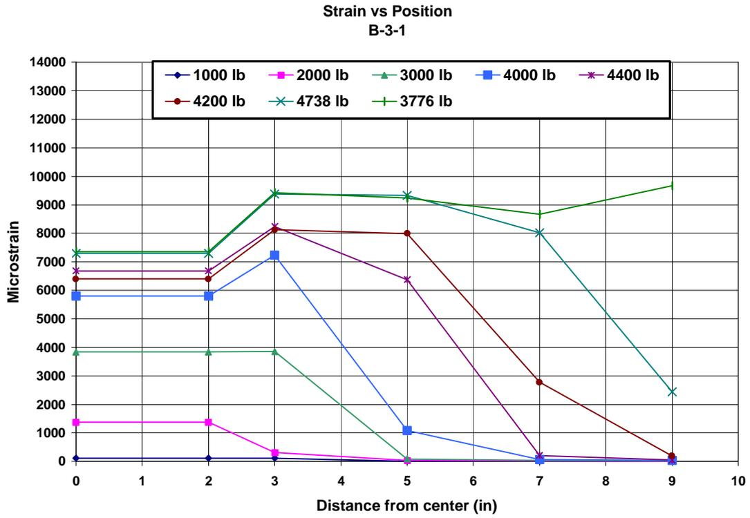
**Figure A.43. Strain vs. Position plot for B-3-1 (1 in = 25.4 mm, 1 lb = 4.448 N)**
