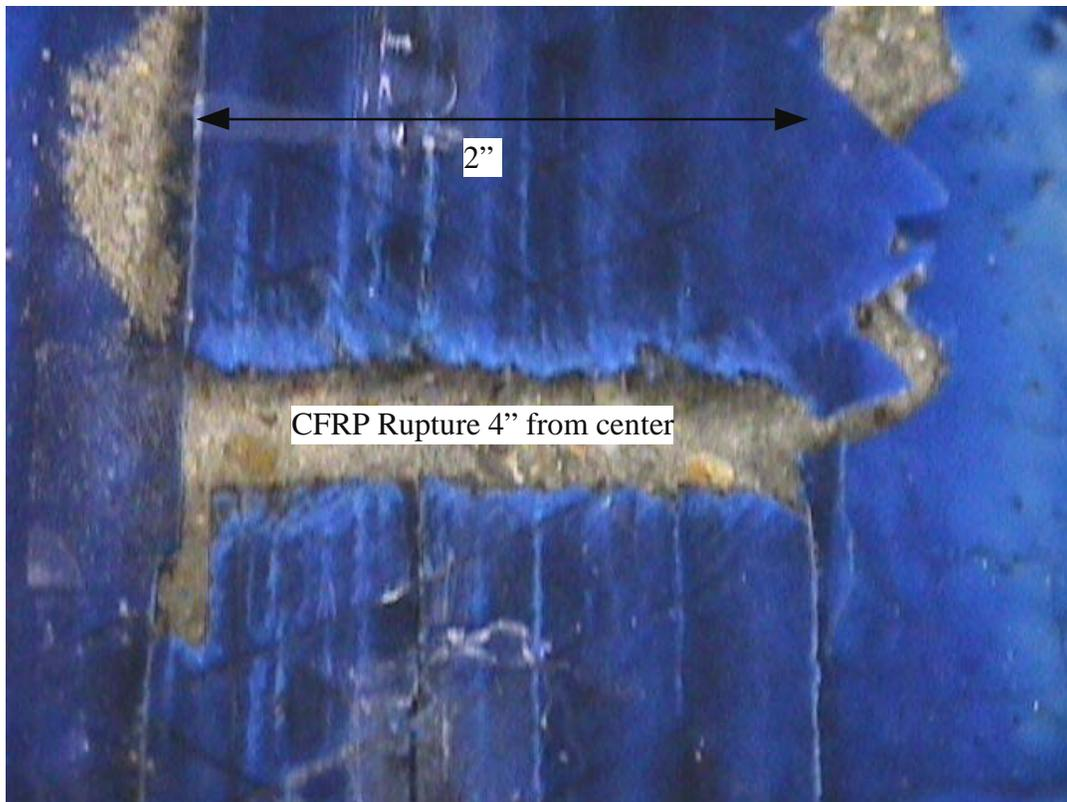
Figure A.20. Picture of failure location for A-4-3a (1 in = 25.4 mm)
