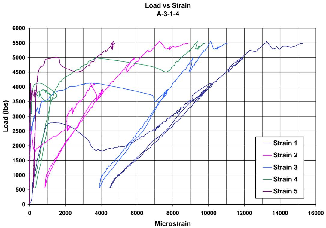
**Figure A.30. Load vs. Strain plot for A-3-1-4 (1 lb = 4.448 N)**
