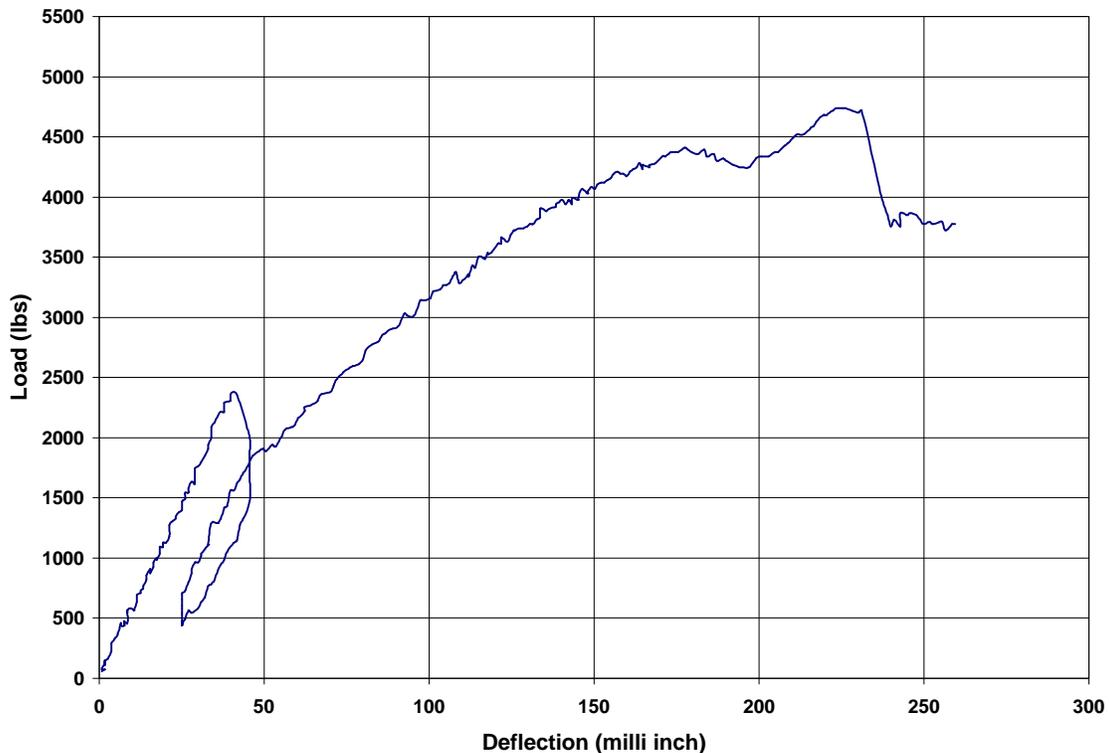
**Figure 4.1. Typical Load vs. Deflection plot (B-3-1)**
