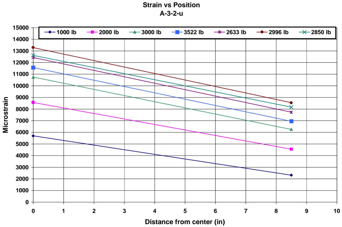
**Figure A.27. Strain vs. Position plot for A-3-2-u (1 in = 25.4 mm, 1 lb = 4.448 N)**
