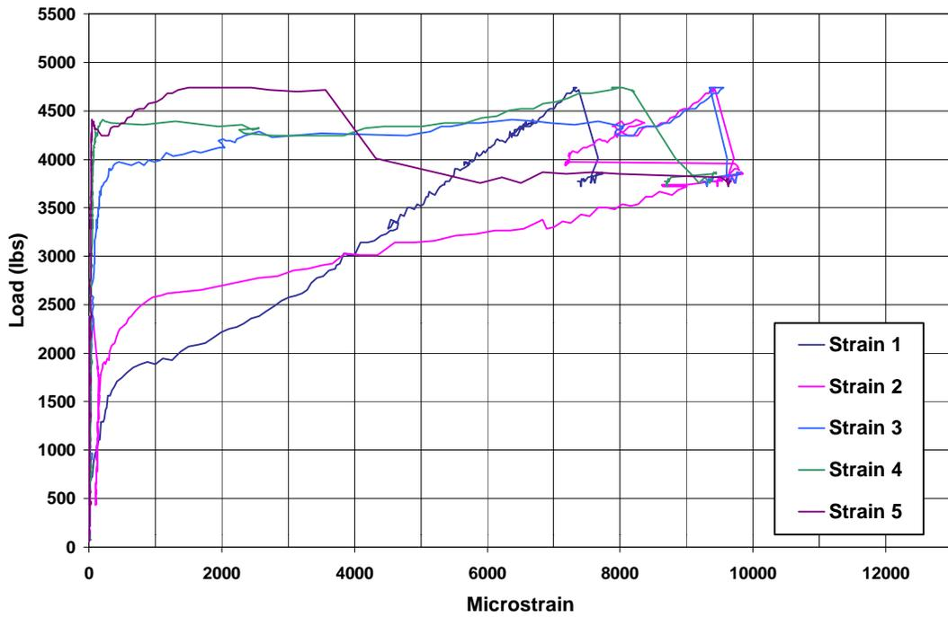
Figure A.42. Load vs. Strain plot for B-3-1 (1 lb = 4.448 N)
