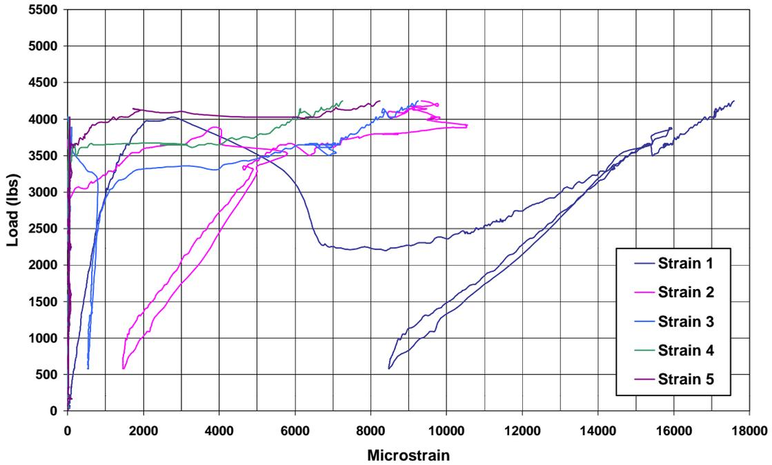
Figure A.18. Load vs. Strain plot for A-4-3a (1 lb = 4.448 N)
