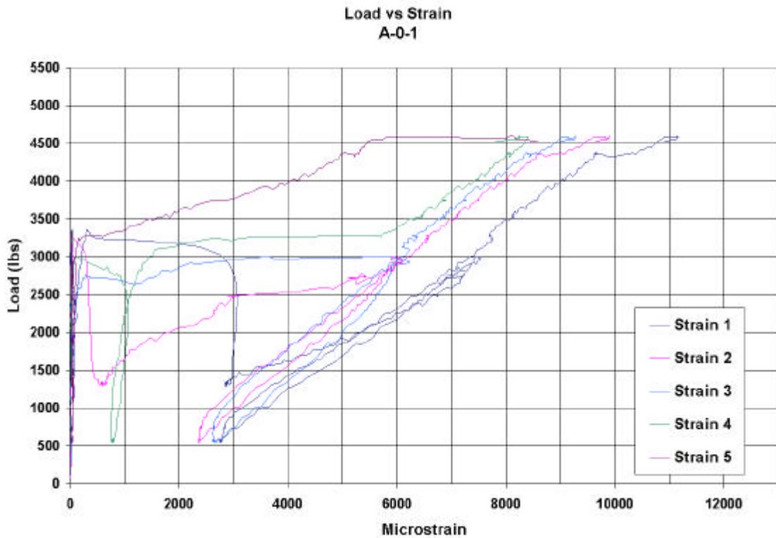
**Figure A.2. Load vs. Strain plot for A-0-1 (1 lb = 4.448 N)**
