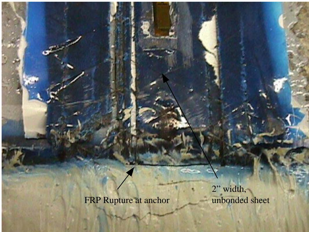
**Figure A.64. Picture of failure location for B-3-2-u (1 in = 25.4 mm)**
