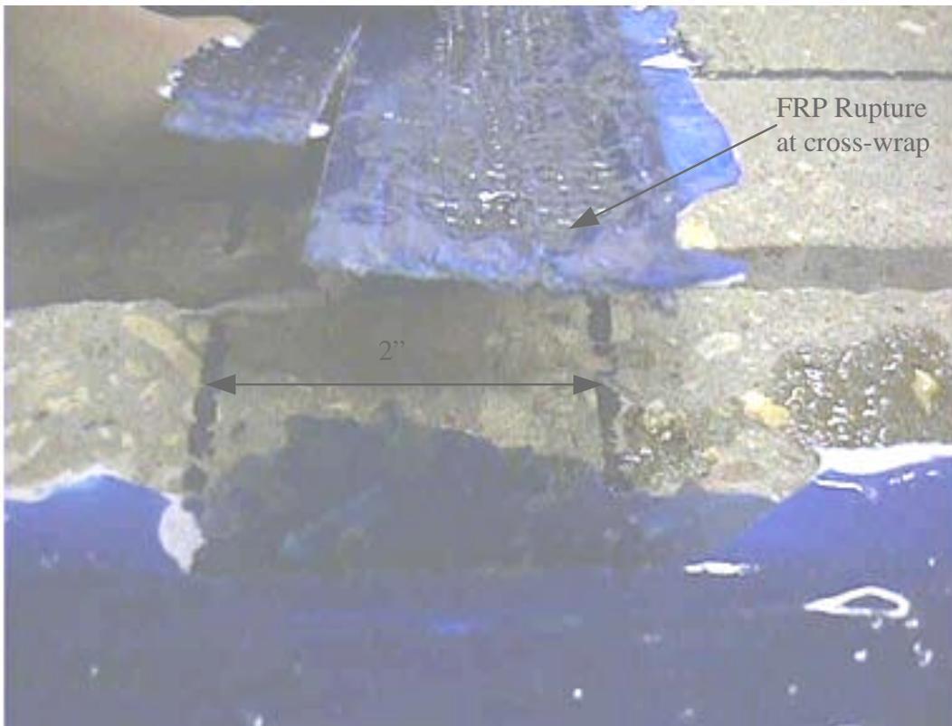
**Figure A.36. Picture of failure location for B-0-1 (1 in = 25.4 mm)**
