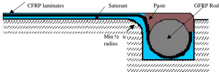
**Figure 1.2. Anchorage Mechanism cross-section**
