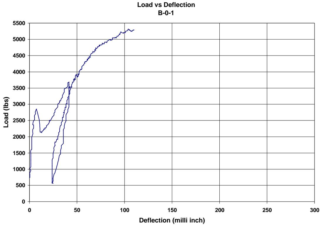
**Figure A.33. Load vs. Deflection plot for B-0-1 (1 in = 25.4 mm, 1 lb = 4.448 N)**
