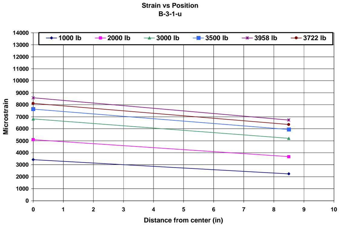
**Figure A.59. Strain vs. Position plot for B-3-1-u (1 in = 25.4 mm, 1 lb = 4.448 N)**
