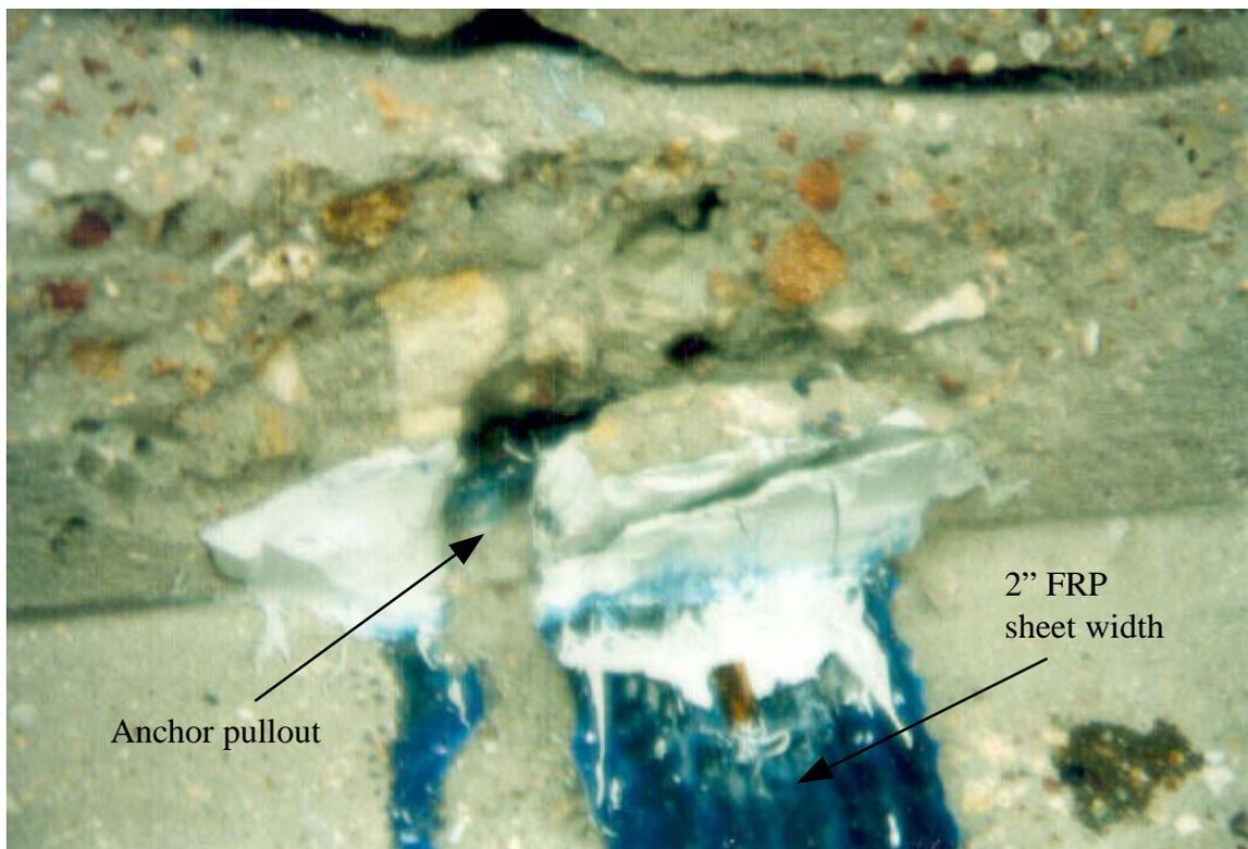
**Figure A.12. Picture of failure location for A-3-2 (1 in = 25.4 mm)**
