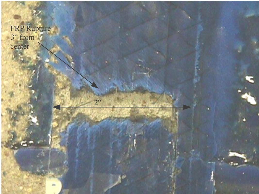
**Figure A.40. Picture of failure location for B-0-1a (1 in = 25.4 mm)**
