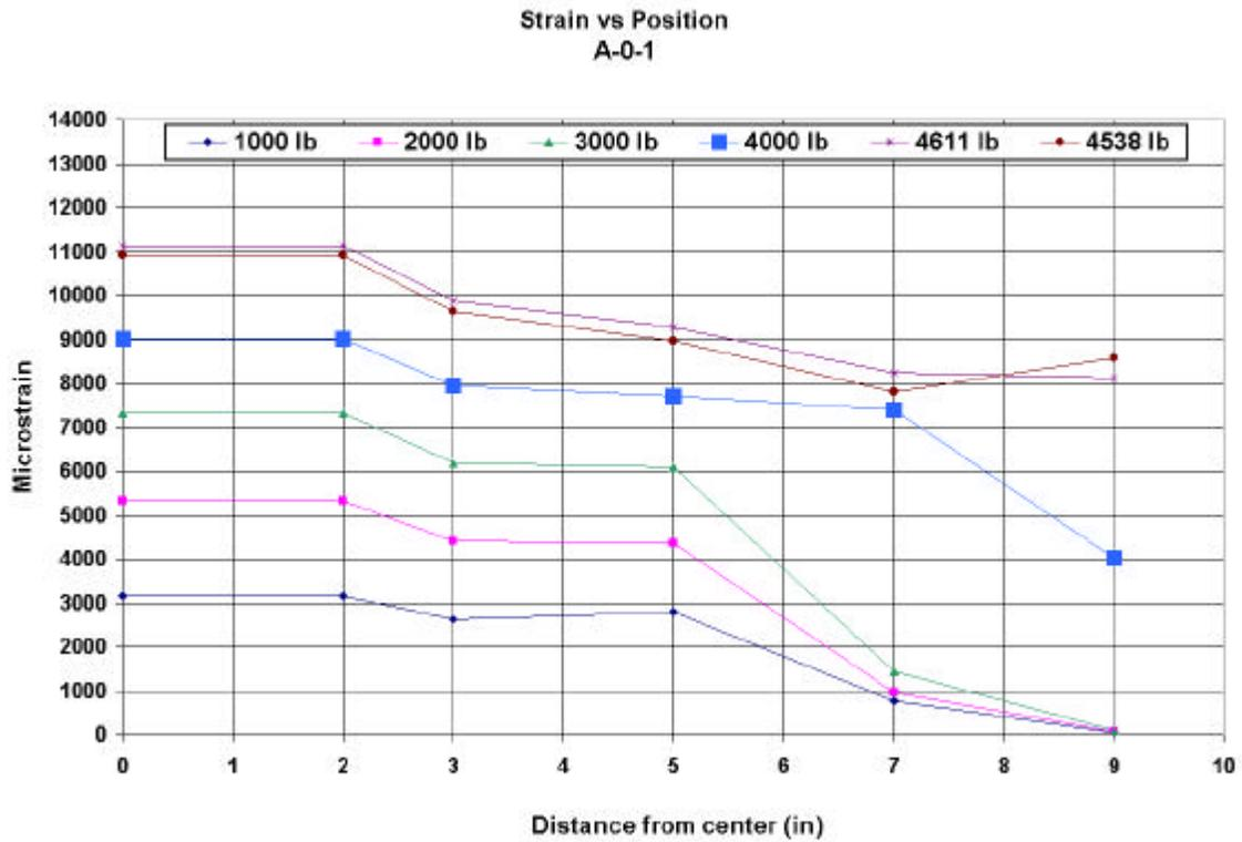
**Figure A.3. Strain vs. Position plot for A-0-1 (1 in = 25.4 mm, 1 lb = 4.448 N)**
