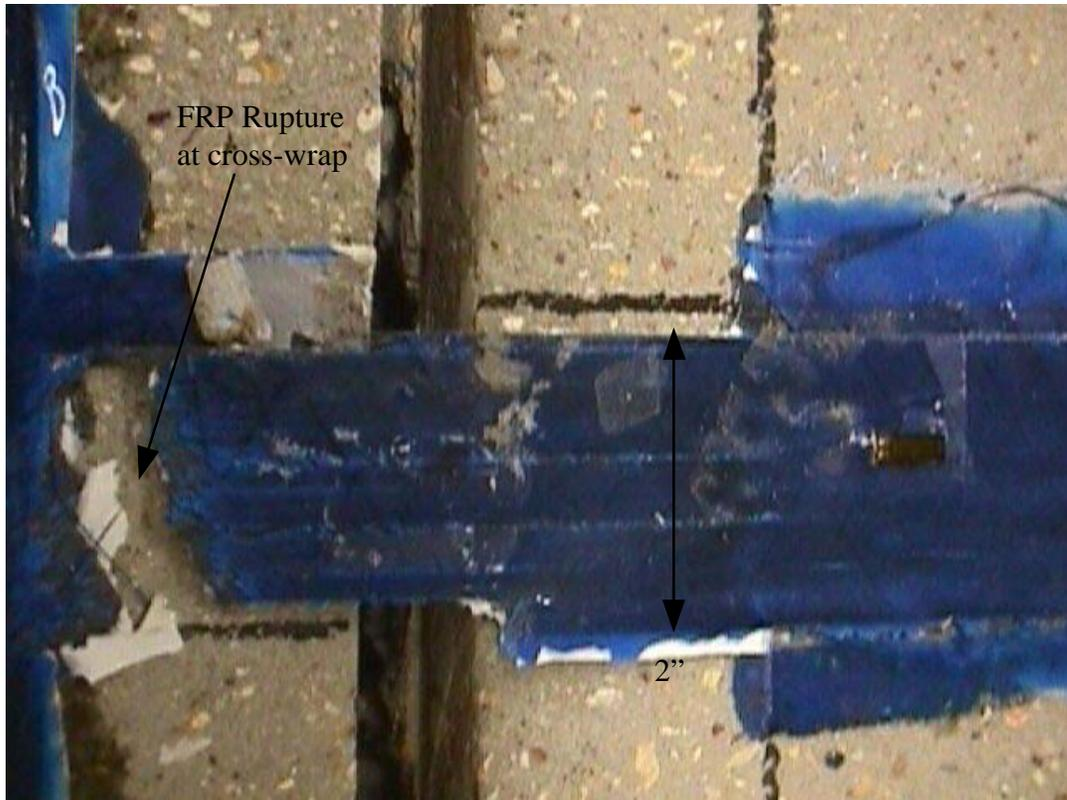
**Figure A.56. Picture of failure location for B-4-3a (1 in = 25.4 mm)**
