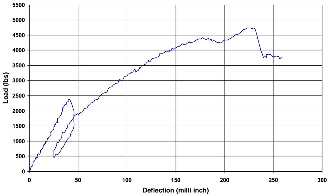
Figure A.41. Load vs. Deflection plot for B-3-1 (1 in = 25.4 mm, 1 lb = 4.448 N)
