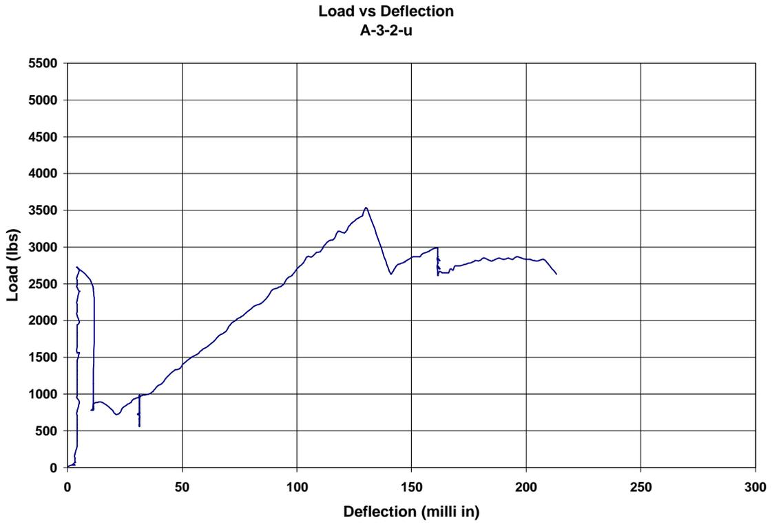
**Figure A.25. Load vs. Deflection plot for A-3-2-u (1 in = 25.4 mm, 1 lb = 4.448 N)**
