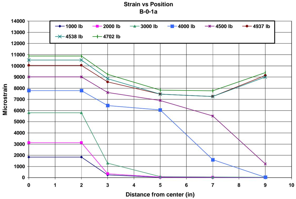
**Figure A.39. Strain vs. Position plot for B-0-1a (1 in = 25.4 mm, 1 lb = 4.448 N)**
