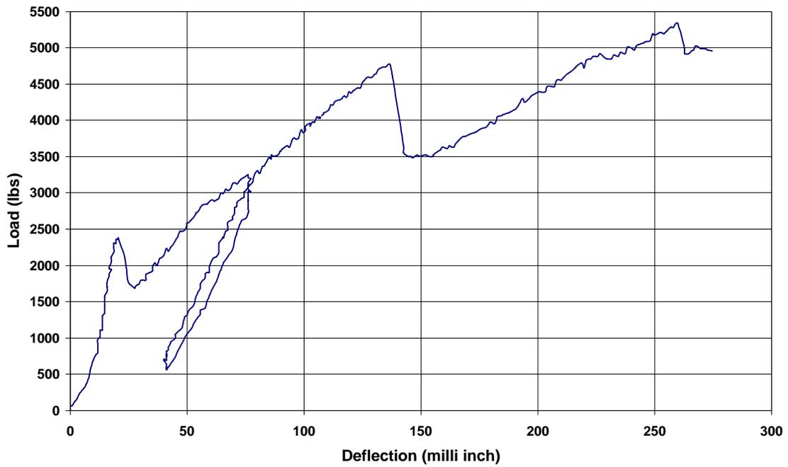
Figure A.49. Load vs. Deflection plot for B-4-3 (1 in = 25.4 mm, 1 lb = 4.448 N)
