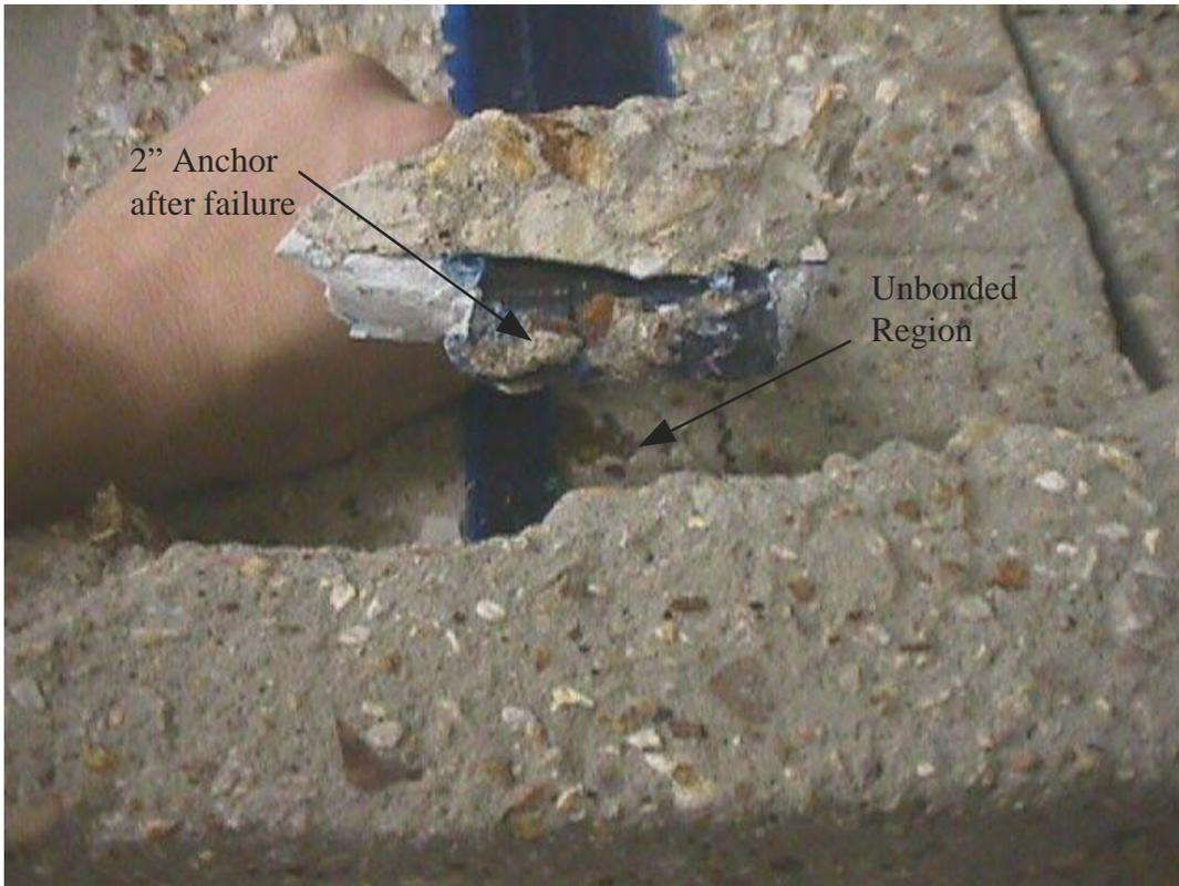
**Figure A.28. Picture of failure location for A-3-2-u (1 in = 25.4 mm)**
