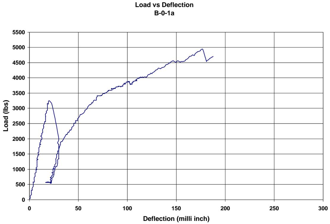
**Figure A.37. Load vs. Deflection plot for B-0-1a (1 in = 25.4 mm, 1 lb = 4.448 N)**
