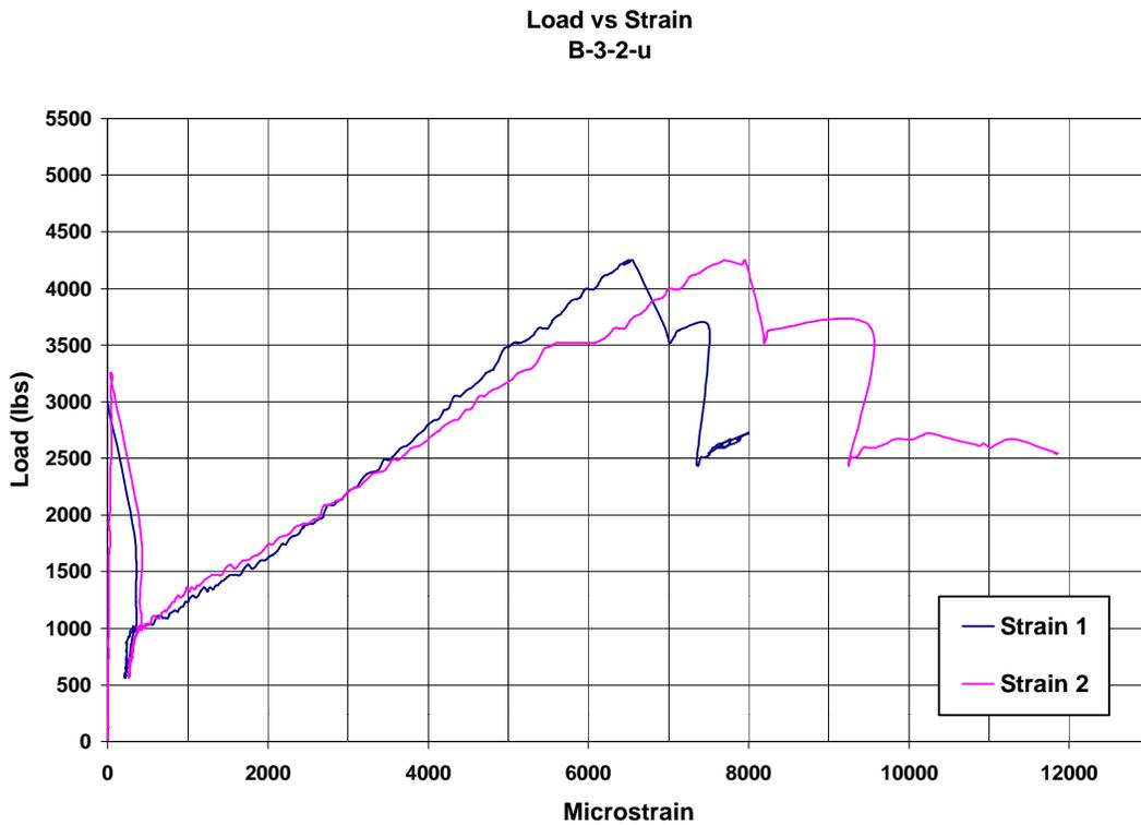
**Figure A.62. Load vs. Strain plot for B-3-2-u (1 lb = 4.448 N)**
