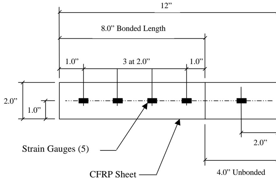
**Figure 3.1. Placement of strain gauges (1 in = 25.4 mm)**
