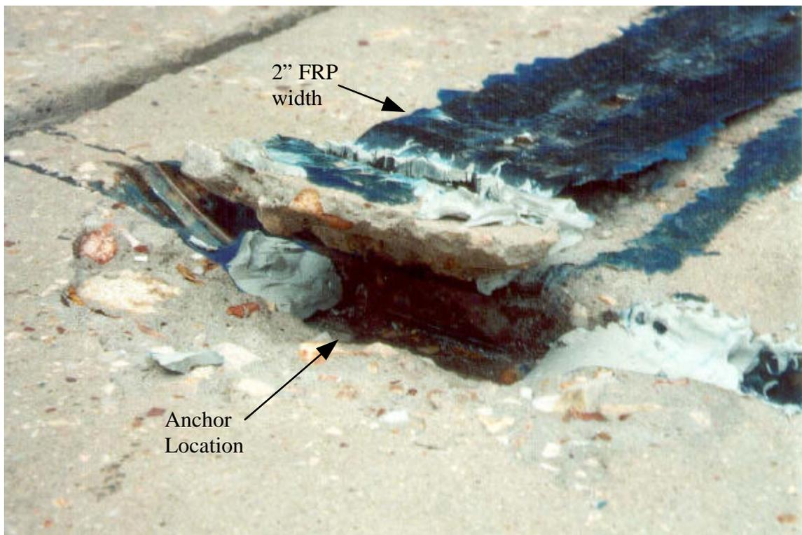
**Figure A.48. Picture of failure location for B-3-2 (1 in = 25.4 mm)**
