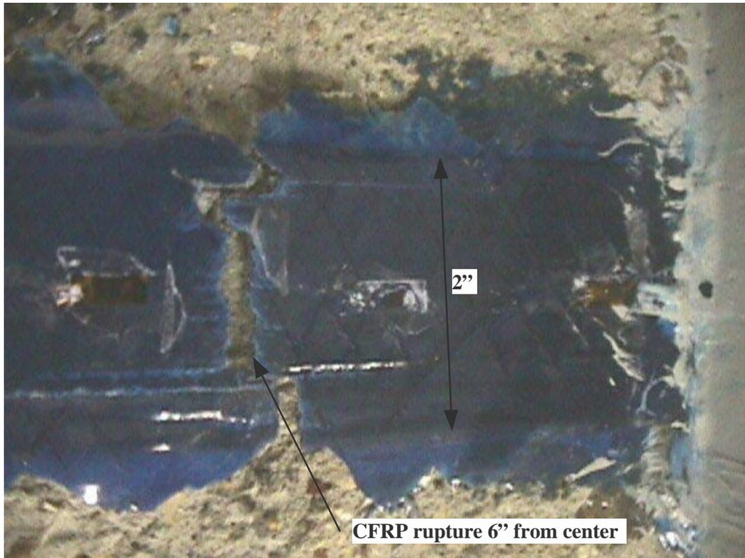
**Figure A.32. Picture of failure location for A-3-1-4 (1 in = 25.4 mm)**
