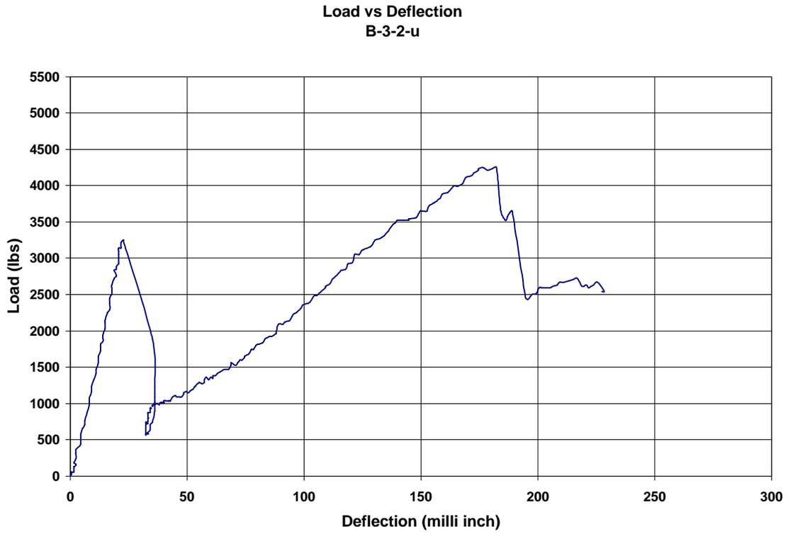
**Figure A.61. Load vs. Deflection plot for B-3-2-u (1 in = 25.4 mm, 1 lb = 4.448 N)**
