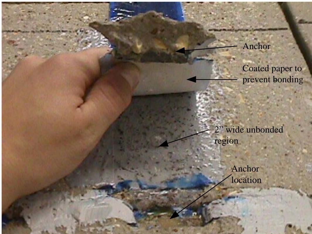
**Figure A.60. Picture of failure location for B-3-1-u (1 in = 25.4 mm)**
