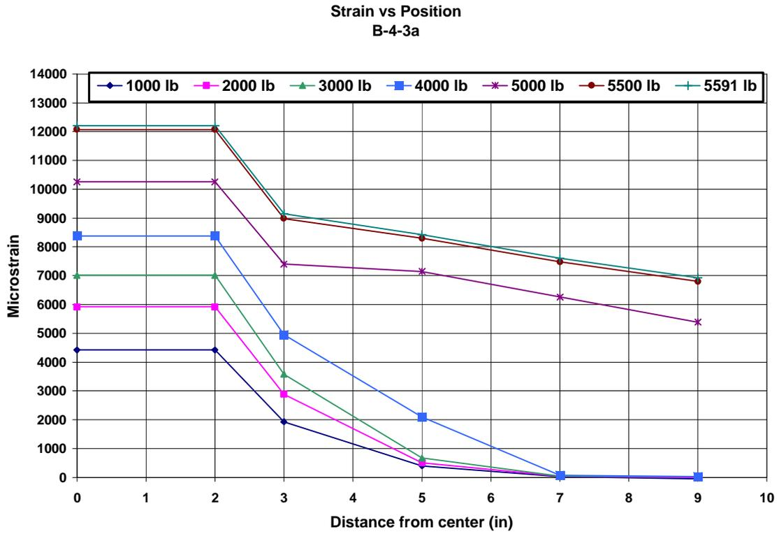
**Figure A.55. Strain vs. Position plot for B-4-3a (1 in = 25.4 mm, 1lb = 4.448 N)**
