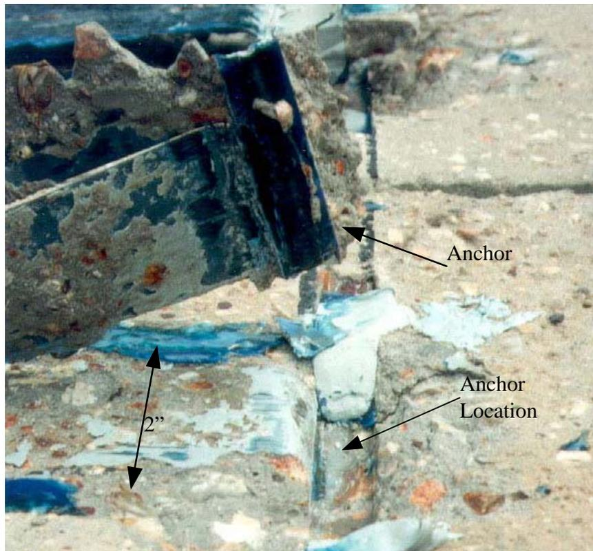
**Figure A.44. Picture of failure location for B-3-1 (1 in = 25.4 mm)**
