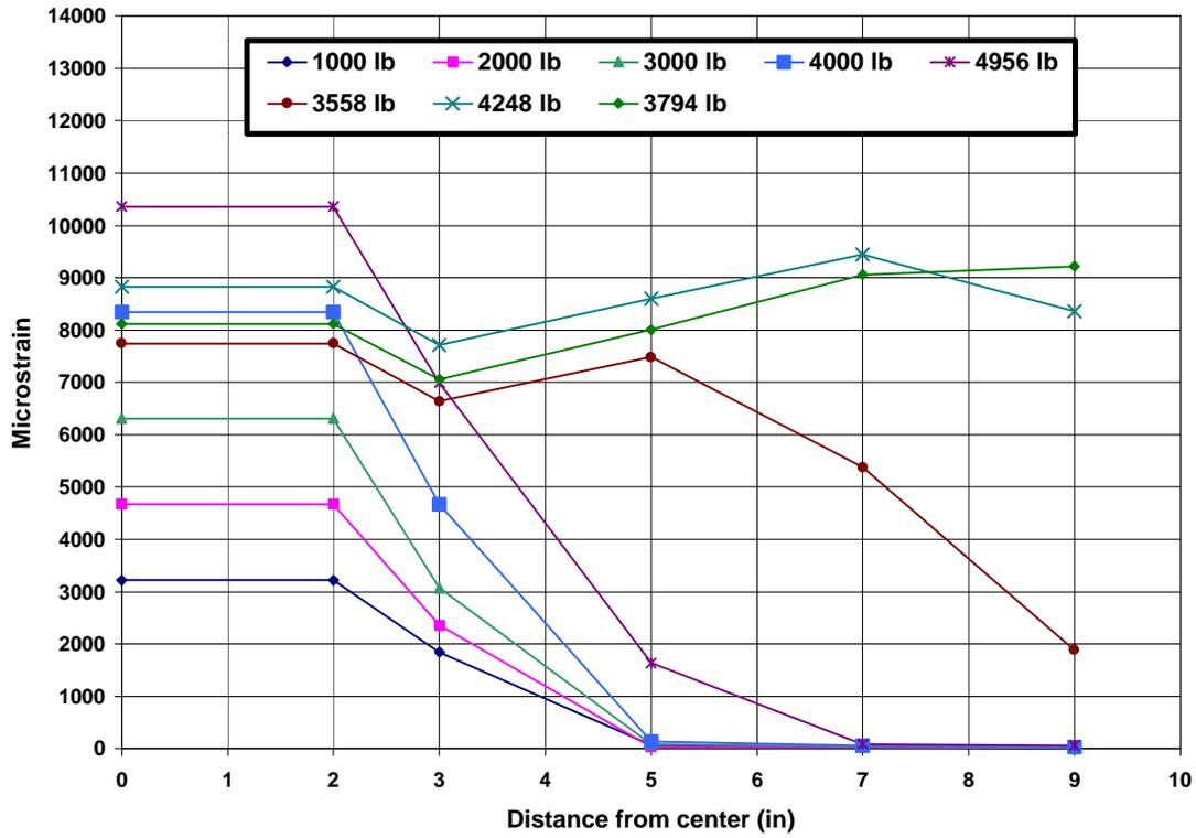
**Figure 4.3. Typical Strain vs. Position plot (B-3-2)**
