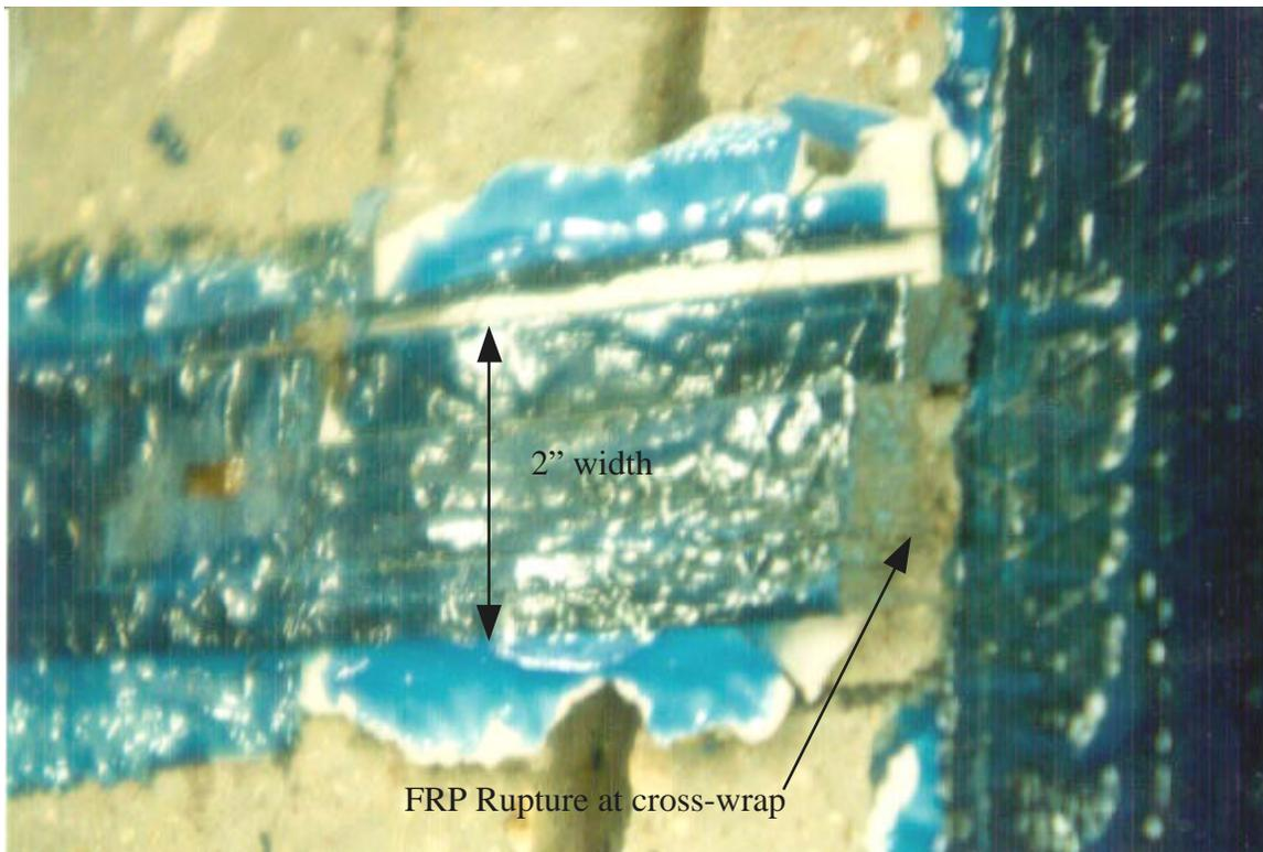
**Figure A.16. Picture of failure location for A-4-3 (1 in = 25.4 mm)**
