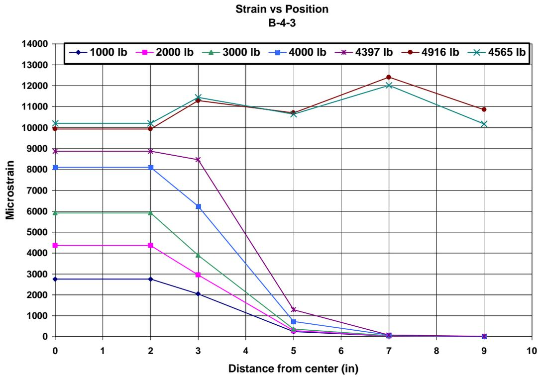
**Figure A.51. Strain vs. Position plot for B-4-3 (1 in = 25.4 mm, 1 lb = 4.448 N)**
