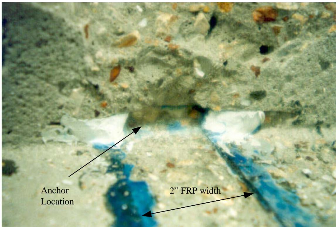
**Figure A.4. Picture of failure location for A-0-1 (1 in = 25.4 mm)**
