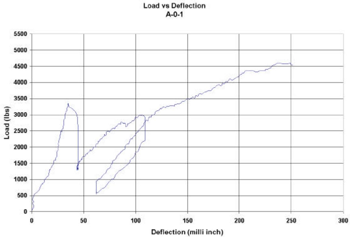
**Figure A.1. Load vs. Deflection plot for A-0-1 (1 in = 25.4 mm, 1 lb = 4.448 N)**
