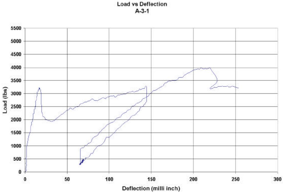
**Figure A.5. Load vs. Deflection plot for A-3-1 (1 in = 25.4 mm, 1 lb = 4.448 N)**
