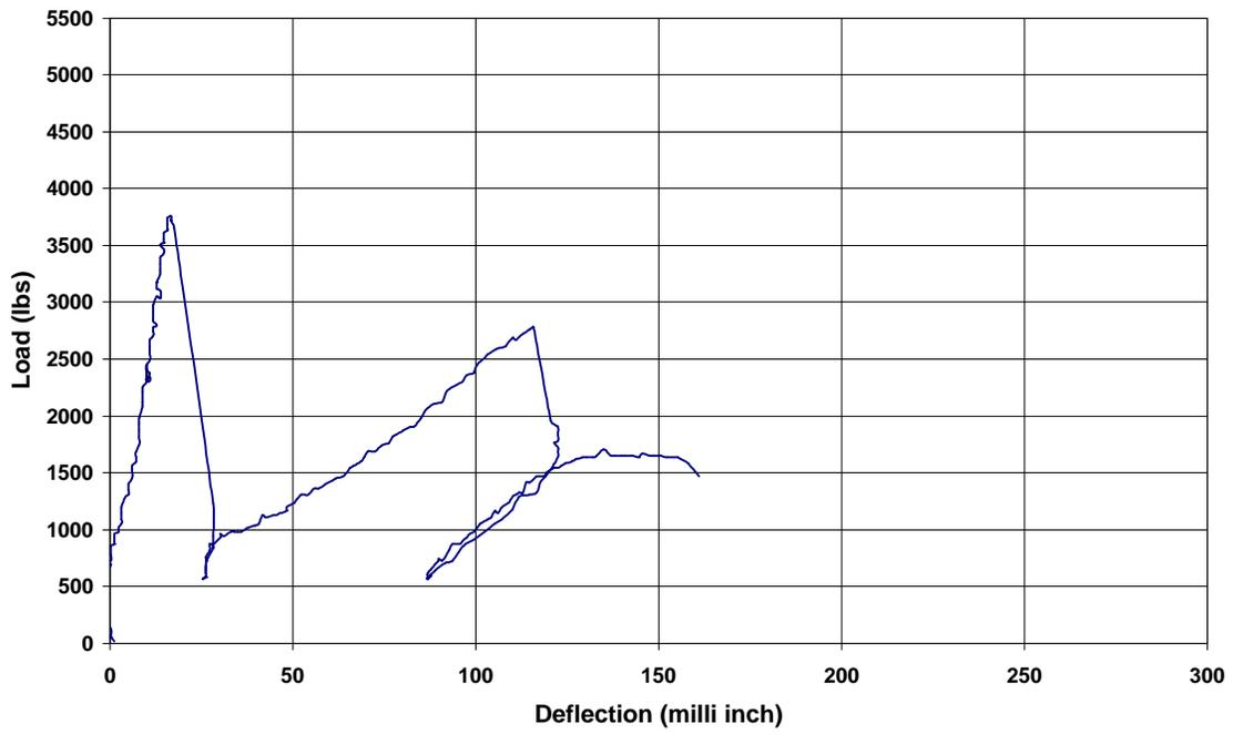
Figure A.21. Load vs. Deflection plot for A-3-1-u (1 in = 25.4 mm, 1 lb = 4.448 N)
