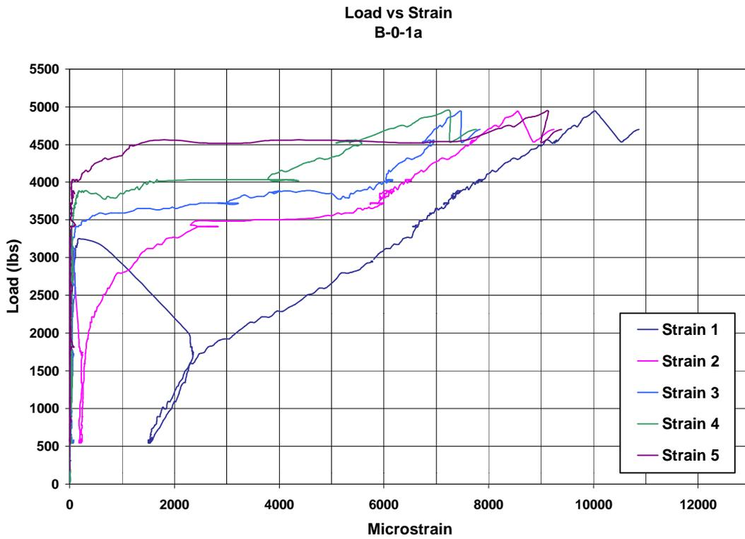
**Figure A.38. Load vs. Strain plot for B-0-1a (1 lb = 4.448 N)**
