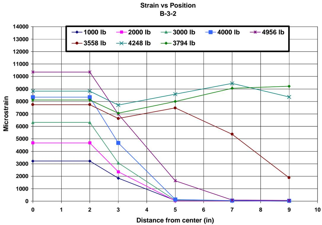
**Figure A.47. Strain vs. Position plot for B-3-2 (1 in = 25.4 mm, 1 lb = 4.448 N)**
