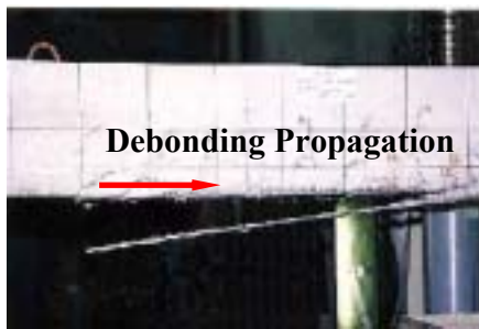
(b) Delamination of FRP at FRP ends
