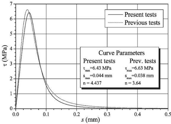
Figure 7—Comparison between interface laws calibrated with present experimental results and previous results by Mazzotti et al. <sup>9</sup>
