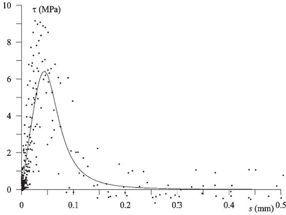
Figure 6—Shear stress-slip data obtained by post-processing experimental results from SP1 and SP2 specimens and proposed interface law.
