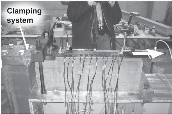
Figure 2—Experimental set-up: view of the clamping system for concrete and plate at the opposite sides of the specimen.
