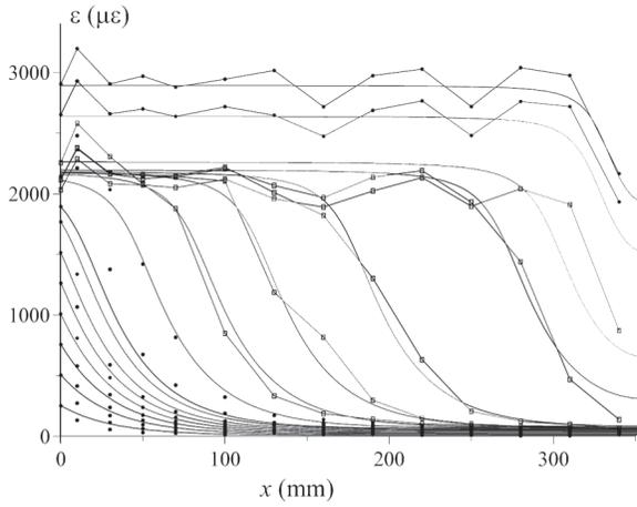
Figure 8—Profiles of strains along FRP plate: comparison between numerical and experimental results from specimen SP<sub>1</sub>;  $\square$ —measures taken during delamination phase.
