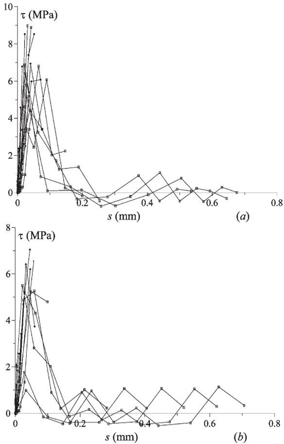
Figure 5—Shear stress—slip data obtained from post-processing experimental results from (a) SP1 and (b) SP2 specimens;  $\square$ —measures taken during delamination phase.
