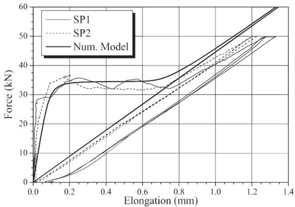
Figure 3—Force-plate elongation curves from experimental tests (specimens SP1, SP2) and numerical simulations.
