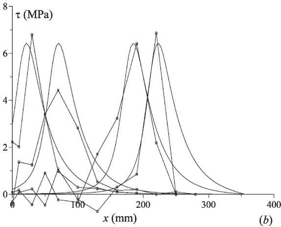
Figure 9—Profiles of shear stressed along FRP plate for specimen SP1. Comparison between numerical and experimental results for: (a) low and (b) high loading levels;  $\square$ —measures taken during delamination phase.
