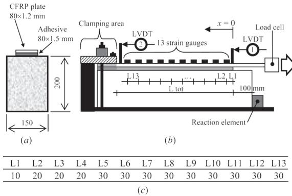
Figure 1—Experimental set-up: (a) Specimen transverse section, (b) side view with instrument positions and CFRP plate clamping system, (c) spacing between strain gauges (mm) along the CFRP plate.
