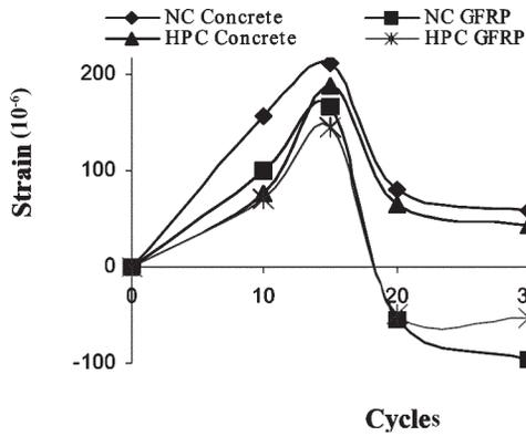
Fig. 11 - Strain behavior of WD conditioned specimens
