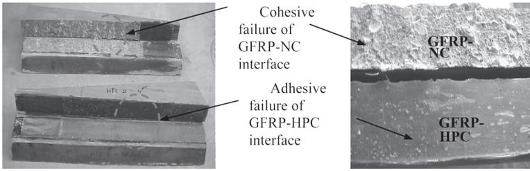
Fig. 6 - Typical fracture surfaces of GFRP-NC and GFRP-HPC specimens after dry fracture test
