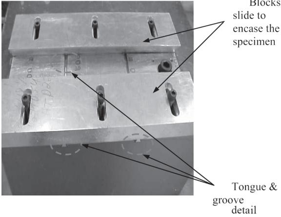
Fig. 2 - Single Contour Cantilever Beam Specimen Fixture
