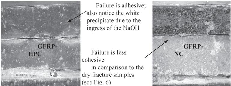
Fig. 13 - Typical Fracture Surfaces after 10 Wet-Dry Cycles
