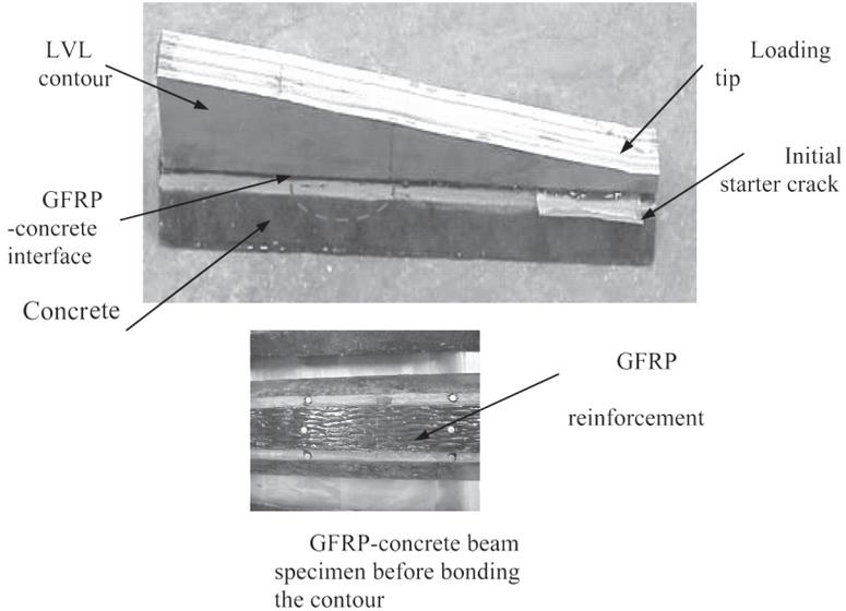
Fig. 3 - Single Contour Cantilever Beam Specimen
