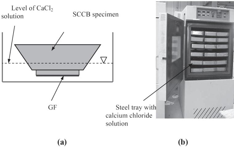
Fig. 7 - FT cycling of specimen within: (a) a tray, and (b) an environmental chamber
