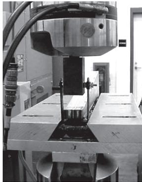
**Fig. 1 - Single Contour Cantilever Beam Specimen and Fixture**
