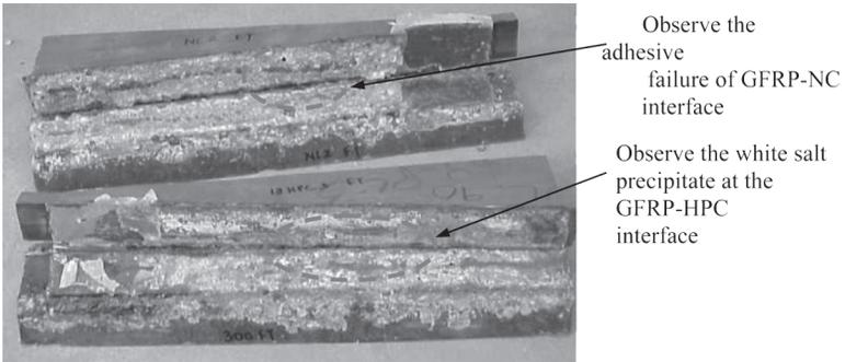
Fig. 10 Fracture surface after 300 FT cycles
