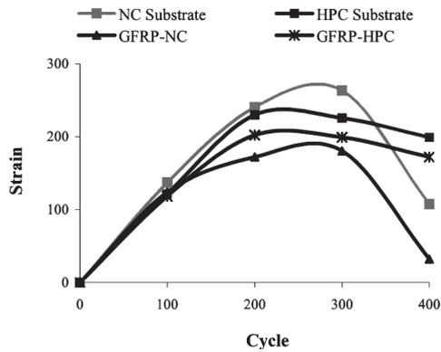
Fig. 8 - Strains in GFRP-NC & GFRP-HPC interfaces
