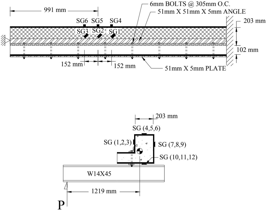
Figure 1. FRP Strengthened Specimen Detail
