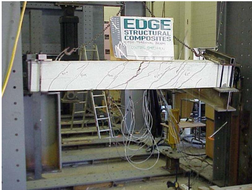
**Figure 2.** Baseline Specimen (TB6) Failure Mode
