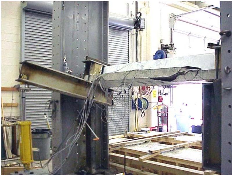
**Figure 3.** Strengthened Specimen (TB2) Failure Mode
