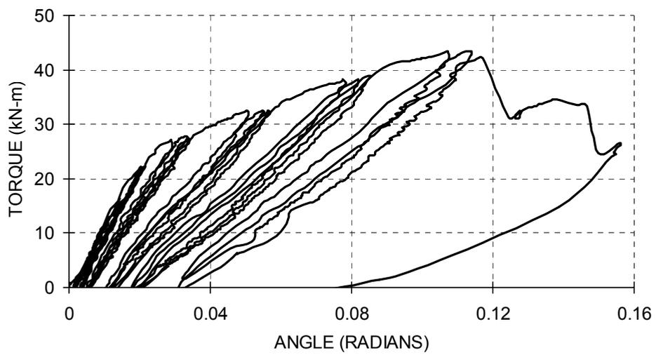
**Figure 4.** Specimen TB3 – Torque vs. Angle of Rotation
