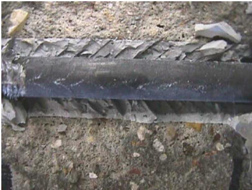
**Figure 3.42. Internal Cracks in Specimen C3S6a**
