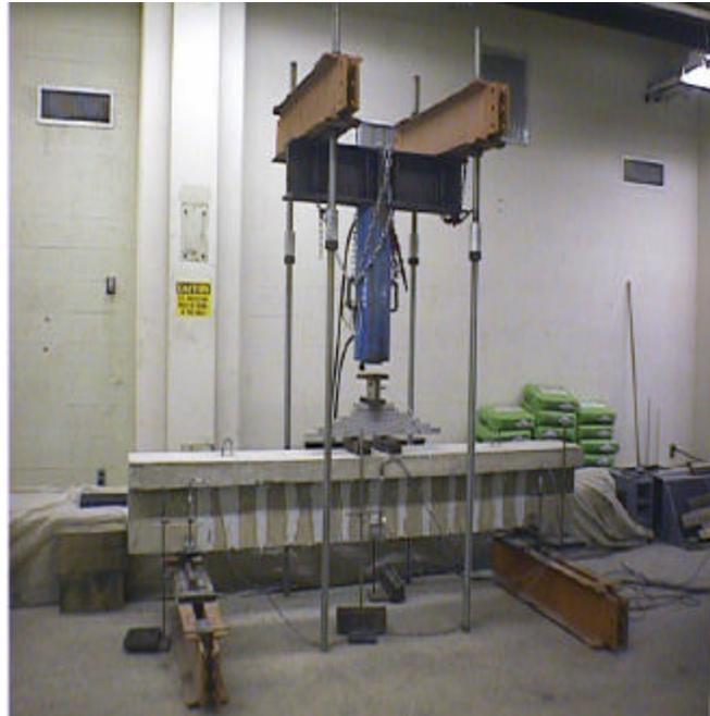
**Figure 5.5. Test Setup of Beam B90-7**
