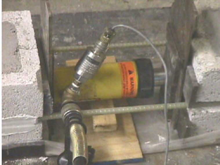
**Figure 4.8. Detail of Hydraulic Jack and Pressure Transducer**
