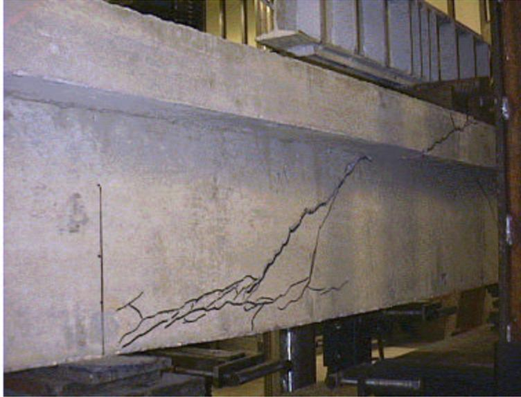
**Figure 5.6. Failure of Beam BV**
