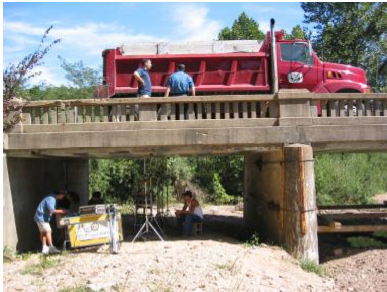
Figure 4-1 – Load Test with H20 Truck
