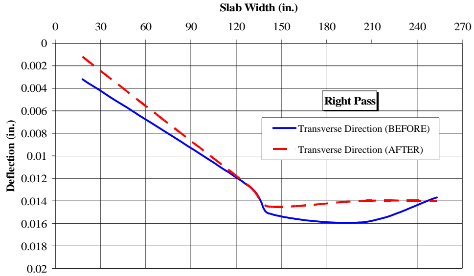
Figure 4-6 – Mid Span Deflection in the Transverse Direction, Stop No.3
