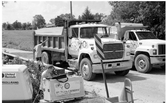
**Figure 6.** Bridge In-situ load testing
