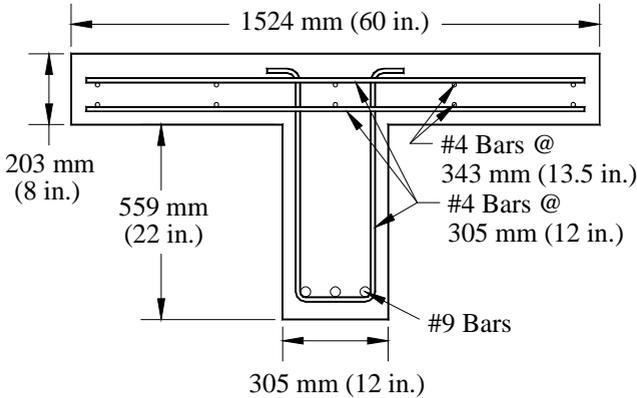
**Figure 1.** Internal steel layout of T beams.
