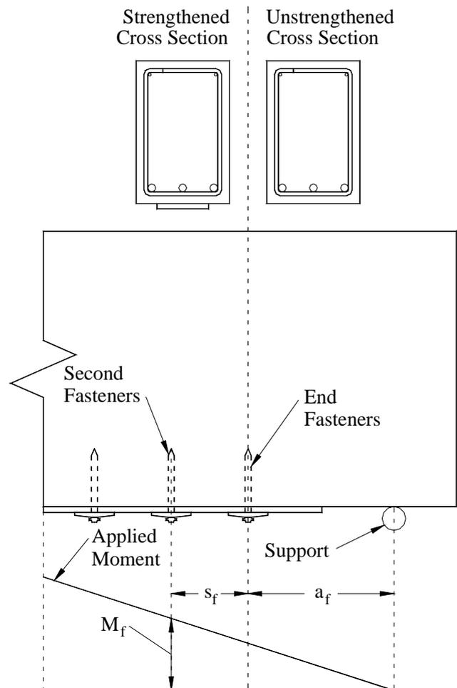
**Figure 5.** Close up of end fastener distance and applied moment diagram.
