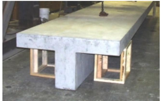
**Figure 2.** A T beam after it was removed from the formwork.
