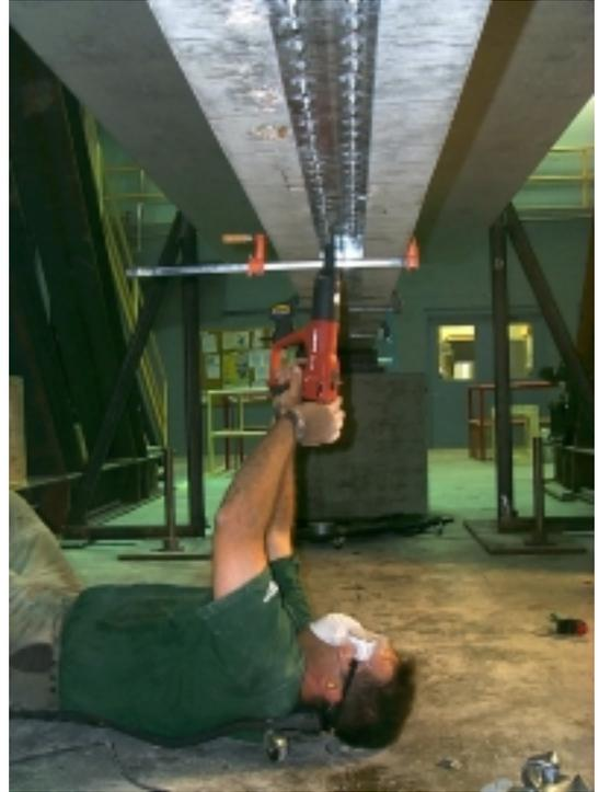
**Figure 3.** Fastener being driven to attach the strip.
