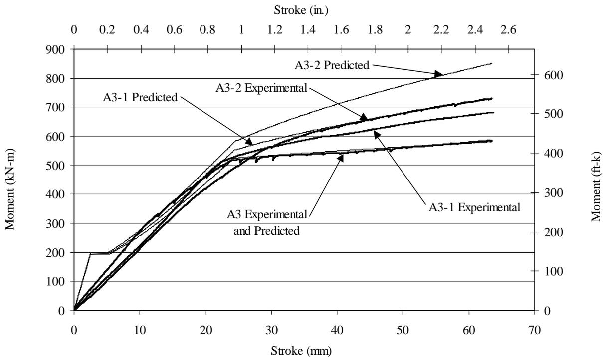
**Figure 7.** Experimental and predicted moment-stroke plots for A3 T beams.
