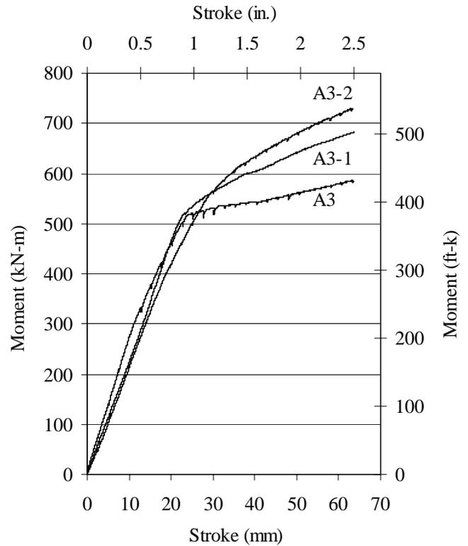
**Figure 4.** Moment-stroke curves for beams A3, A3-1, and A3-2.
