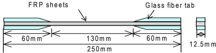
**Figure 2.** Details of Tensile Specimens
