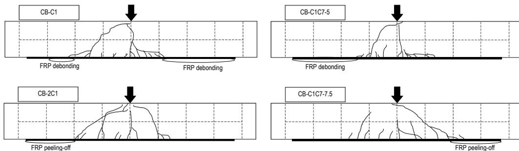
**Figure 11.** Cracking and Debonding Patterns of Specimens
