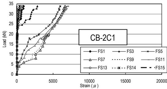
**Figure 13.** Load-FRP Strain Relations of CB-2C1
