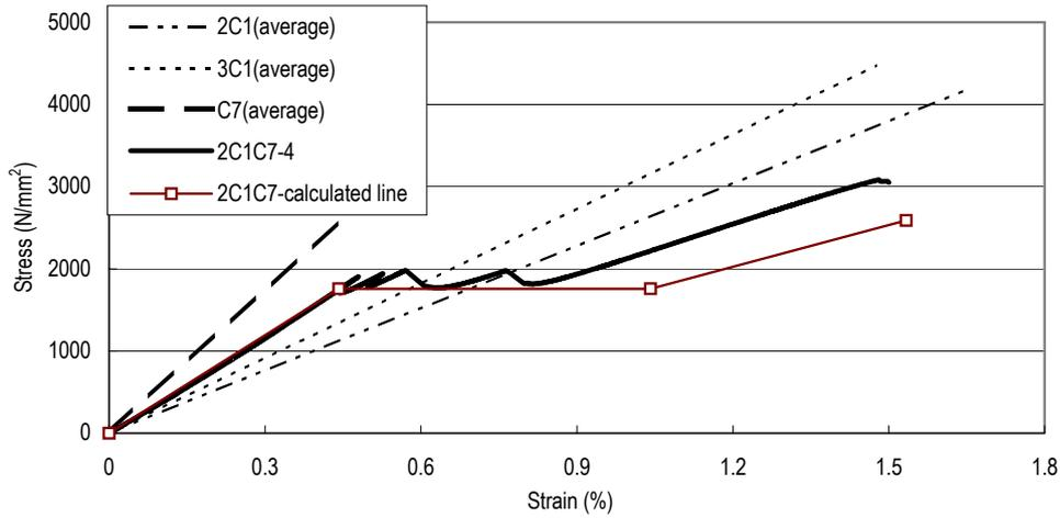
**Figure 7.** Comparison of Stress-Strain Relationships
