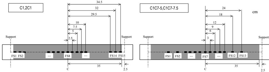
**Figure 10.** Arrangement of FRP Stain Gauges
