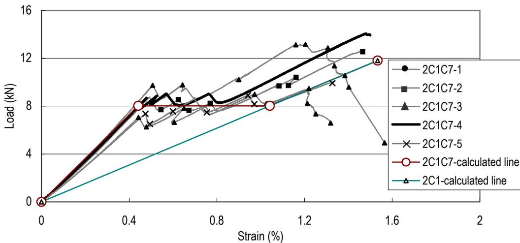
**Figure 6.** Load-Strain Relationships (2C1C7 Hybrid)
