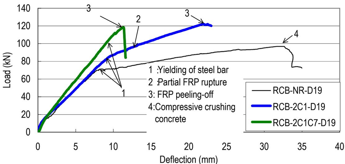
**Figure 18.** Load-Deflection Relations (Type A Specimens)
