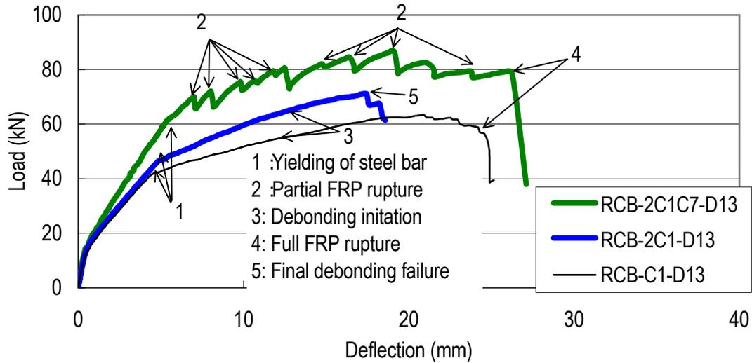
**Figure 19.** Load-Deflection Relations (Type B Specimens)
