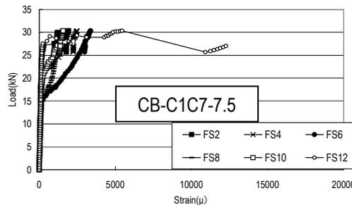
**Figure 15.** Load-FRP Strain Relations of CB-C1C7-7.5
