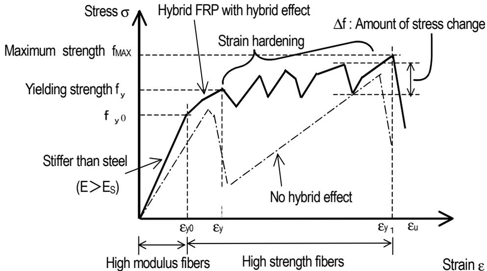
**Figure 1.** Idealized Stress-Strains Relation of Hybrid FRP Sheets Consisting of Two Types of Fiber Sheets
