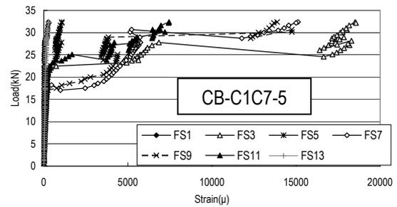
**Figure 14.** Load-FRP Strain Relations of CB-C1C7-5
