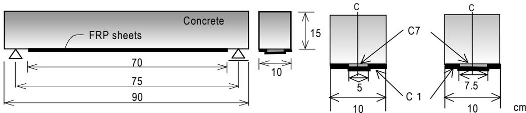
**Figure 8.** Details of Beam Specimen
