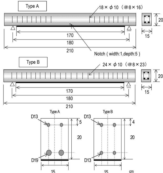
**Figure 16.** Details of Beam Specimens
