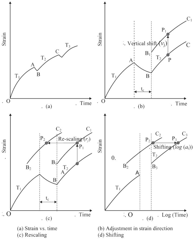
Figure 1 – SIM procedure in schematic diagrams
