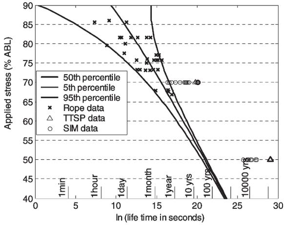
Figure 8 – Comparison of stress rupture data at 50 and 70% ABL
