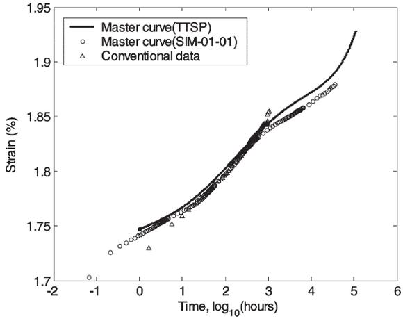
Figure 6 – Master curves with conventional creep data at 70% ABL
