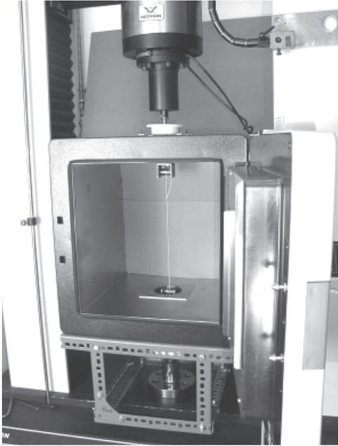
Figure 2 – Experimental set-up for tensile, TTSP and SIM test
