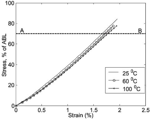
Figure 3 – Stress vs. strain curves at different temperature
