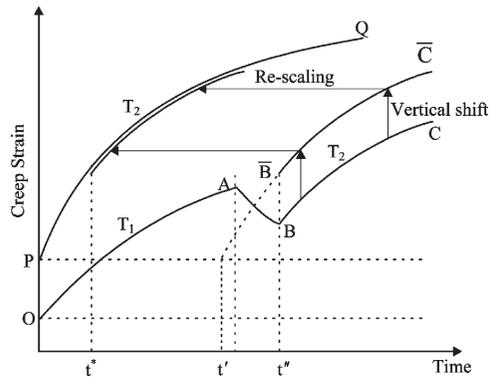
Figure 5 – Rescaling procedure for SIM
