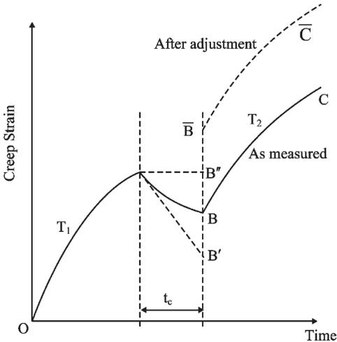
Figure 4 – Change of creep behaviour at a temperature step
