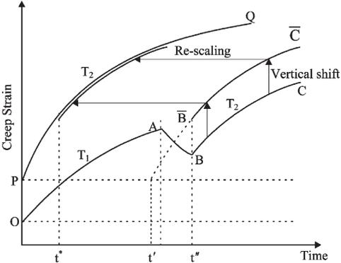
Figure 5 – Rescaling procedure for SIM
