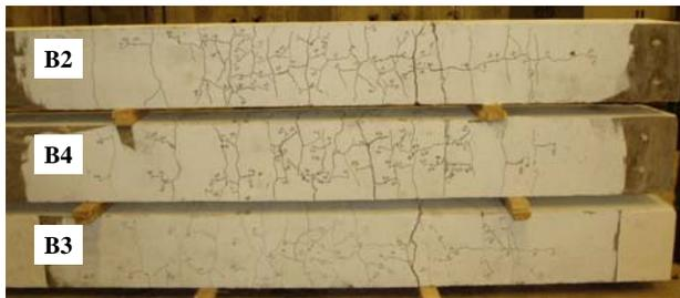
Figure 6 Lap Splice Failure - Crack Pattern
