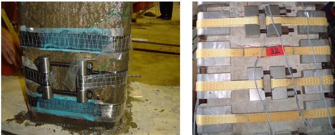
Figure 1. Pre-tensioning technique for carbon (left) and aramid FRP belts (right).
