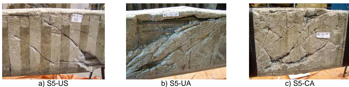
Fig. 3 Specimens after failure with FRP removed.
