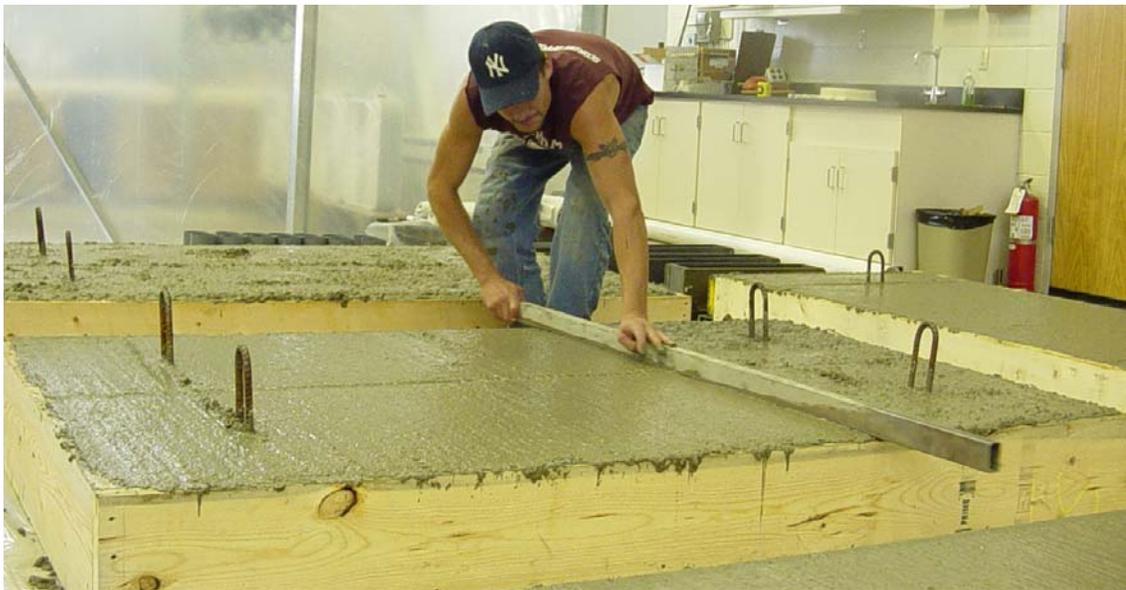
Figure 3.9. Specimen Leveling of Fresh Concrete
