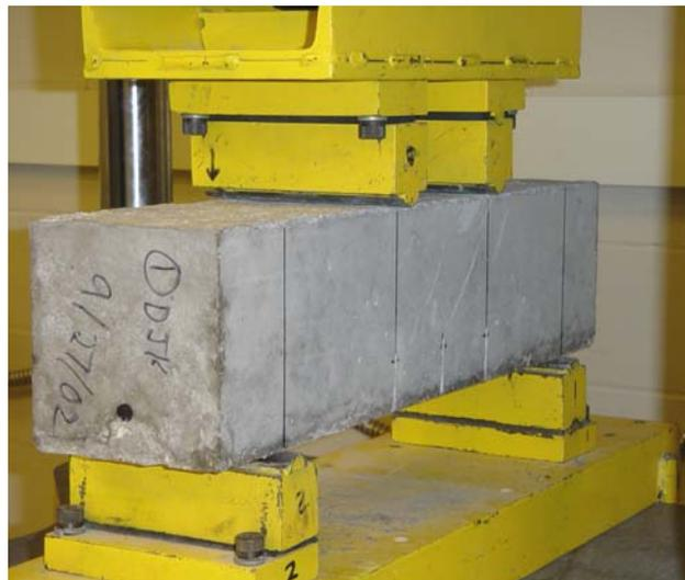
Figure 4.3. Third-Point Loading of Flexural Beam
