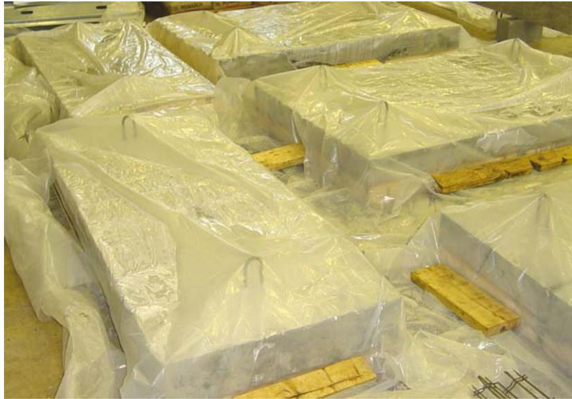
Figure 3.10. Phase III Concrete Curing
