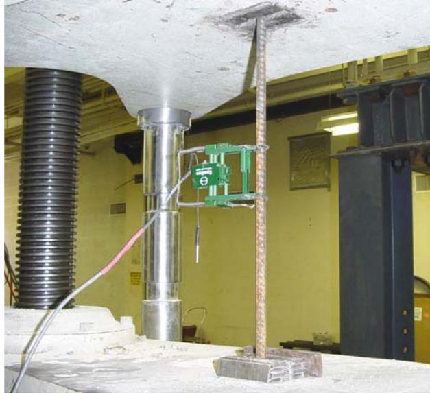
Figure 4.4. Steel Rebar Tensile Coupon Test
