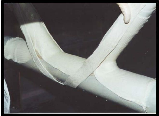
Fig. 2. Support frame and test configuration Fig. 3. Application of unidirectional GFRP tendons
