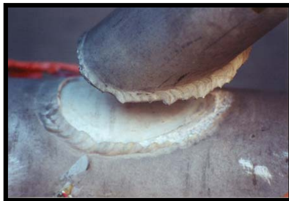
Fig. 8. Close-up of weld failure of specimen TS3
