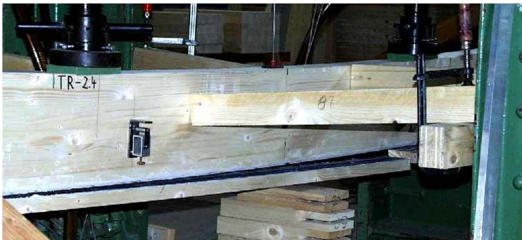
**Figure 4:** Delamination of the timber facing of specimen Tr-2.4 with CFRP and an Epoxid adhesive
