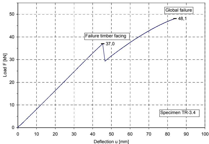
**Figure 7:** Load deflection curve of test specimen Tr-3.4
