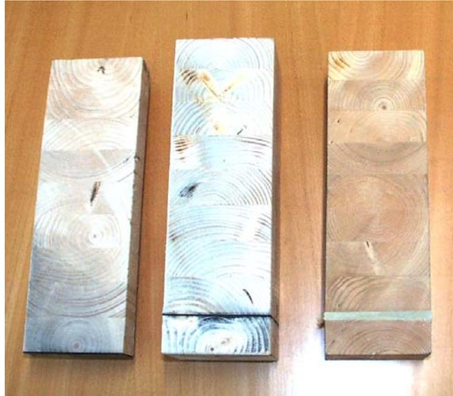
**Figure 3:** Types of cross section: CFRP without timber facing; CFRP with timber facing; AFRP with timber facing
