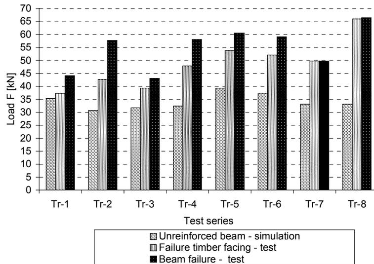
**Figure 6:** Mean values of the ultimate load for first and global failure
