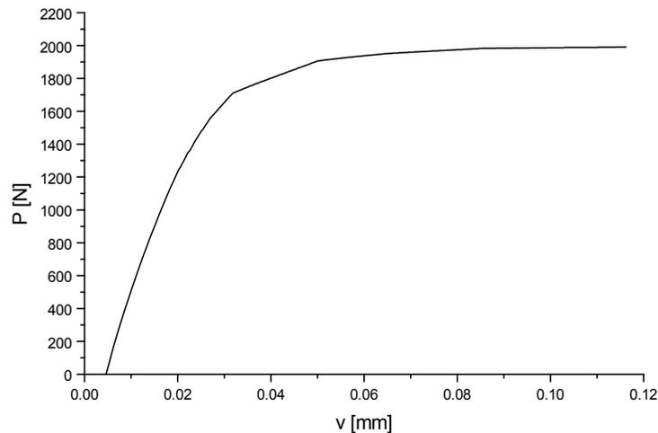
**Figure 8.** Mechanical response of the unreinforced arch.
