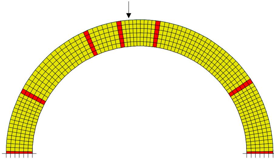
**Figure 6.** Arch discretization: geometry and constraints.
