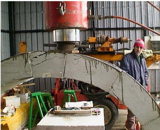
**Figure 3.** Failure of the first reinforced arch.
