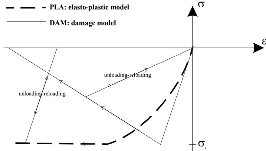
**Figure 5.** Stress-strain relations accounting for the plastic or the damage evolution.
