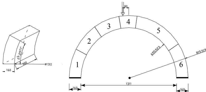
**Figure 1.** Geometry of the arch and of a single block.
