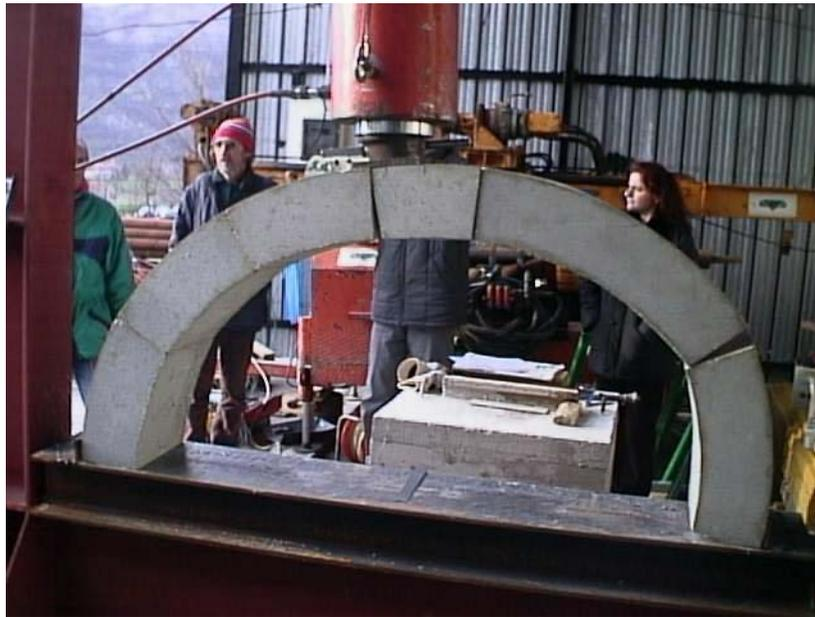
**Figure 2.** The four hinges mechanism for the unreinforced arch.
