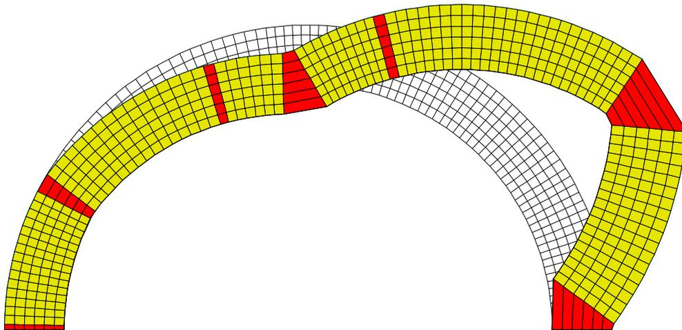
**Figure 7.** Deformation of the unreinforced arch at collapse.
