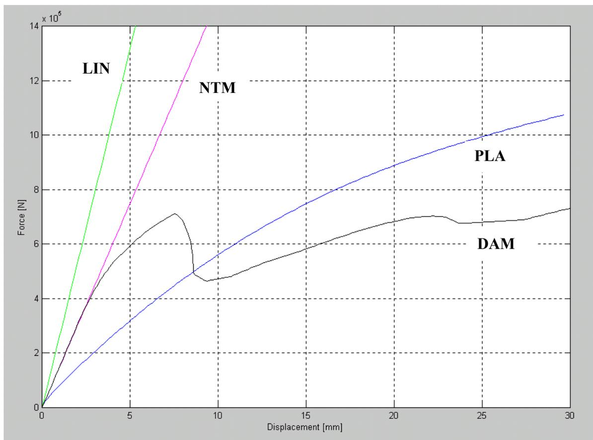
**Figure 10.** Mechanical response of the reinforced arch.
