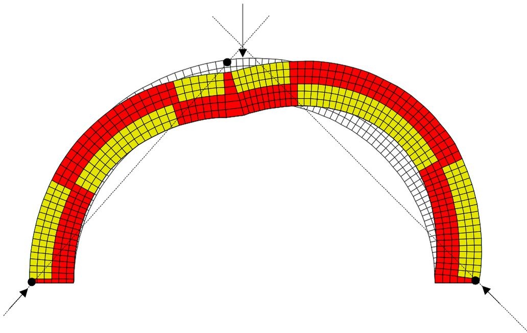
**Figure 9.** Deformed configuration of the reinforced arch.
