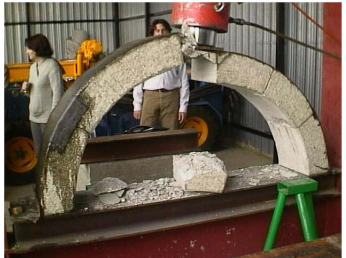
**Figure 4.** Collapse of the second reinforced arch.
