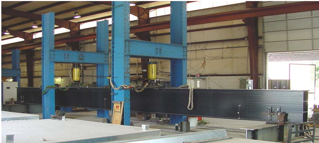
Figure 2. Long-span testing of the 36-inch DWB.
