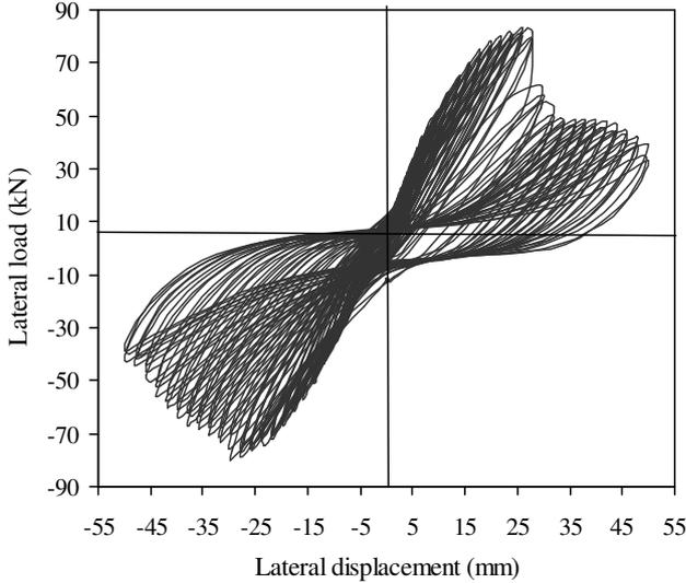
Fig. 4 Load-displacement hysteretic plot for CFRP upgraded specimen.
