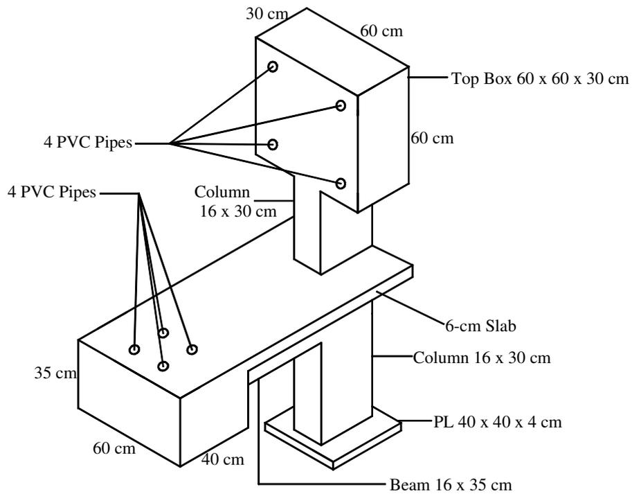
**Fig. 1** Schematic diagram of exterior joint specimen.
