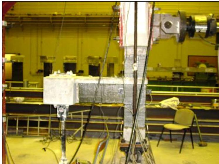
**Fig. 2** Picture showing FRP repaired specimen.
