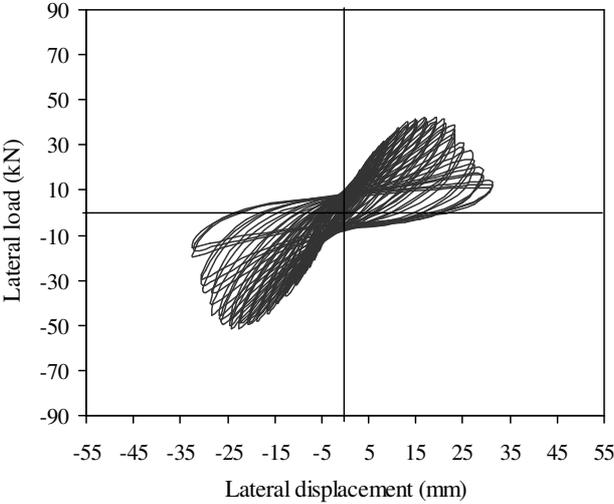
Fig. 3 Load-displacement hysteretic plot for control specimen.
