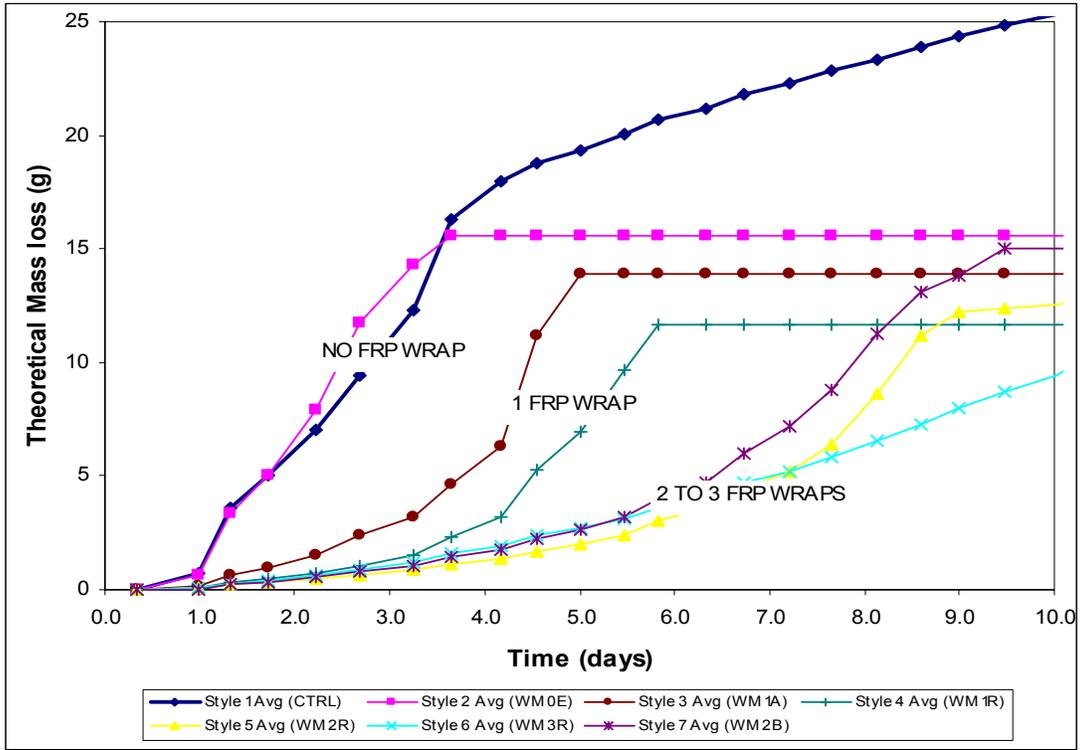
Figure 4. Mass Loss Averages vs. Time – WM Epoxy (10 Days)
