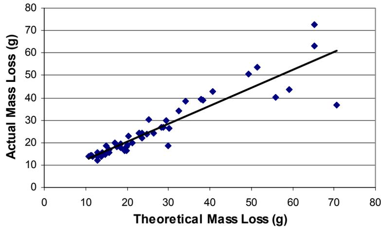
**Figure 2.** Total Mass Loss – Theoretical vs. Actual
