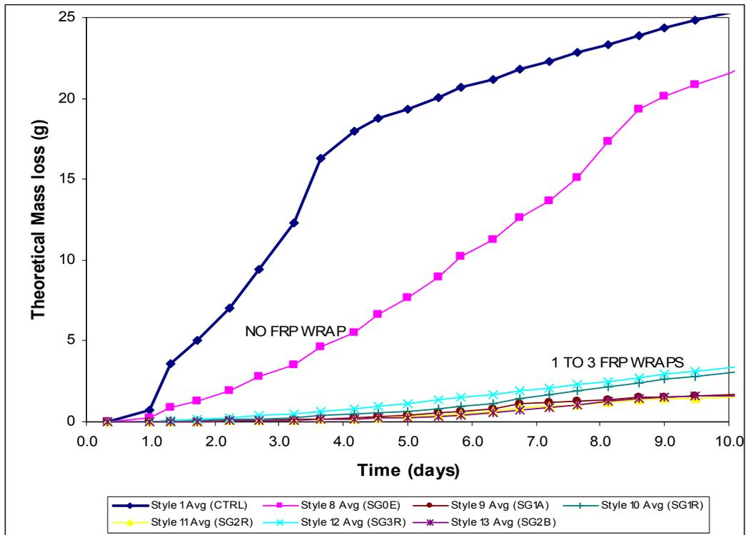
Figure 5. Mass Loss Averages vs. Time – SG Epoxy (10 Days)
