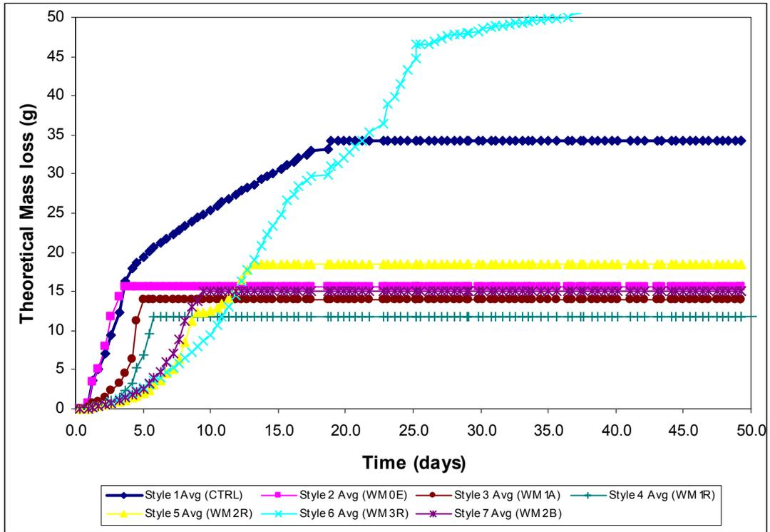
**Figure 6.** Mass Loss Averages vs. Time – WM Epoxy (50 Days)
