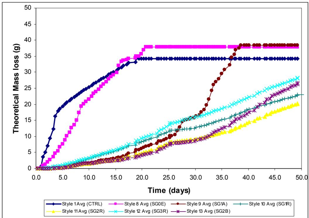
**Figure 7.** Mass Loss Averages vs. Time – SG Epoxy (50 Days)
