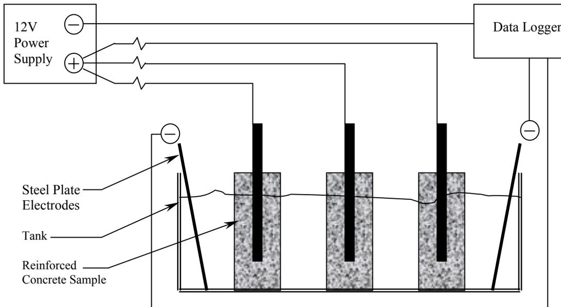
**Figure 1.** Test Configuration Schematic
