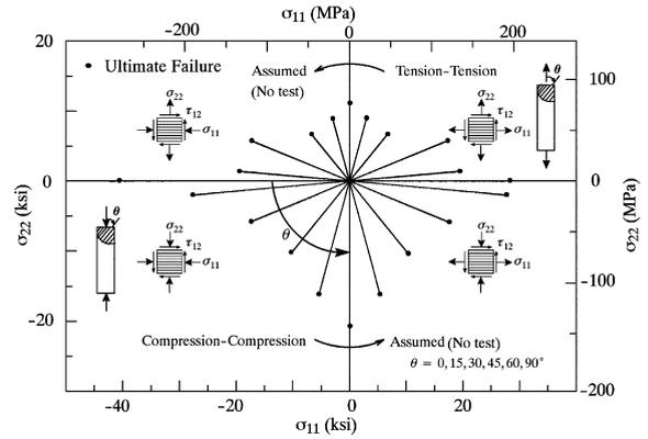
Fig. 4. Axial and transverse stress paths ( $\sigma_{11}$  and  $\sigma_{22}$ ).
