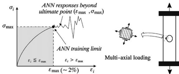
Fig. 14. Schematic drawing of the ANN response out of range of the training data.
