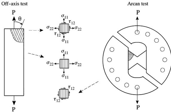
Fig. 3. Off-axis and Arcan bi-axial coupon tests performed to generate multi-axial stress–strain data needed for the ANN training.
