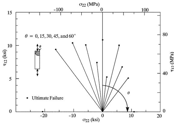
Fig. 6. Transverse and shear stress paths ( $\sigma_{22}$  and  $\tau_{12}$ ) from off-axis tests. The pure shear case was obtained from the modified Arcan test.
