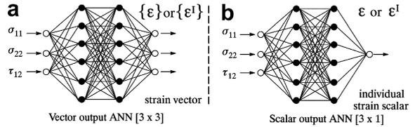
Fig. 2. Schematic drawing of two ANN general models using total and/or inelastic strain. The second approach in (b) is to generate ANNs for each individual output variable.
