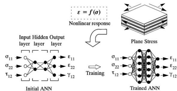
Fig. 1. Schematic drawing of a typical feed-forward 4-layer ANN structure for plane-stress nonlinear material models.
