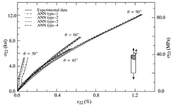
Fig. 7. ANN representation of transverse stress–strain in the local material direction after training.
