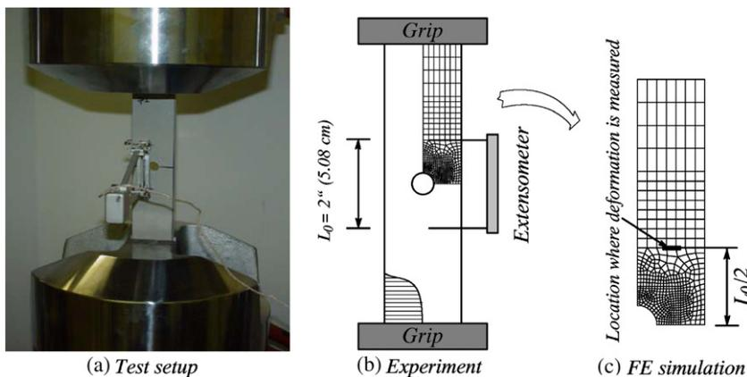
Fig. 11. Schematic drawing of the experiment and FE simulation used in the verification.
