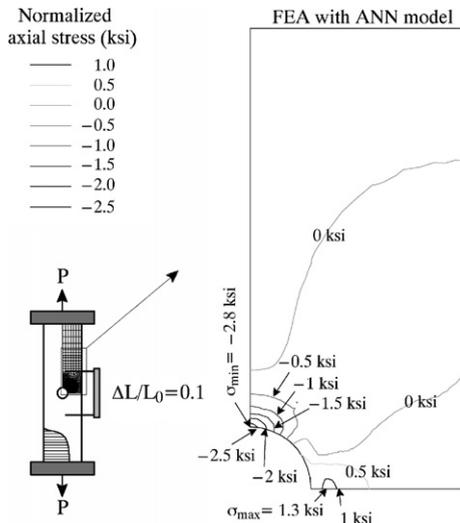
Fig. 13. Normalized axial stress contours generated from the proposed ANN material model.
