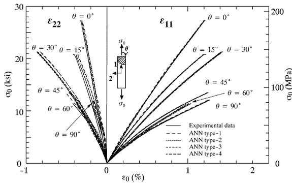
Fig. 8. Global tension stress versus direct and Poisson's strains calculated from the local response of the trained ANNs.
