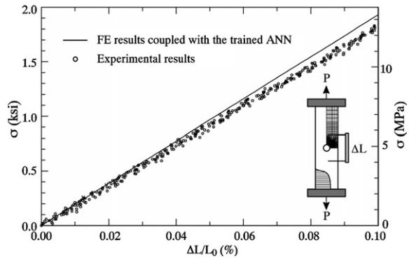
Fig. 12. Prediction for the remote stress–strain curves obtained from experiments and FE simulations implemented with the proposed ANN material model.
