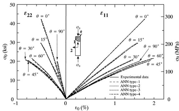
Fig. 9. Global compression stress versus direct and Poisson's strains calculated from the local response of the trained ANNs.
