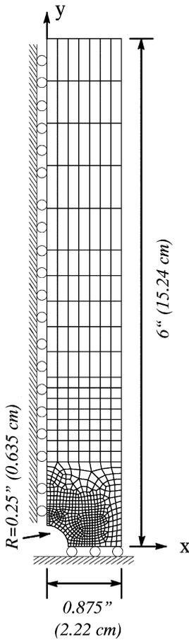
Fig. 10. Geometry of the quarter FE model with hole.
