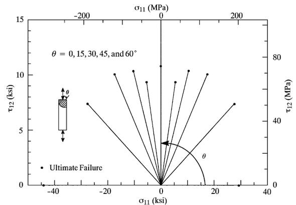
Fig. 5. Axial and shear stress paths ( $\sigma_{11}$  and  $\tau_{12}$ ) from off-axis tests. The pure shear case was obtained from the modified Arcan test.
