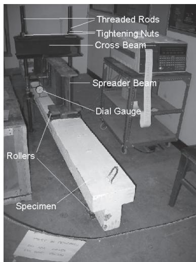
Figure 6 – Long-term beam test set-up
