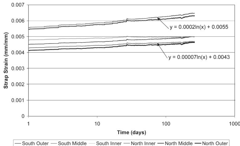
Figure 9 – Logarithmic plot of strap strain vs. time
