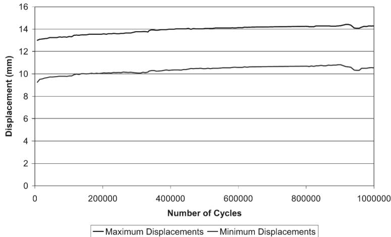
Figure 13 – Mid-span deflection vs. number of cycles
