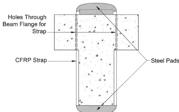
Figure 2 – CFRP strap configuration used in Kesse, Chan and Lees
