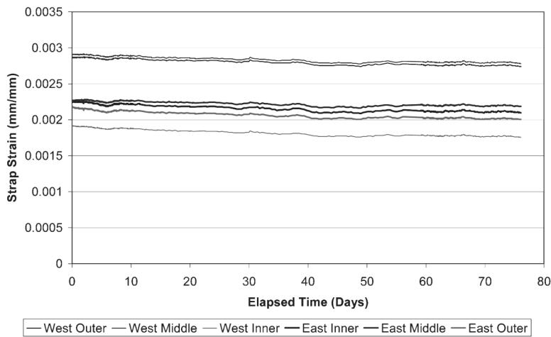
Figure 7 – Long-term CFRP strap strain vs. time under no applied load
