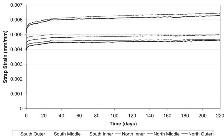
Figure 8 – Long-term CFRP strap strain vs. time under applied load
