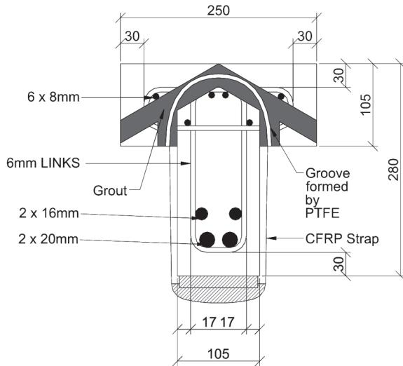
Figure 3 – Beam cross-section
