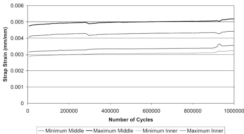
Figure 14 – Strap strains vs. number of cycles
