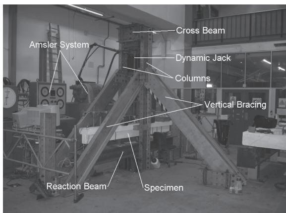
Figure 12 – Self-reacting frame for cyclic test
