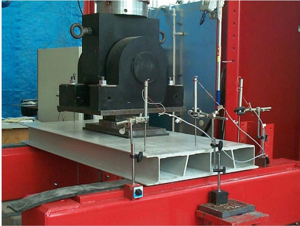
**Figure 7.** Static 3-Point Bending Test at CFL (NCSU) for the 5” Deck Profile; May 2001.
