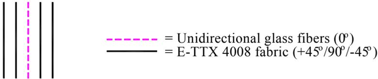
**Figure 3.** Schematic of Ply Lay-Up in Web Section of DuraSpan 500 Deck.
