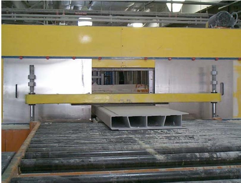
**Figure 5.** Five-Inch Deck Profile Being Pultruded at Creative Pultrusions, Inc.; May 2001.
