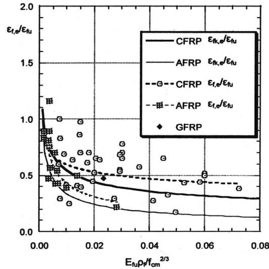
**Figure 3** Nominal FRP Strain Limit in fib Code
