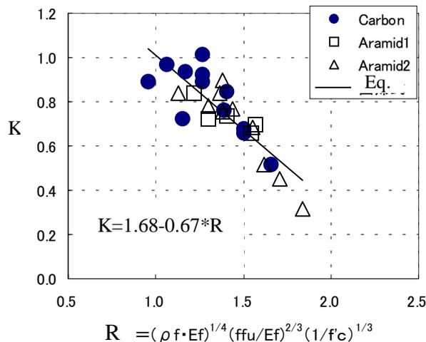
**Figure 2** Relationship between K and R in JSCE Code
