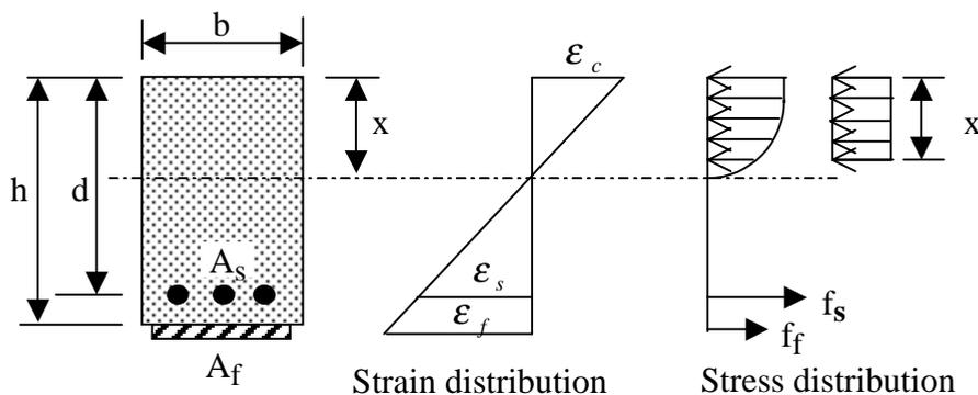
**Figure 1.** Analysis of cross section for flexure
