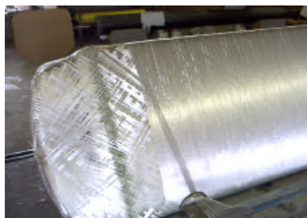
Figure 2. Filament Winding of Entire Module
