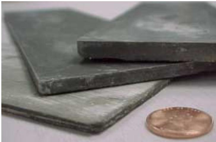
Figure 1:Thin cement plate reinforced with unidirectional fiber tapes (thickness=2, 3, 4 mm, from bottom to top).
