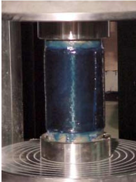
Figure 2: Concrete confined with CFRP composite jacket.
