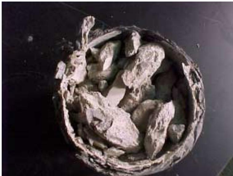
Figure 7: Concrete inside the CFRC jacket was crushed completely after global failure.
