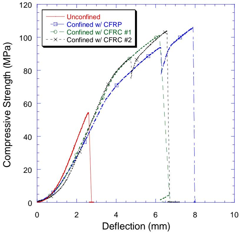
Figure 4: Compressive behavior of unconfined and confined concrete.
