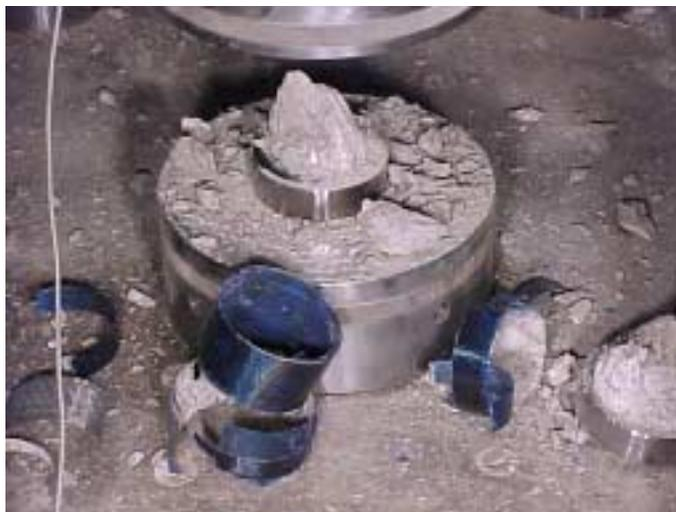
Figure 5: Remnants of CFRP sample after violent failure.
