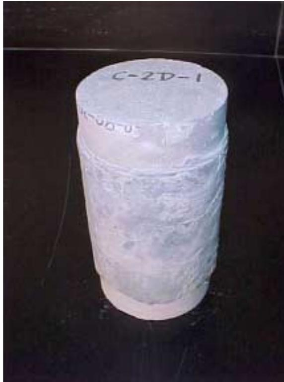
Figure 3: Concrete confined with CFRC composite jacket.
