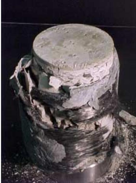
Figure 6: Global failure of the CFRC sample due to rupture of the CFRC jacket.
