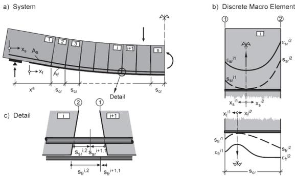
Figure 3 – Numerical model for strengthened flexural members
