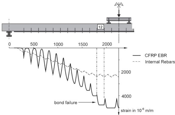
Figure 5 – Calculated reinforcement strains prior to bond failure (last convergent increment) (slab No. B2-o8-B2C)
