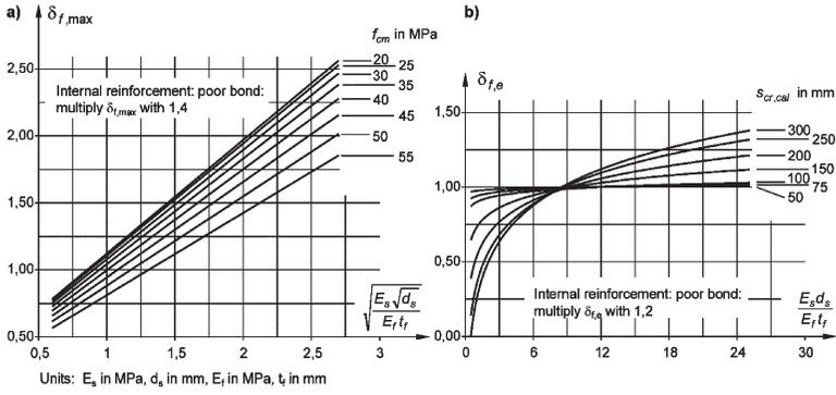
Figure 8 – Bond coefficients for CFRP-laminates combined with ribbed reinforcing bars
