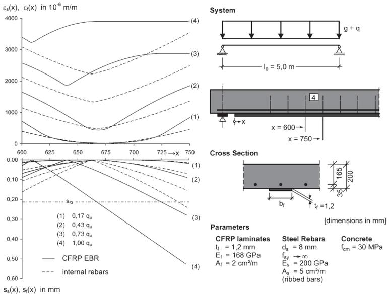
Figure 6 – Reinforcement strains and related slip in element No. 4 for 4 different load steps
