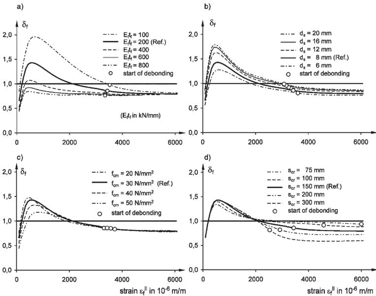
Figure 7 – Development of strain ratio  $d_f$  at midspan with increasing load, parameters affecting the distribution of cross sectional forces (Reference system acc. to Fig. 6)
