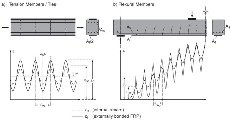
Figure 2 – Influence of bond on tensile strains in the different reinforcement layers
