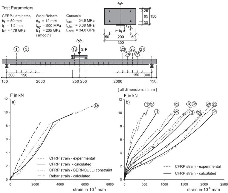
Figure 4 – Calculated reinforcement strains vs. measured strains in predefined cracks (slab No. B2-o8-B2C)
