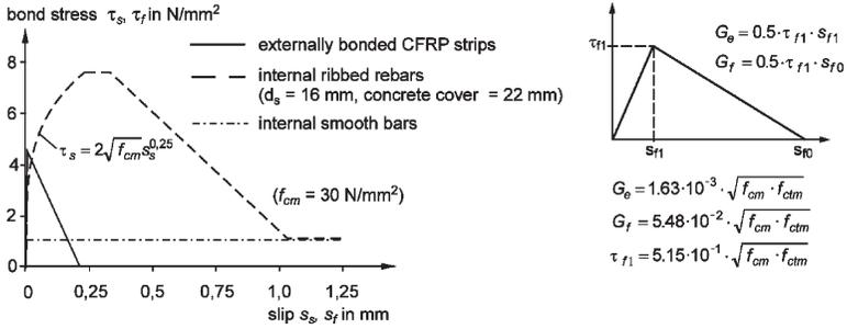
Figure 1 – Bond models for internal rebars and externally bonded reinforcement
