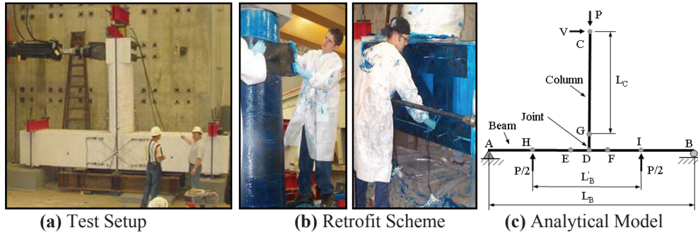
Figure 1. Test setup, retrofit scheme, and analytical model.
