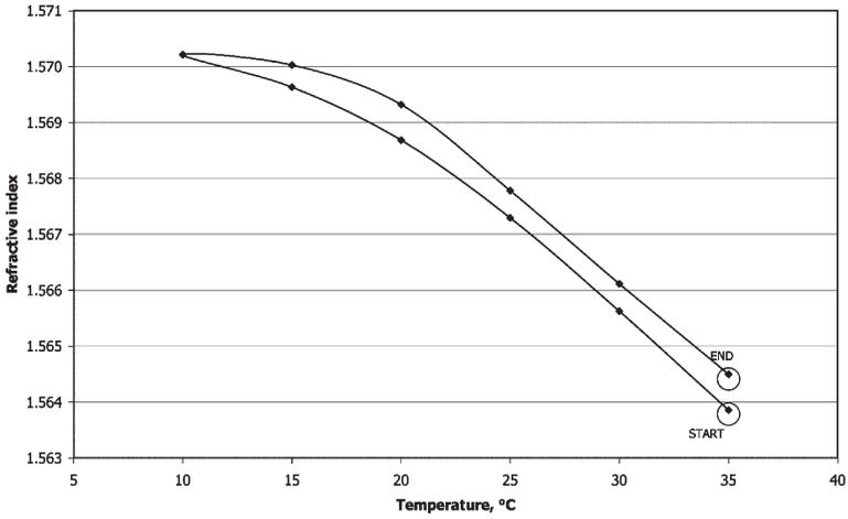
Figure 5 — Refractive index of the partial cured resin (conversion=0.7) as function of temperature during the temperature ramps in the range 10-35 °C.
