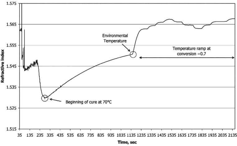
Figure 4 — Refractive index as function of time during the incomplete polymerization at 70°C and the temperature ramps.
