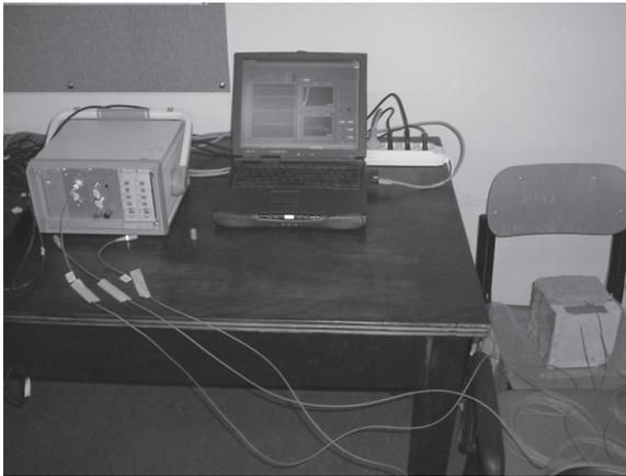
Figure 2 – Fiber optic refractometer and its in-situ application.
