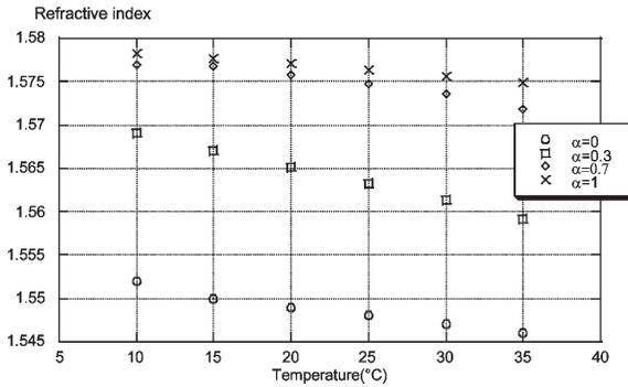
Figure 6 — Refractive index as function of temperature for different level of resin conversion.
