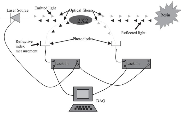
Figure 1 – Schematic of the fiber optic refractometer.
