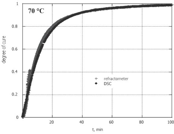
Figure 3 — Conversion evaluated by DSC test and refractive index measurements.
