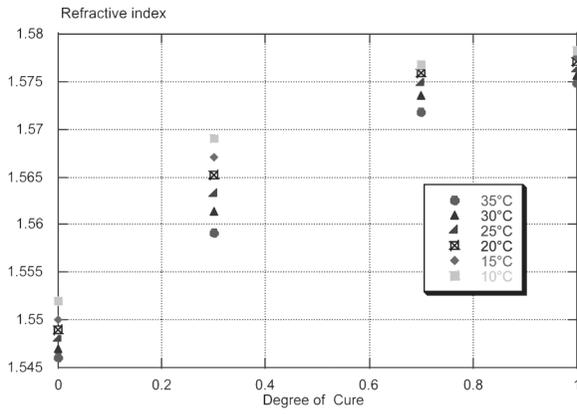
Figure 7 — Refractive index as function of cure for different temperature levels.
