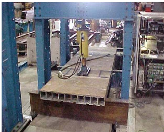
(a) Test configuration using steel patch
