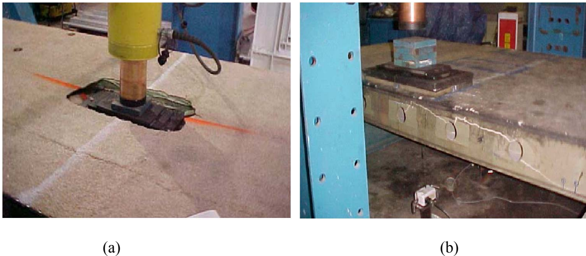
Figure 6. Failure of Deck A using steel loading patch [7]
