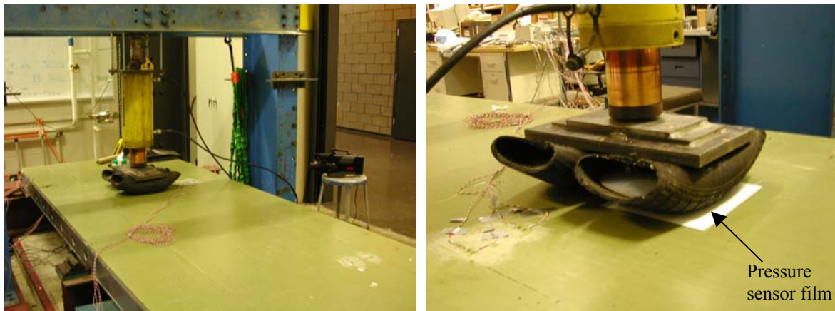
Figure 3. Test configuration using the patch made of real tire stuffed with silicon rubber
