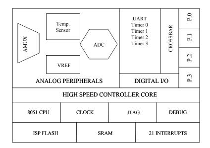
Figure 6-5 C8051 Block Diagram
