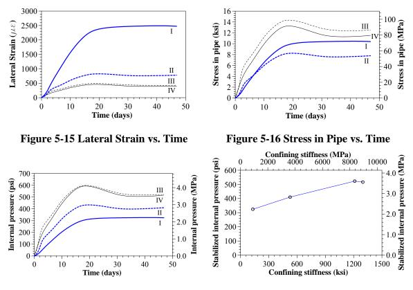
**Figure 5-17 Internal Pressure vs. Time**
