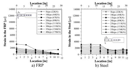
Figure 3-30 Strain Profiles – Specimen C-2
