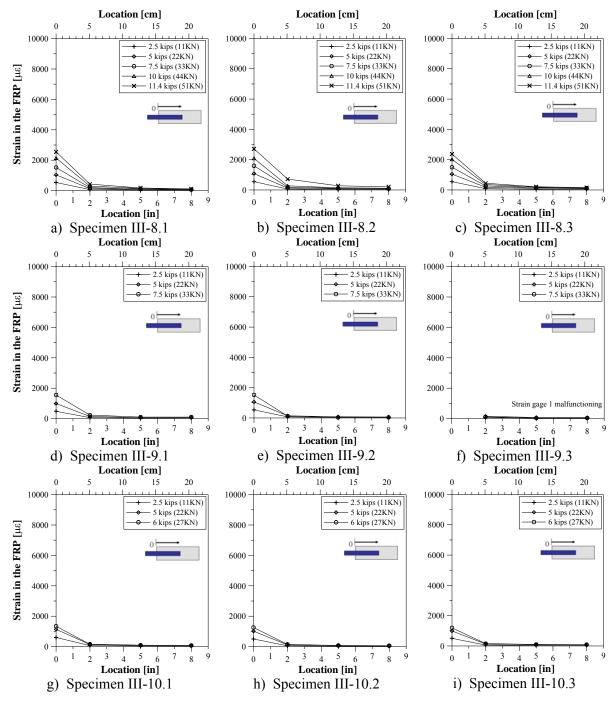
Figure 3-23 Strain Profiles – Specimen III-8 to III-10
