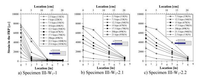
Figure 3-27 Strain Profiles – Test Series III-W1
