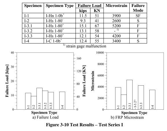
Table 3.6 Test Results – Test Series I
