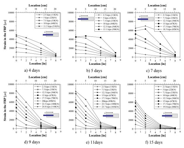
Figure 3-26 Strain Profiles – Test Series IIIT
