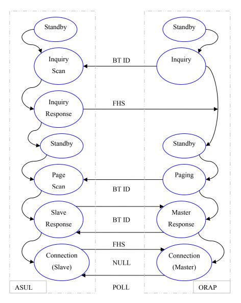
**Figure 6-7 Connection Establishment Process**
