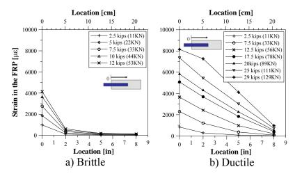
**Figure 3-31 Typical Strain Profiles**
