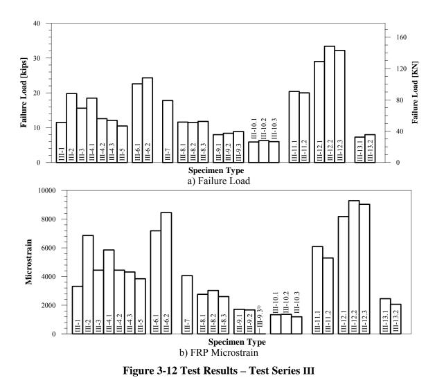
In Specimen III-2 the GC-Hybrid FRP laminate was sanded prior to the application. But beads of 80mils (2mm) diameter were used to control the adhesive thickness. Post-test inspection indicated that the epoxy was properly cured. This specimen experienced a failure at the interface between the steel and the epoxy (see Figure 3-6c), and was described as exhibiting Failure Mode S.
