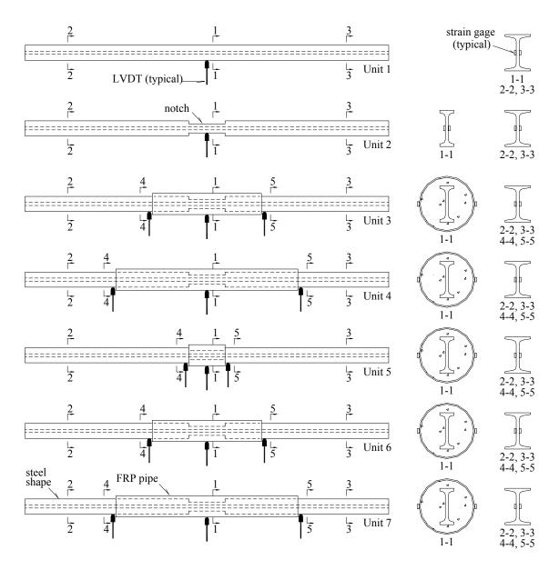
Figure 5-29 Distributions of LVDTs and Strain Gages
