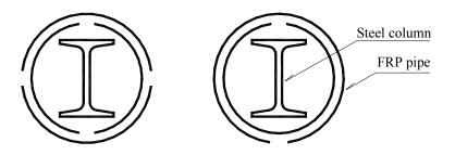
**Figure 5-26 Fabrication Schemes of FRP Jackets**
