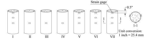
Figure 5-3 Strain Gages on Specimens of the Seven Groups
