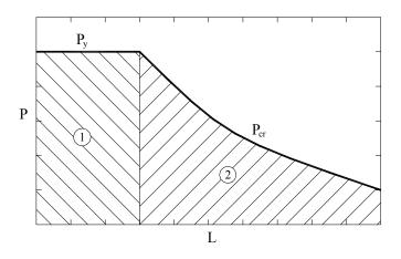
Figure 5-37 Ultimate Load (P) vs. Slenderness Parameter (L) for a Steel Column
