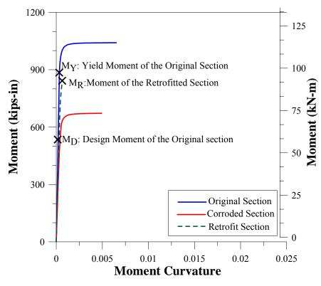
Figure 4-2 Moment Curvature Analysis for W12 x 14 Section
