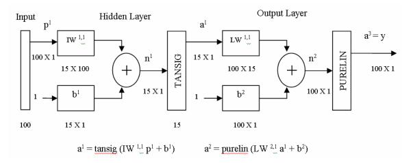
Figure 7-12 Backpropagation Architecture
