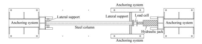
Figure 5-28 Test Setup
