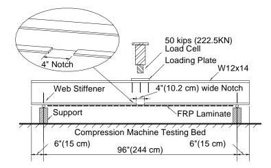
Figure 4-4 Test Setup (Liu, 2002)
