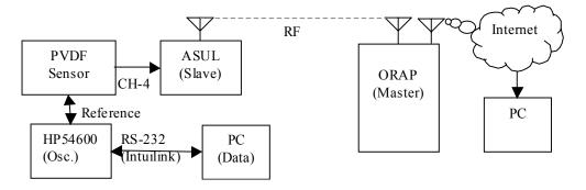
Figure 6-18 ASUL Test Configuration
