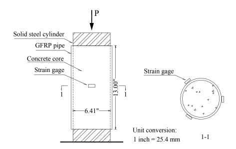
**Figure 5-11 Instrumentation of the Compression Test**
