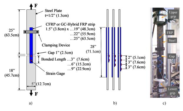
**Figure 3-1 Discontinuous Specimen**
