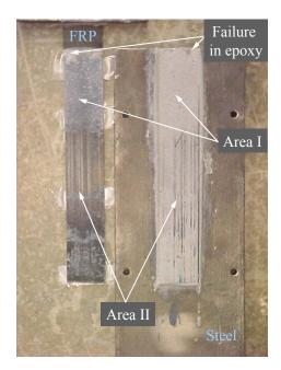
Figure 3-13 Failure of CFRP 200/2000 -Sikadur<sup>®</sup> 30 Specimens
