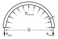
**Figure 5-4 Force Balance Mechanism**
