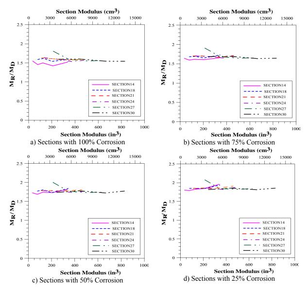
Figure 4-3  $M_R/M_D$  for Different Levels of Corrosion vs. Section Modulus
