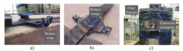
Figure 3-9 Failure of Wraps (+w)
