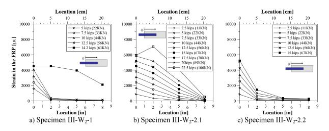
Figure 3-28 Strain Profiles – Test Series III-W2
