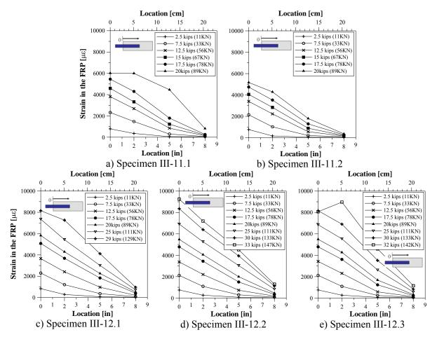
Figure 3-24 Strain Profiles – Specimen III-11 to III-12
