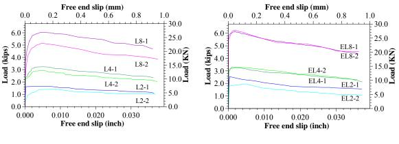
Figure 5-21 Load vs. Free End Slip of Group I
