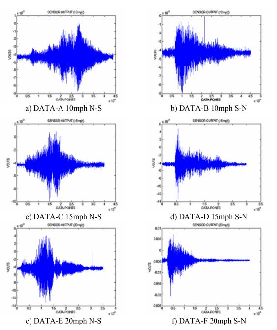
sensor specifications and is converted to +/- 2.4 volts. Figure 7-7 shows the data values in volts after the calibration process was completed.
