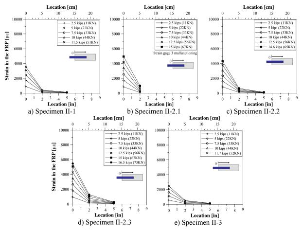
Figure 3-20 Strain Profiles – Test Series II
