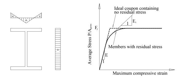
Figure 5-35 Influence of Residual Stress on Average Stress-strain Curve
