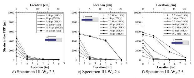
Figure 3-28 Strain Profiles – Test Series III-W<sub>2</sub> (Continuation)
