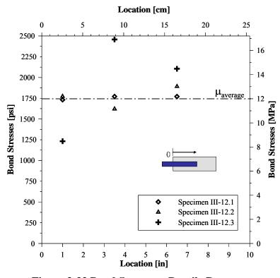
Figure 3-33 Bond Stresses – Ductile Response
