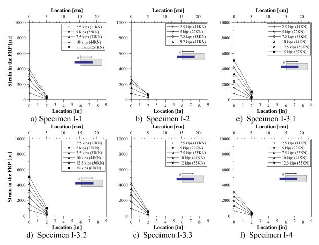
Figure 3-19 Strain Profiles – Test Series I
