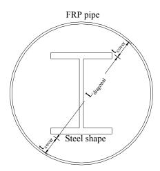
**Figure 5-38 Structural construction requirement for the retrofitted material**
