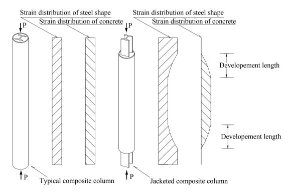
Figure 5-32 Load Transfer Mechanisms of Typical Composite Column and Jacketed Composite Column
