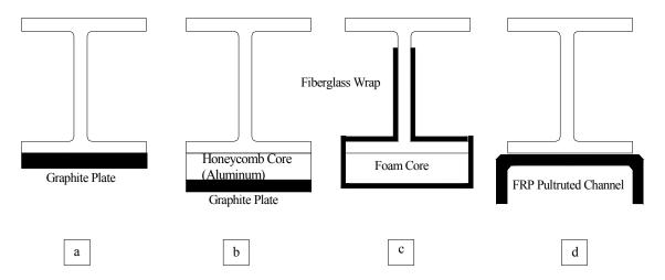
Figure 2-4 Reinforcement Schemes (Gillespie et al, 1996)
