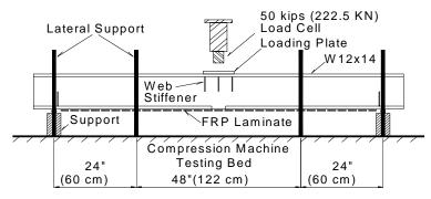
Figure 4-6 Lateral Support Setup (Liu, 2002)
