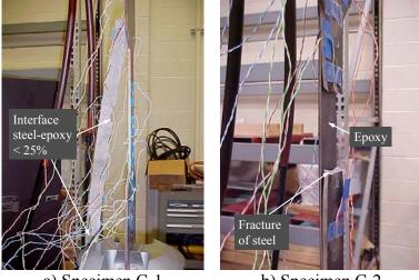
a) Specimen C-1b) Specimen C-2Figure 3-18 Failure of Continuous Specimen
