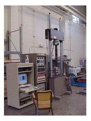
strain gage channels of the machine and **Figure 3-5 MTS 880 and Data Acquisition** balanced to zero. (6) The steel angles, holding the steel plates together, were removed. (7) To
