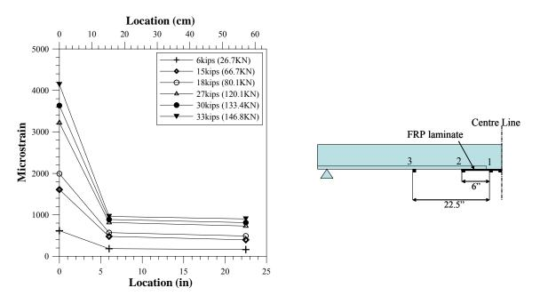
Figure 4-18 Strain-Location – Test Unit 4
