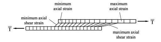
Figure 2-1 Deformations for Rigid – Deformable Joint
