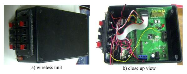
Figure 6-9 Smart Sensor Cluster
