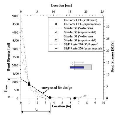
Figure 3-32 Bond Stresses – Brittle Response
