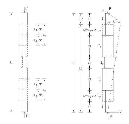
Figure 5-34 Assumed Stiffness Distribution and Deflection Shape for Test Unit 3 to 7
