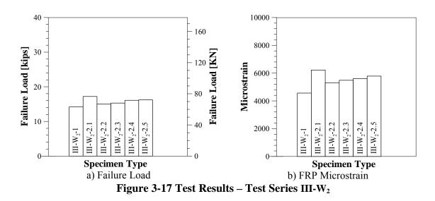
As indicated in Table 3.11, in Specimen III- $W_2$ -1 the GC-Hybrid FRP laminate was not sanded prior to the application. No beads were used to obtain a constant adhesive thickness. The epoxy had cured sufficiently at the time of the test. This specimen experienced a failure at the interface between the FRP and the epoxy, and the failure mode is therefore characterized as Failure Mode F (see Figure 3-8c).
