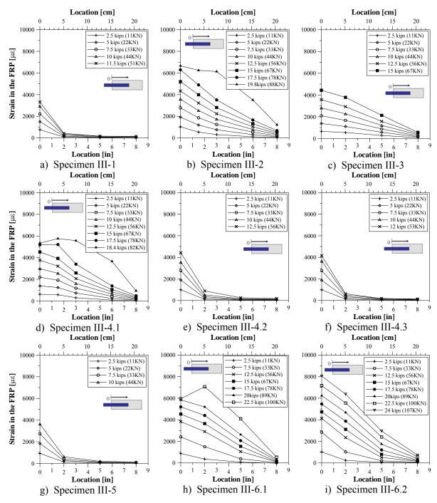
Figure 3-21 Strain Profiles – Specimen III-1 to III-6
