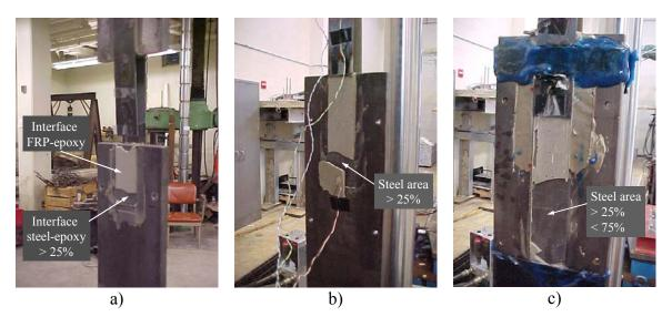
Figure 3-7 Failure Mode SF
