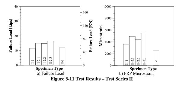
Specimen II-3 was the only specimen fabricated with the CFRP 200/2000. Glass beads of a diameter of 80mils (2mm) were used to obtain a constant adhesive thickness. Post-test inspection indicated that the epoxy was properly cured. This specimen experienced failure at the interface between the FRP and the epoxy (Failure Mode F, see Figure 3-8b). Carbon fibers remained on the epoxy.
