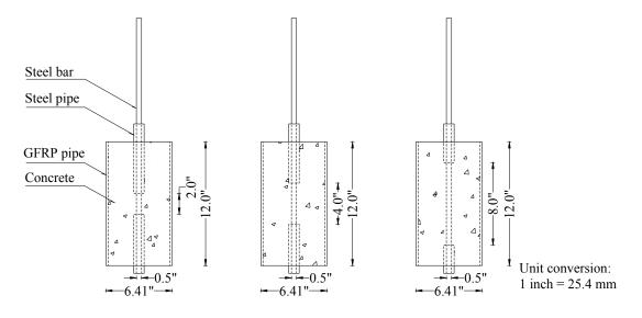
**Figure 5-19 Test Specimens**
