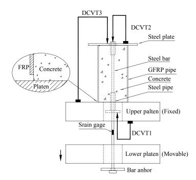
**Figure 5-20 Test Setup and Instrumentations**
