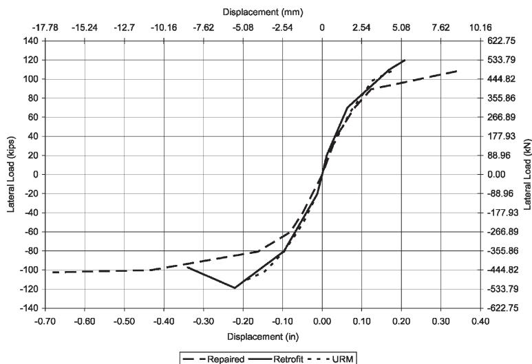
Figure 8 – Backbone curves for unreinforced, repaired and retrofitted symmetric brick structures.
