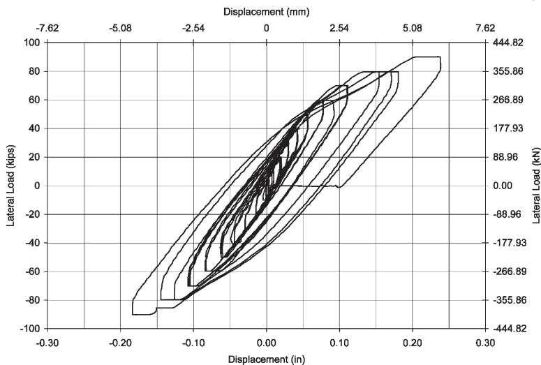
Figure 2 – Hysteretic curve for the unreinforced, symmetric CMU structure.
