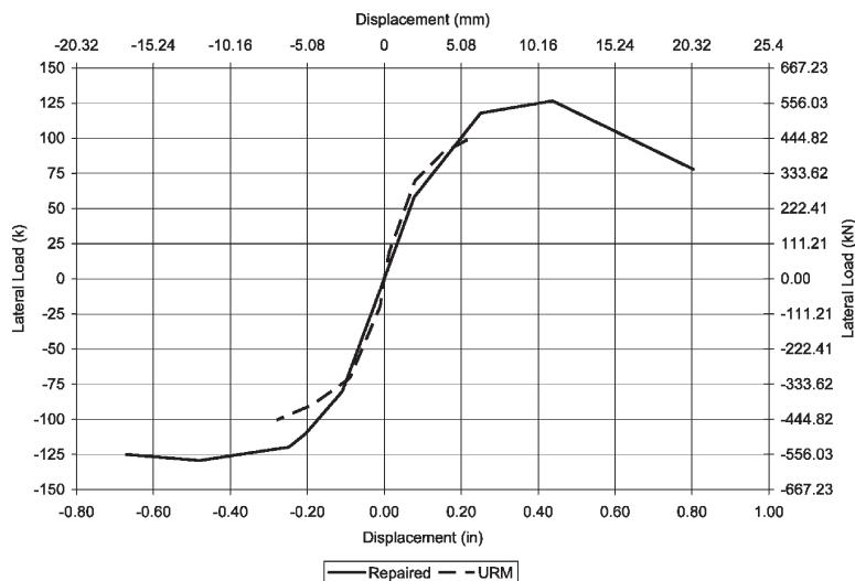
Figure 11 – Backbone curve comparison for asymmetric CMU structure in unreinforced and repaired condition.
