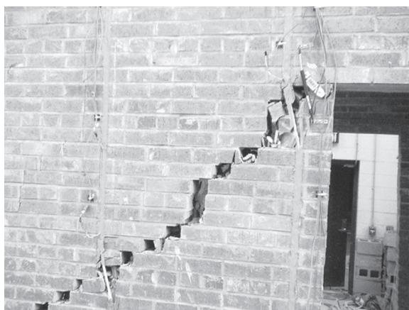
Figure 9 – Diagonal tension failure and GFRP NSM rod rupture of the symmetric retrofitted brick structure.
