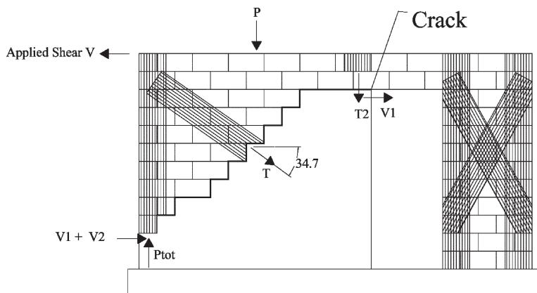
Figure 3 – Free body diagram from determination of composite layout using a strut and tie configuration.
