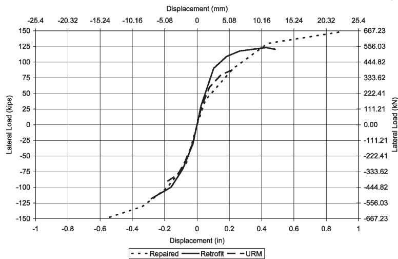
Figure 6 – Idealized backbone curve for the unreinforced, repaired and retrofitted symmetric CMU structures.
