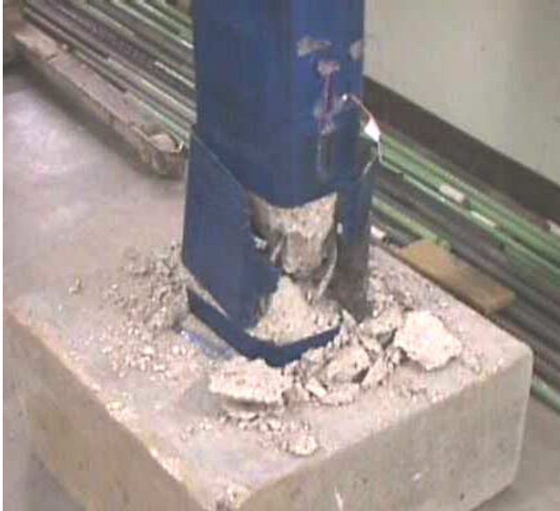
Figure 4.2. 305-mm Jacket Rupture on 2CFRP-Rect3/2-Ti178mm-p1.6
