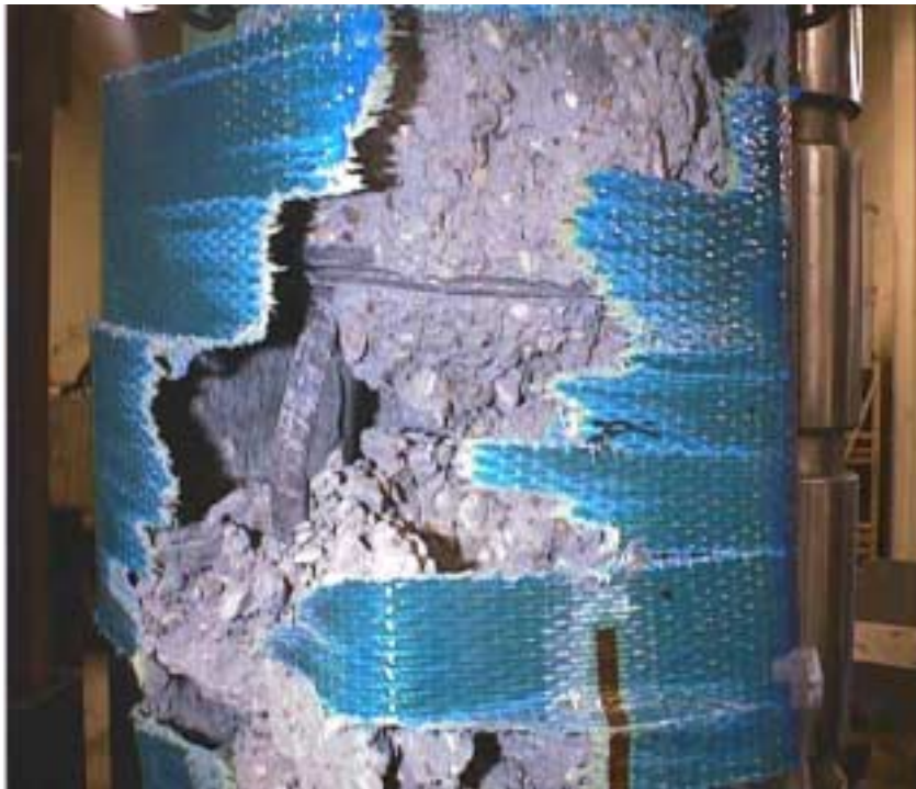
Figure 4.3. Close-up of 250-mm Jacket Rupture on 2AFRP-Rect1/1-Ti178mm-p1.6
