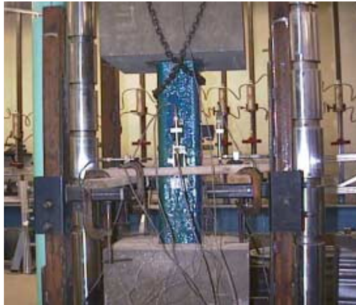
Figure 3.7. Instrumented Column in Test Frame
