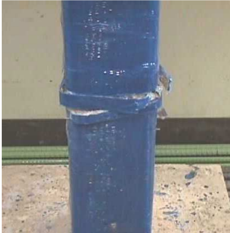
Figure 4.4. 57-mm Jacket Rupture on 2GFRP-Rect1/1-Ti178mm- \rho 1.6
