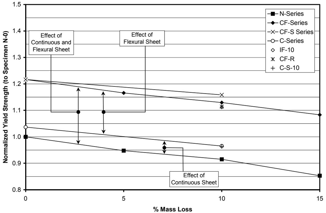
Figure 7. Small-scale specimens - normalized yield strength (to specimen N-0) vs. % mass loss
