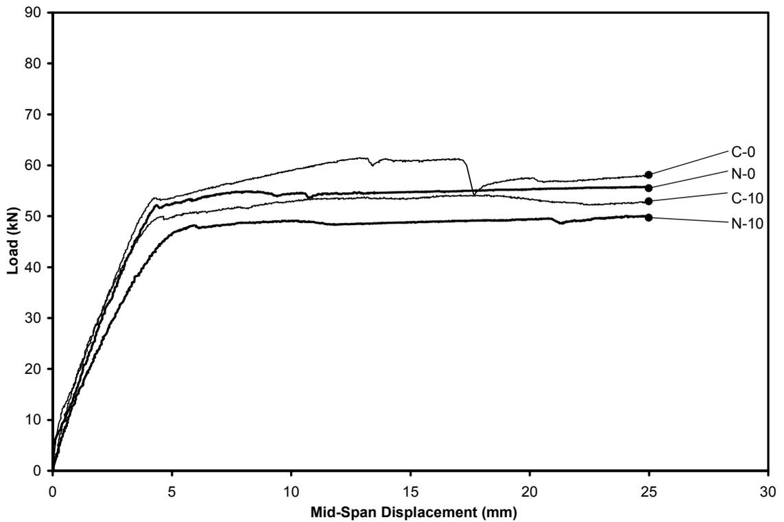
**Figure 6a.** Behaviour of small-scale CFRP strengthened RC beams at different corrosion levels
