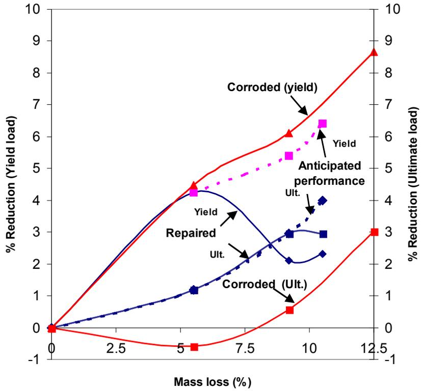
**Figure 10.** Large-scale specimens - % reduction in yield and ultimate load vs. mass loss
