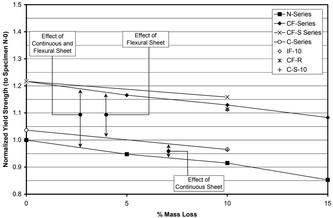
Figure 8. Small-scale specimens - normalized ultimate strength (to specimen N-0) vs. % mass loss
