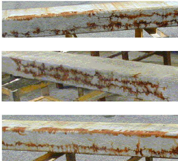
**Figure 4.** Corrosion cracking pattern in large-scale specimens
