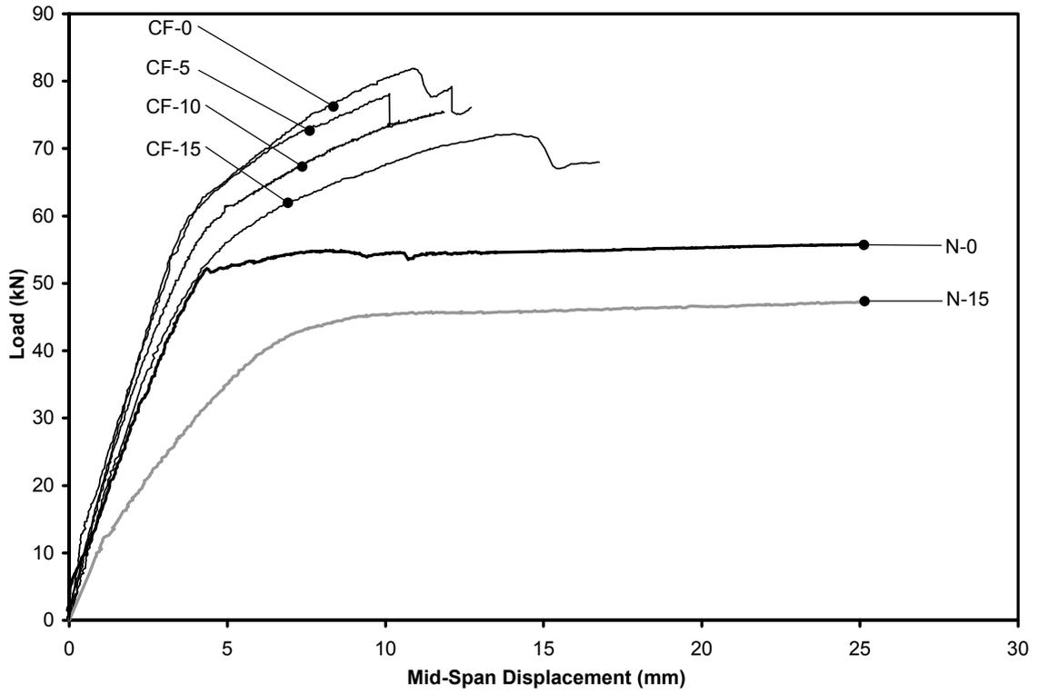
Figure 6b. Behaviour of small-scale CFRP strengthened RC beams at different corrosion levels
