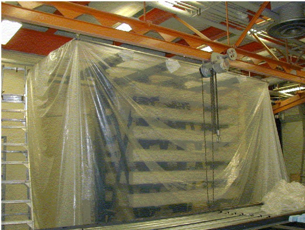
**Figure 2.** Specimens in the corrosion chamber
