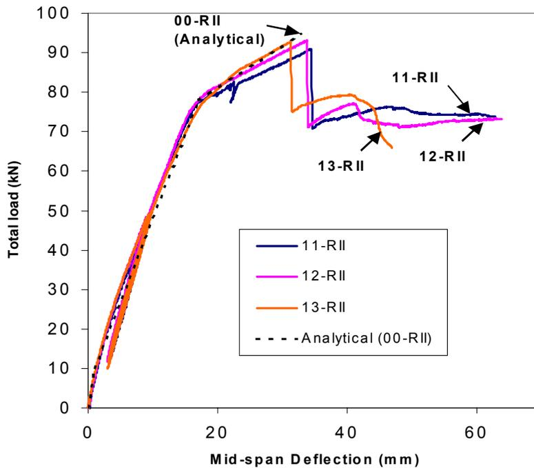
Figure 9. Behaviour of large-scale specimens repaired with GFRP U-wraps and CFRP flexural sheets
