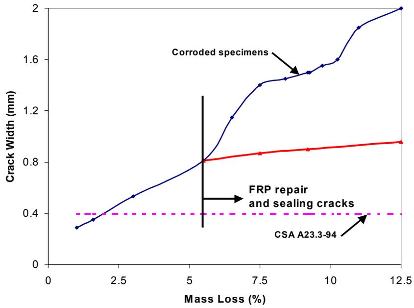
**Figure 5.** Crack width vs. mass loss
