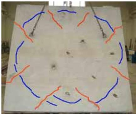
a) Top cracks in solid slab
