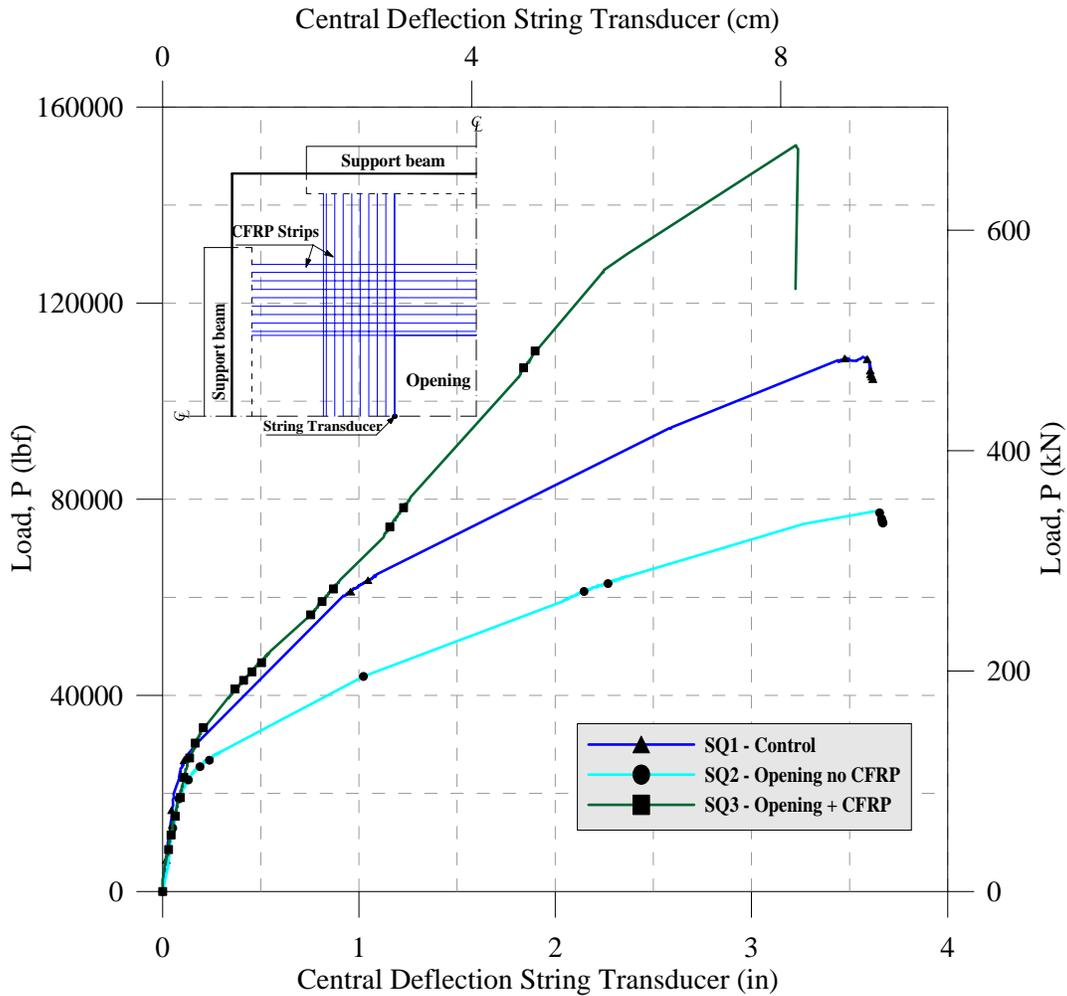
Figure 5 - Load vs Deflection curves
