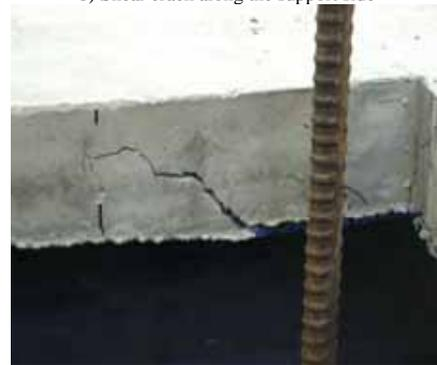
d) Shear crack in the opening
