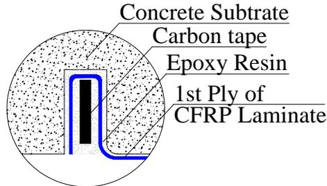
c) Detail of the anchoring device
