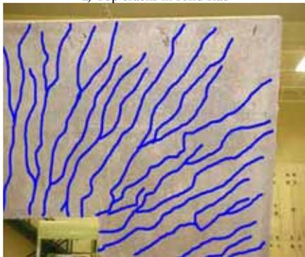
c) Typical crack pattern on bottom of the slab
