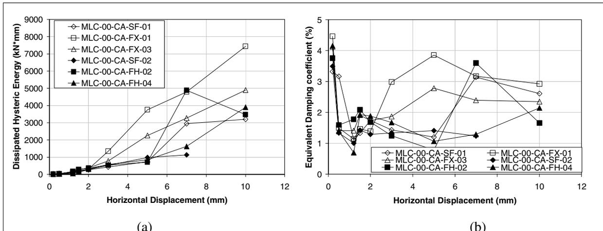
Figure 12. (a) Dissipated hysteretic energy, (b) equivalent damp coefficient for the first cycle.
