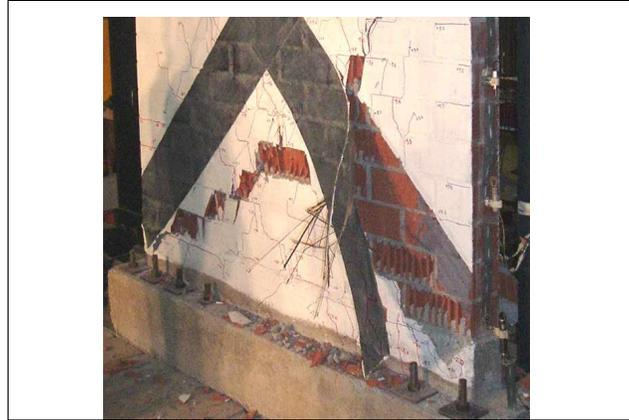
Figure 9. Failure mode of the DRM walls. The bottom bricks were previously damaged.
