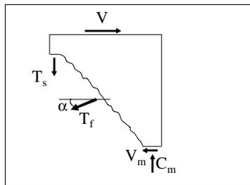
Figure 13. Force system in a cracked wall.
