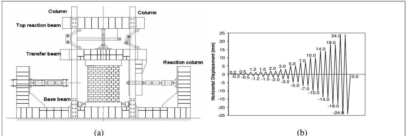
Figure 4. (a) Reaction frame. (b) Horizontal displacement program for the cyclic shear tests.
