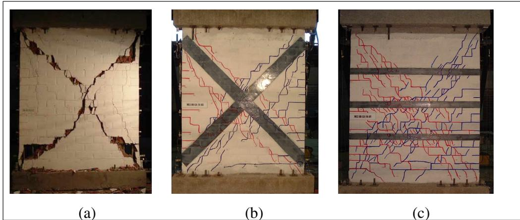
Figure 11. Crack pattern: (a) URM wall, (b) DRM wall, (c) HRM wall.
