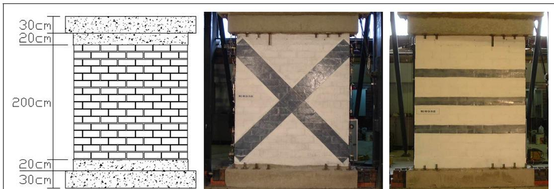
Figure 2. Configurations of the exterior reinforcement.
