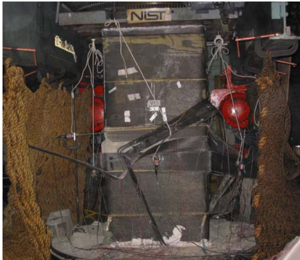
Figure 5 – Failure of Strengthened Square Specimen 36in x 36in at NIST
