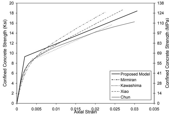
**Figure 8** Comparison of Proposed FRP-Confined Concrete with Reviewed Models
