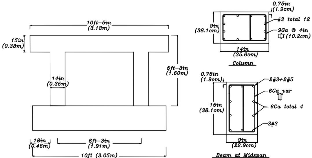
**Figure 1** Test Specimen Dimensions
