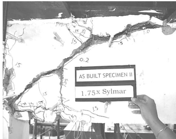
**Figure 5** Final Stage of As-Built Cap Beam
