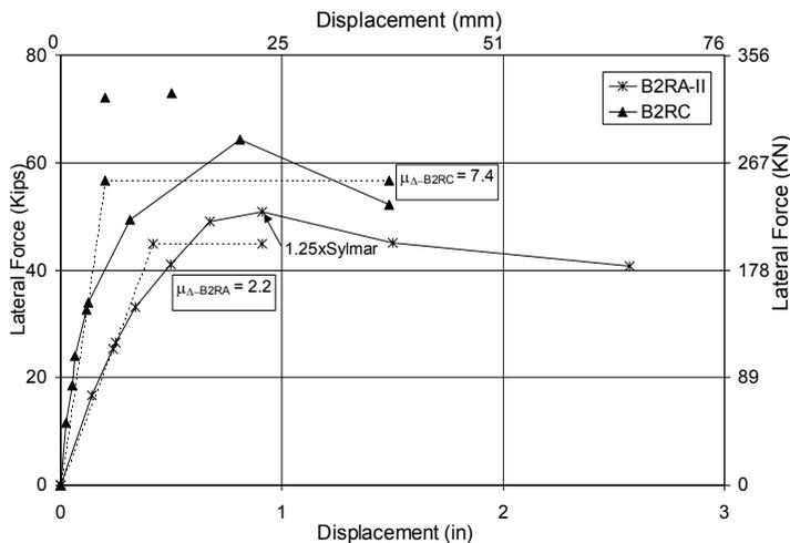
**Figure 7** Comparisons of Force-Displacement Hysteresis Envelopes
