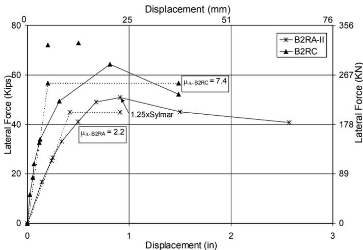
**Figure 7** Comparisons of Force-Displacement Hysteresis Envelopes
