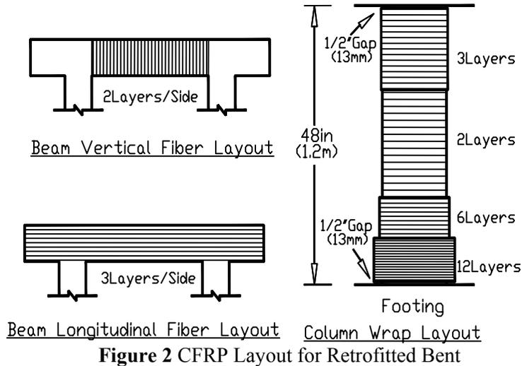
**Figure 2** CFRP Layout for Retrofitted Bent
