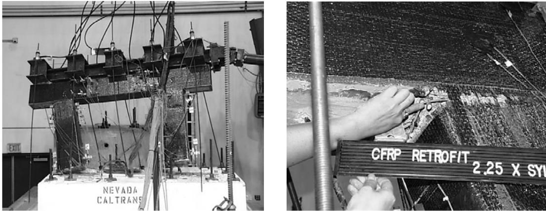
**Figure 6** Final Stage of CFRP Retrofitted Bent
