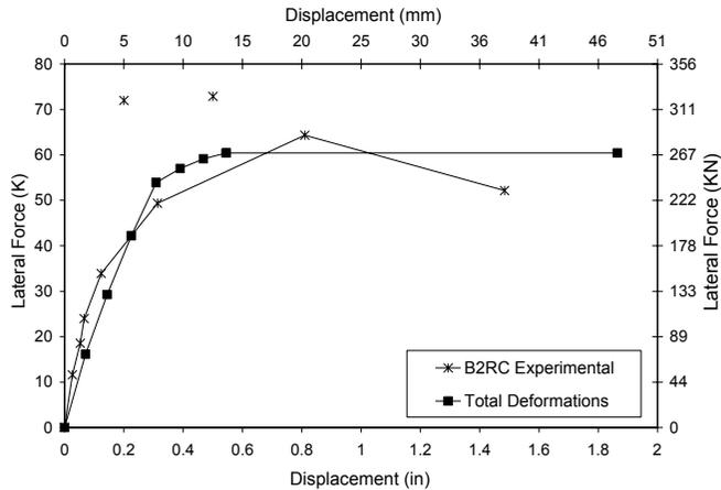
**Figure 9** Force-Displacement Curve of the CFRP Retrofitted Bent
